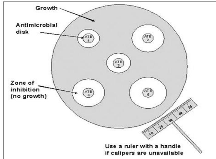
**Figure 5.1 The antimicrobial susceptibility disk diffusion test: approximate disk placement and measurement of inhibition zone diameters.**
