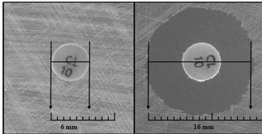
**Figure 5.2 Images showing proper measurement of zone diameter**
