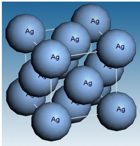
**Figure 4.13 Structure of Ag (Face Centered Cubic Structure)**
