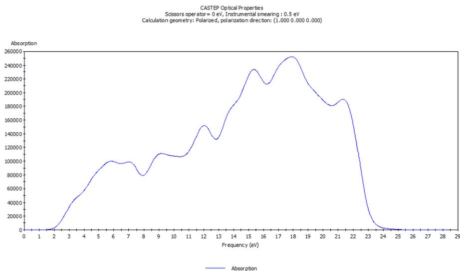
**Figure 4.17 Absorption Spectrum of Ag (LDA)**
