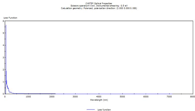
**Figure 4.12 Loss Function of Fe (LDA)**
