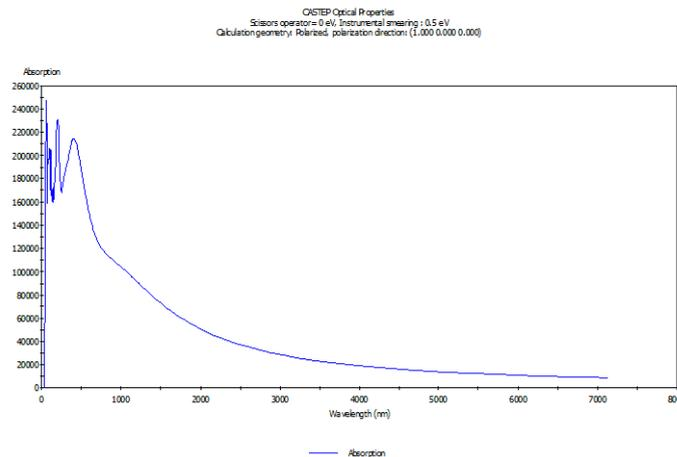
**Figure 4.7 Absorption spectrum of Fe (LDA)**
