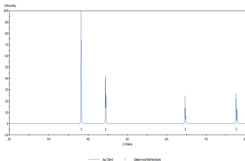
**Figure 4.14 Simulated XRD pattern of Ag Face Centered structure**
