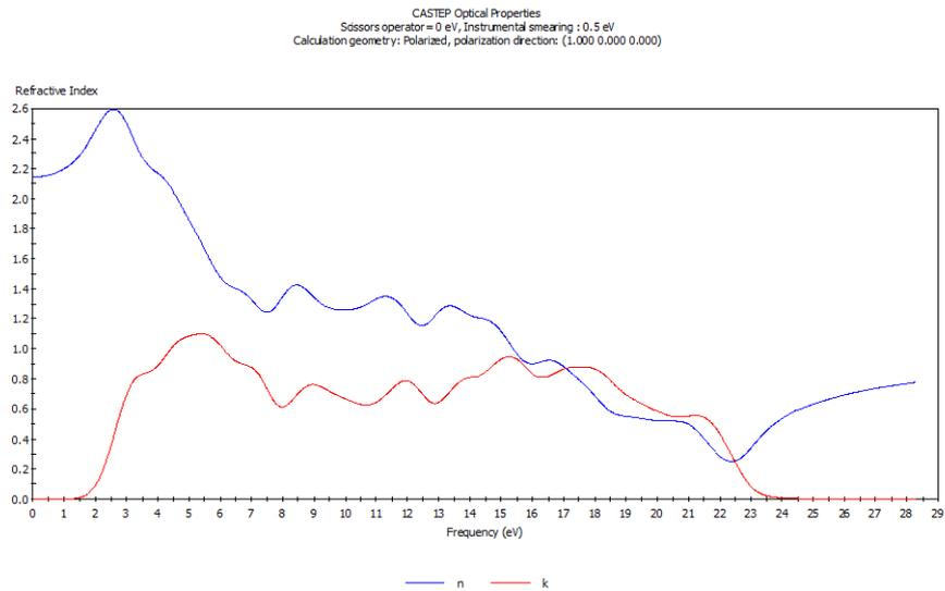
**Figure 4.19 Refractive index and Extinction Coefficient of Ag (LDA)**
