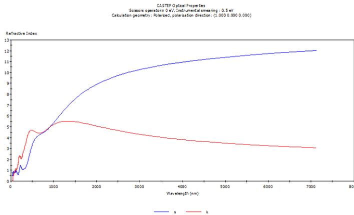
**Figure4.9 Refractive index and Extinction coefficient of Fe (LDA)**
