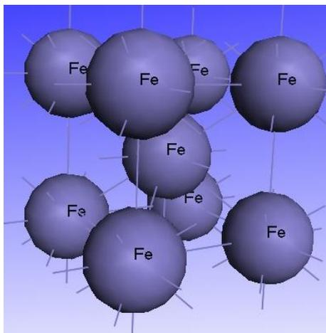
**Figure 4.1 Structure of Fe (Body Centered Cubic Structure)**
