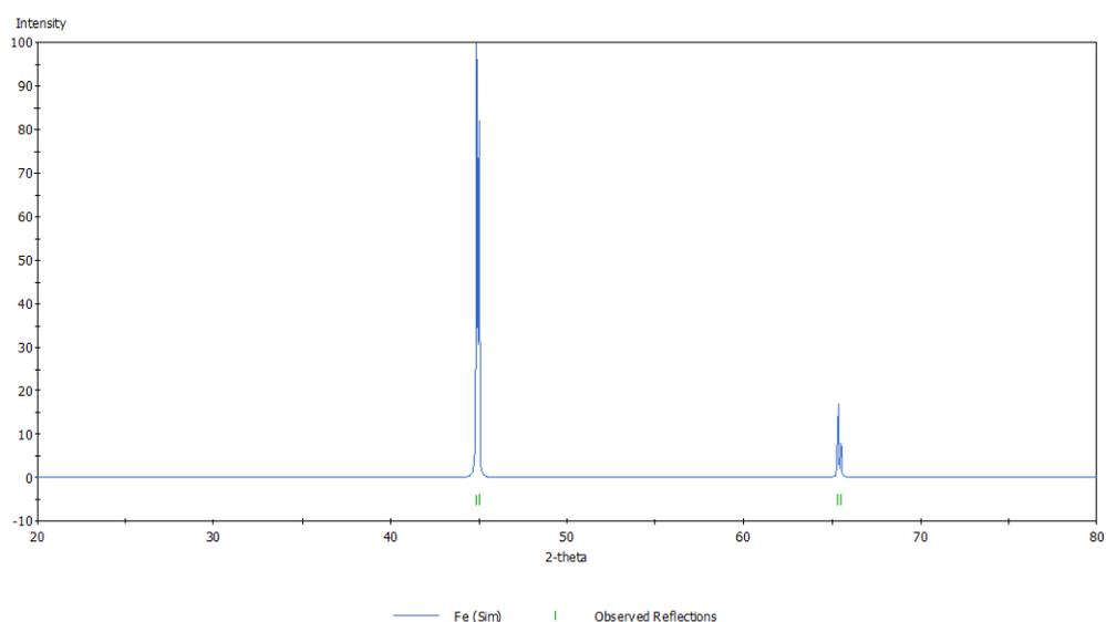
**Figure 4.2 Simulated XRD pattern of FeBody Centered structure**
