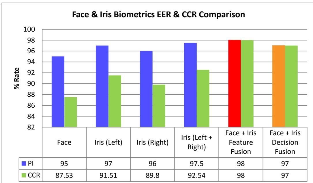
**Fig. 6.6. Performance Index (PI) & CCR comparison for Final Hybrid Multimodal System with Face & Iris Recognition Systems (For Iris Recognition Maximum Performance is considered for Comparison)**
