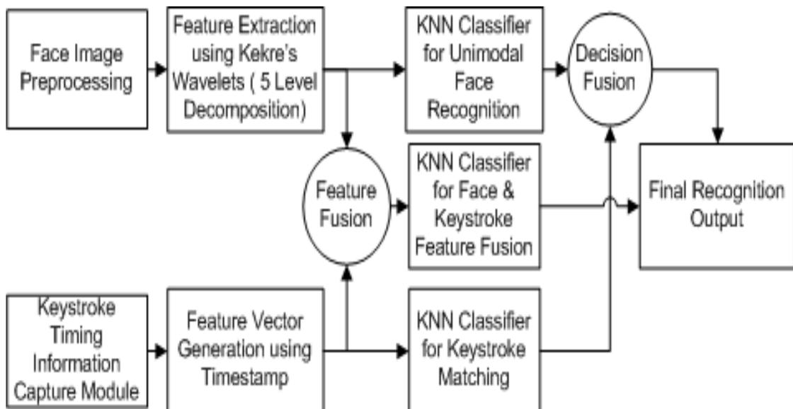
**Fig. 6.7. Architecture of Multimodal Biometric System using Face & Keystroke Dynamics Fusion**
