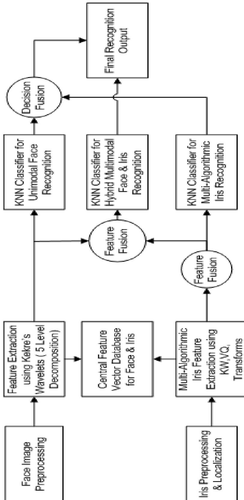
**Fig. 6.2. Multimodal Biometric System using Face & Iris Fusion [275]**
