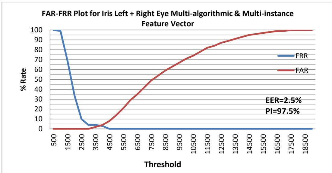
**Fig. 6.4. FAR-FRR Plot for Multi-algorithmic & Multi-instance fusion of Iris Recognition with Left + Right Eye Testing**
