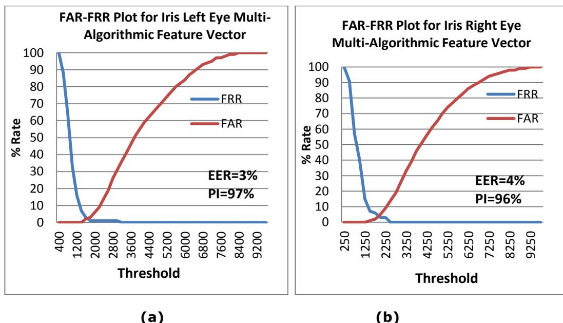
**Fig. 6.3. FAR-FRR Plot for Multi-algorithmic Iris Recognition (a) Only Left Eye Testing (b) Only Right Eye Testing**
