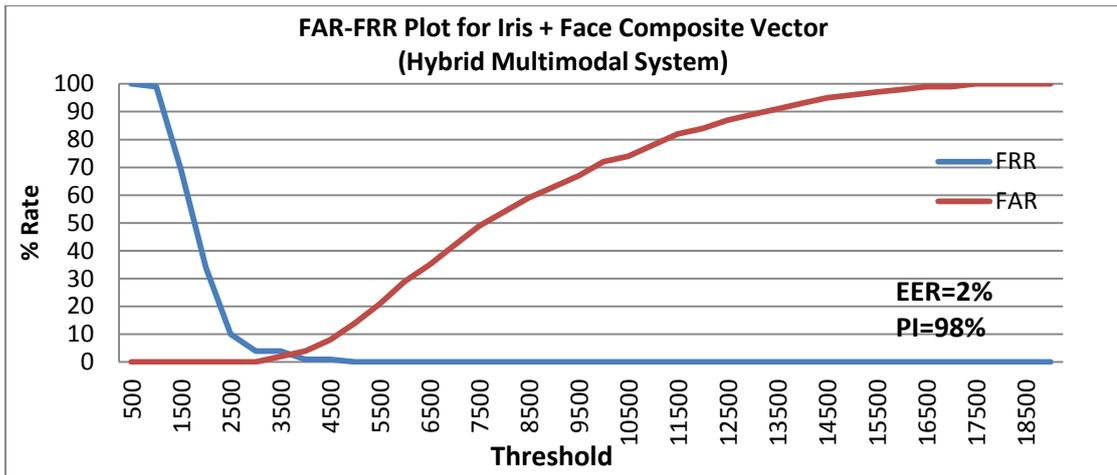
**Fig. 6.5. FAR-FRR Plot for Final Hybrid Multimodal System with Fusion of Face & Iris**
