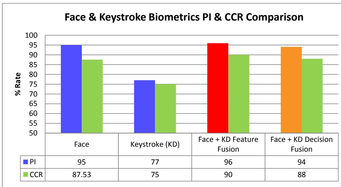
**Fig. 6.9. PI & CCR comparison for Multimodal System with Face & Keystroke Dynamics**
