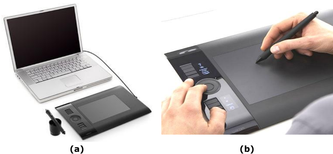
Fig. 5.1. Digitizer Tablet for Online Signature Scan (a) Wacom Intuos4 Digitizer Connected to PC (b) Scanning of Dynamic Signature
