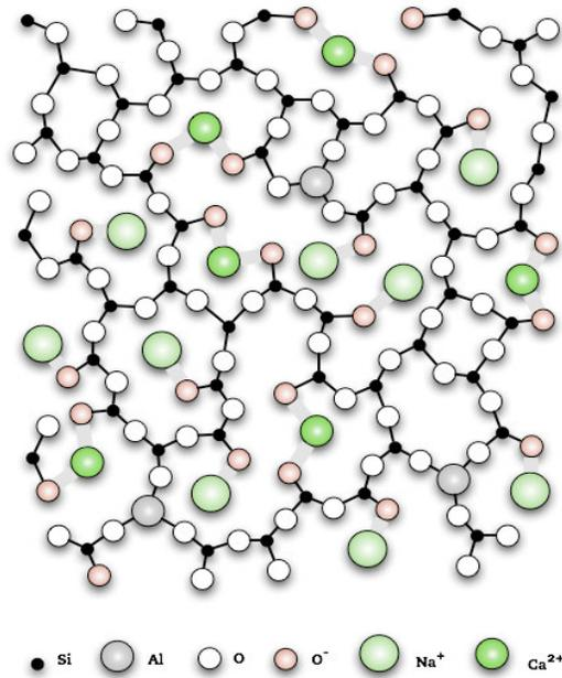
**Fig. 1.2** Structure of a general glass with modifier oxides
