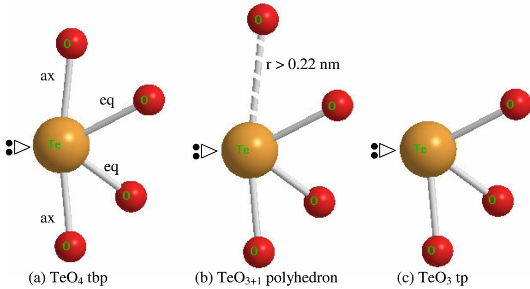
**Fig. 1.4** Illustration of the coordination states of tellurium atom (a)  $\text{TeO}_4$  trigonal bipyramid (tbp), (b)  $\text{TeO}_{3+1}$  polyhedron and (c)  $\text{TeO}_3$  trigonal pyramid (tp)
