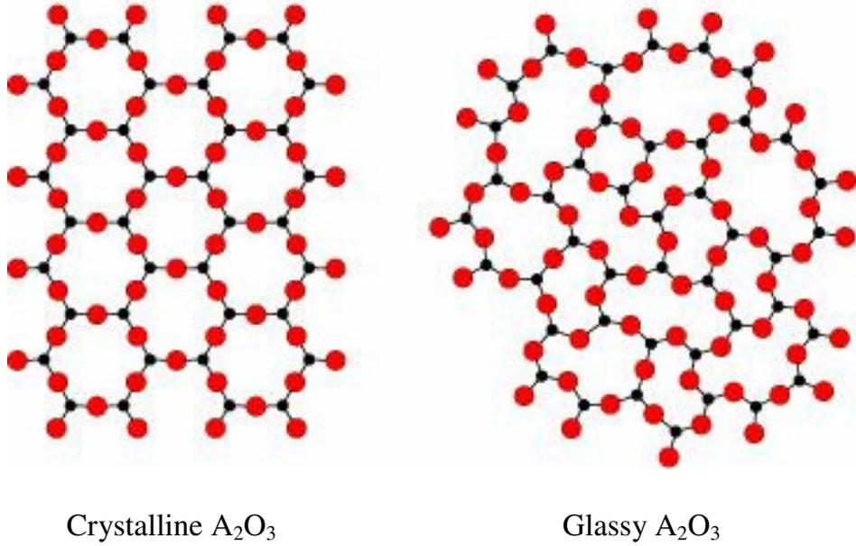
**Fig. 1.1** Two dimensional schematic of crystalline and non-crystalline (glass) materials.
