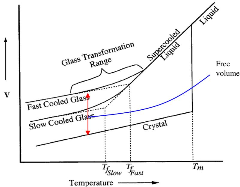
**Fig. 1.3** Schematic illustration of the change in volume with temperature as super cooled liquid is cooled through the glass transition temperature  $T_g$ .
