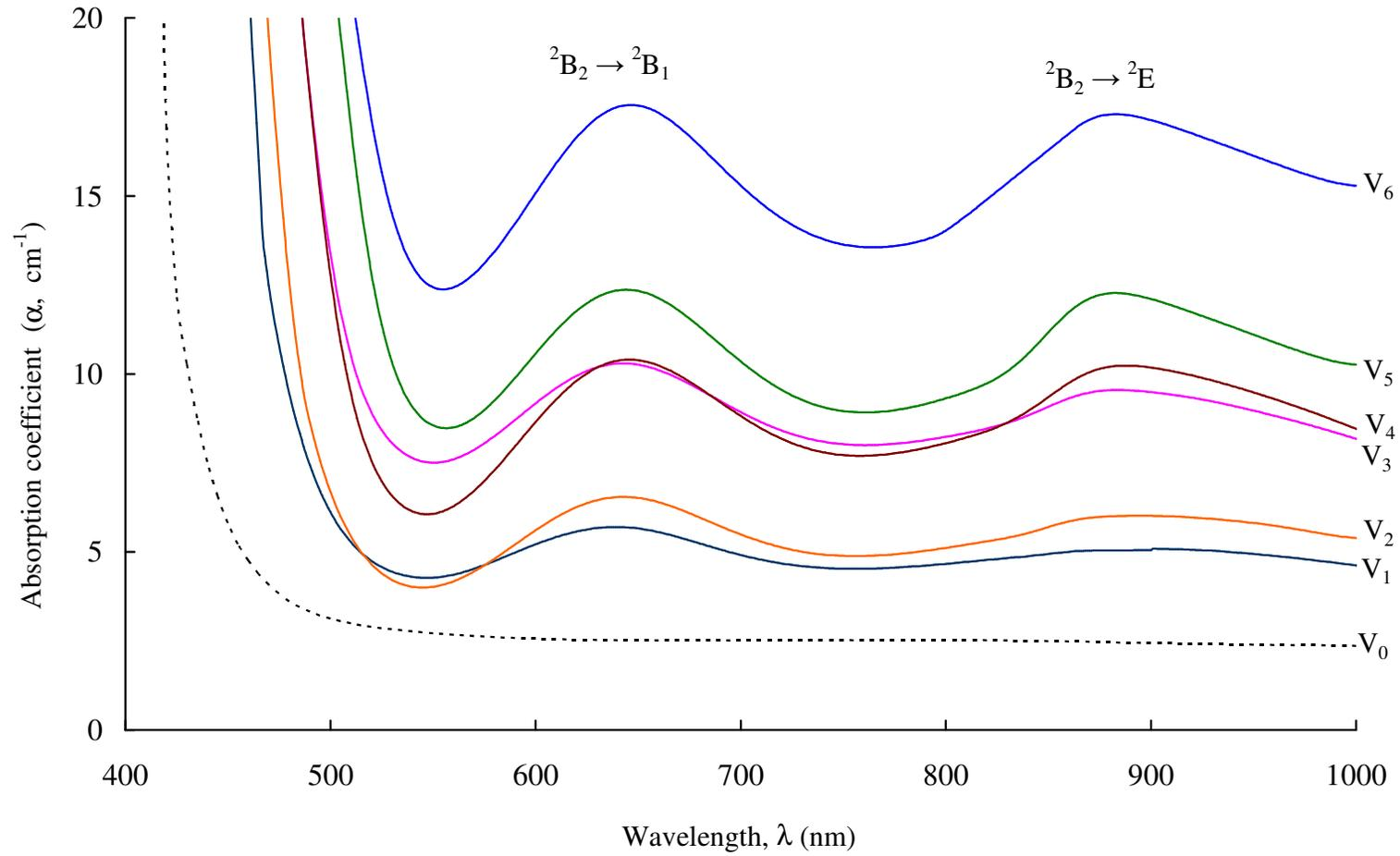
**Fig. 3.4** Optical absorption spectra of ZnF<sub>2</sub>-As<sub>2</sub>O<sub>3</sub>-TeO<sub>2</sub>: V<sub>2</sub>O<sub>5</sub> glasses.
