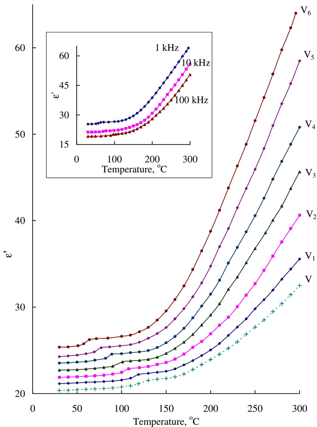
**Fig. 3.10A** A comparison plot of variation of dielectric constant with temperature at 1 kHz for  $\text{ZnF}_2\text{-As}_2\text{O}_3\text{-TeO}_2\text{:V}_2\text{O}_5$  glasses. Inset shows variation of dielectric constant with temperature at different frequencies for glass containing 0.6 mol% of  $\text{V}_2\text{O}_5$ .
