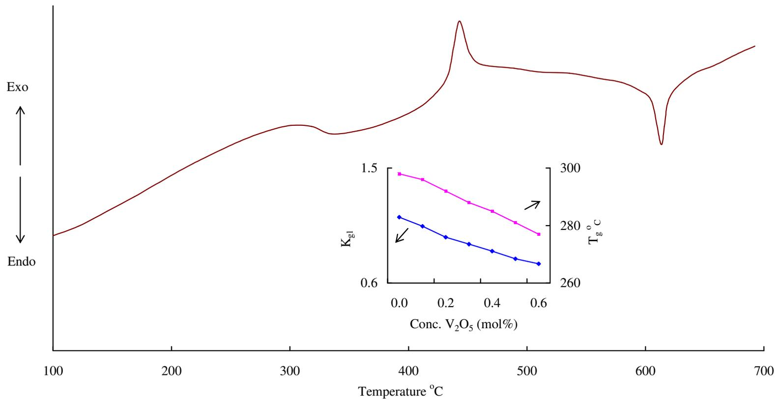
**Fig. 3.4** DSC trace of ZnF<sub>2</sub>-As<sub>2</sub>O<sub>3</sub>-TeO<sub>2</sub> glass doped with 0.3 mol% of V<sub>2</sub>O<sub>5</sub>. Inset shows the variation of T<sub>g</sub> and K<sub>gl</sub> with the concentration of V<sub>2</sub>O<sub>5</sub>.
