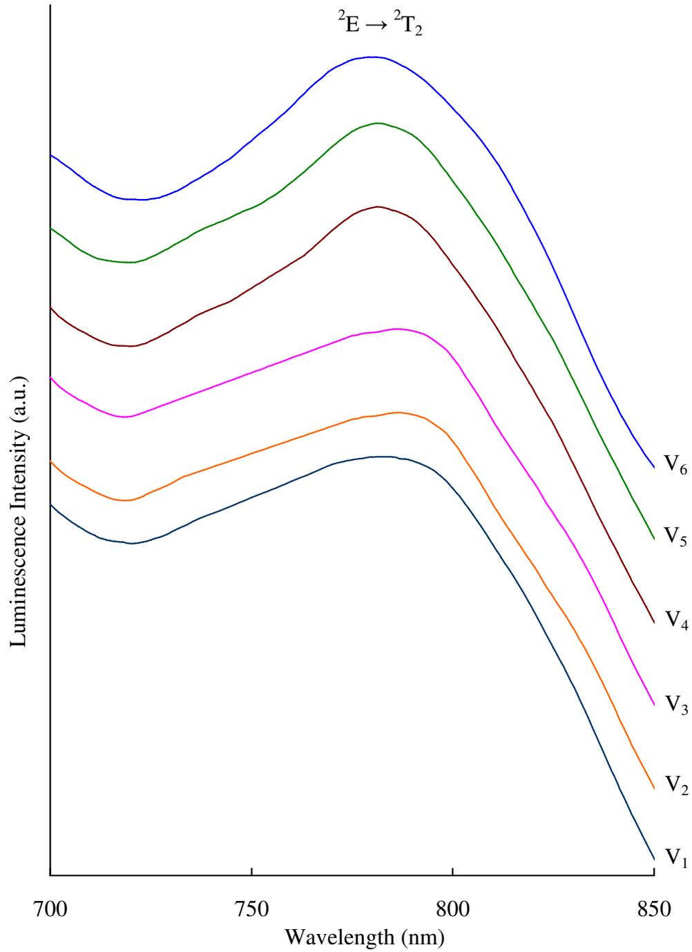
**Fig. 3.6** Photoluminescence of  $\text{ZnF}_2\text{-As}_2\text{O}_3\text{-TeO}_2\text{:V}_2\text{O}_5$  glasses recorded at room temperature ( $\lambda_{\text{exc}}=640\text{nm}$ ).
