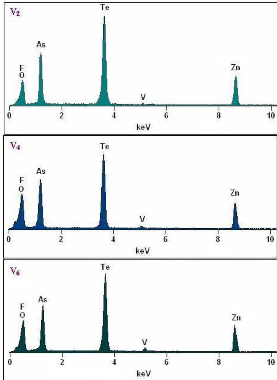
**Fig. 3.3** EDS pictures of some of the  $\text{ZnF}_2\text{-As}_2\text{O}_3\text{-TeO}_2\text{:V}_2\text{O}_5$  glasses.
