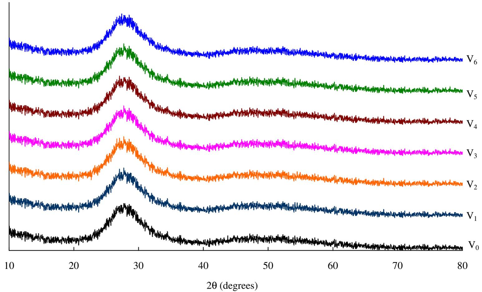
**Fig. 3.2** X-ray diffraction pattern of  $\text{ZnF}_2\text{-As}_2\text{O}_3\text{-TeO}_2\text{:V}_2\text{O}_5$  glasses.
