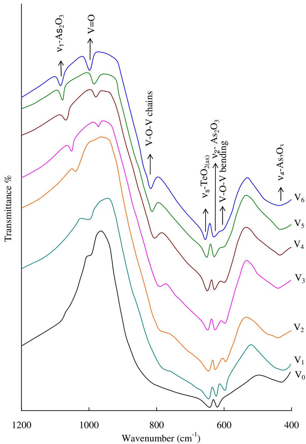
**Fig. 3.8** Infrared transmission spectra of  $\text{ZnF}_2\text{-As}_2\text{O}_3\text{-TeO}_2\text{:V}_2\text{O}_5$  glasses recorded at room temperature.
