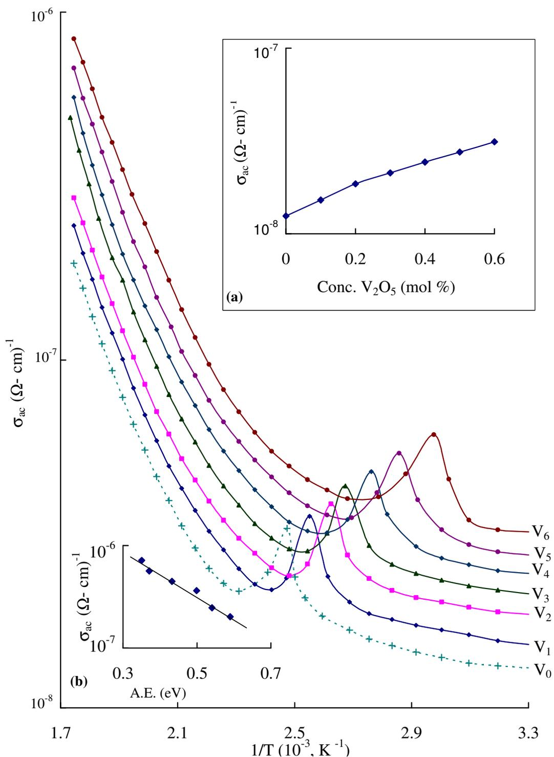
**Fig. 3.12** A comparison plot of variation of ac conductivity with  $1/T$  at 1 kHz for  $\text{ZnF}_2\text{-As}_2\text{O}_3\text{-TeO}_2\text{:V}_2\text{O}_5$  glasses. Inset (a) gives the variation of  $\sigma_{ac}$  with the concentration of  $\text{V}_2\text{O}_5$  and (b) gives the variation of  $\sigma_{ac}$  with the activation energy for conduction.
