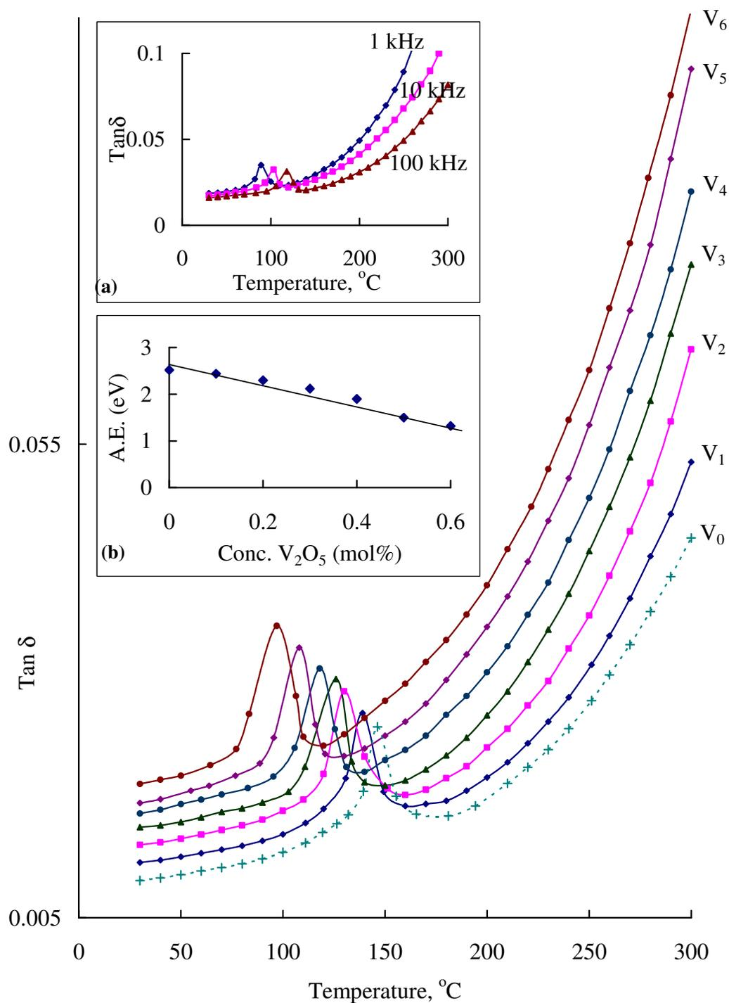
**Fig. 3.11** A comparison plot of variation of dielectric loss with temperature for  $\text{ZnF}_2\text{-As}_2\text{O}_3\text{-TeO}_2\text{:V}_2\text{O}_5$  glasses measured at 100 kHz. Inset (a) shows the variation of dielectric loss with temperature for the glass V<sub>4</sub> at different frequencies. Inset (b) shows variation of activation energy for dipoles with the concentration of  $\text{V}_2\text{O}_5$ .
