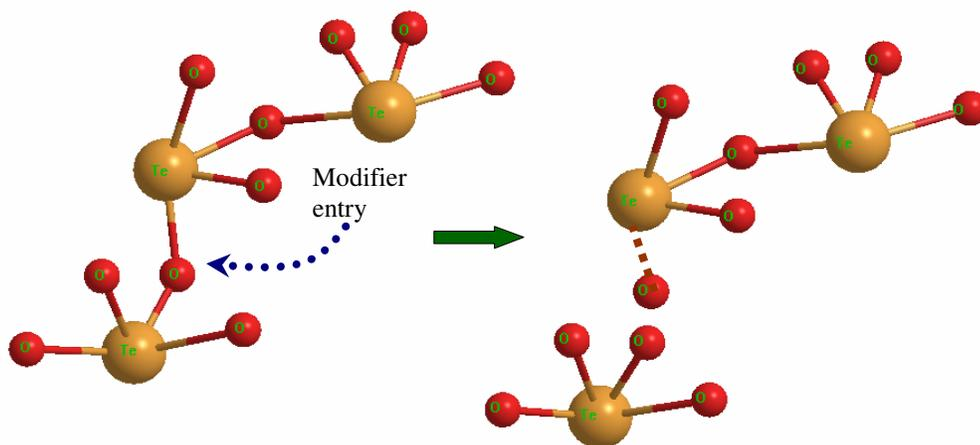
**Fig. 3.13** A mechanism for structural change in TeO<sub>2</sub> glass network from TeO<sub>4</sub> (tbp) to TeO<sub>3+1</sub> polyhedra induced by modifier.
