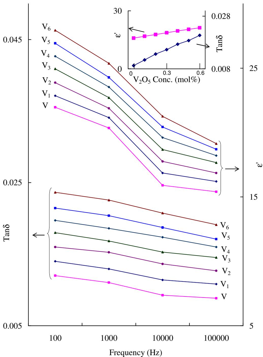
**Fig. 3.9** Variation of dielectric constant and loss with the frequency of  $\text{ZnF}_2\text{-As}_2\text{O}_3\text{-TeO}_2$  glasses containing different concentrations of  $\text{V}_2\text{O}_5$  measured at room temperature. Inset gives the variation of  $\epsilon'$  and  $\text{tan}\delta$  with the concentration of  $\text{V}_2\text{O}_5$  measured at 10 kHz.
