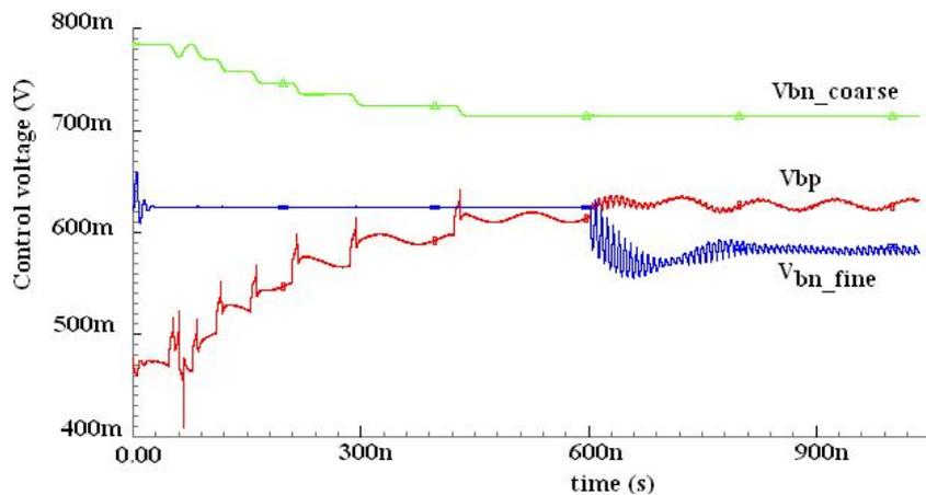
**Figure 4.11 Bias voltages satisfying the requirement of dynamic supply noise rejection**
