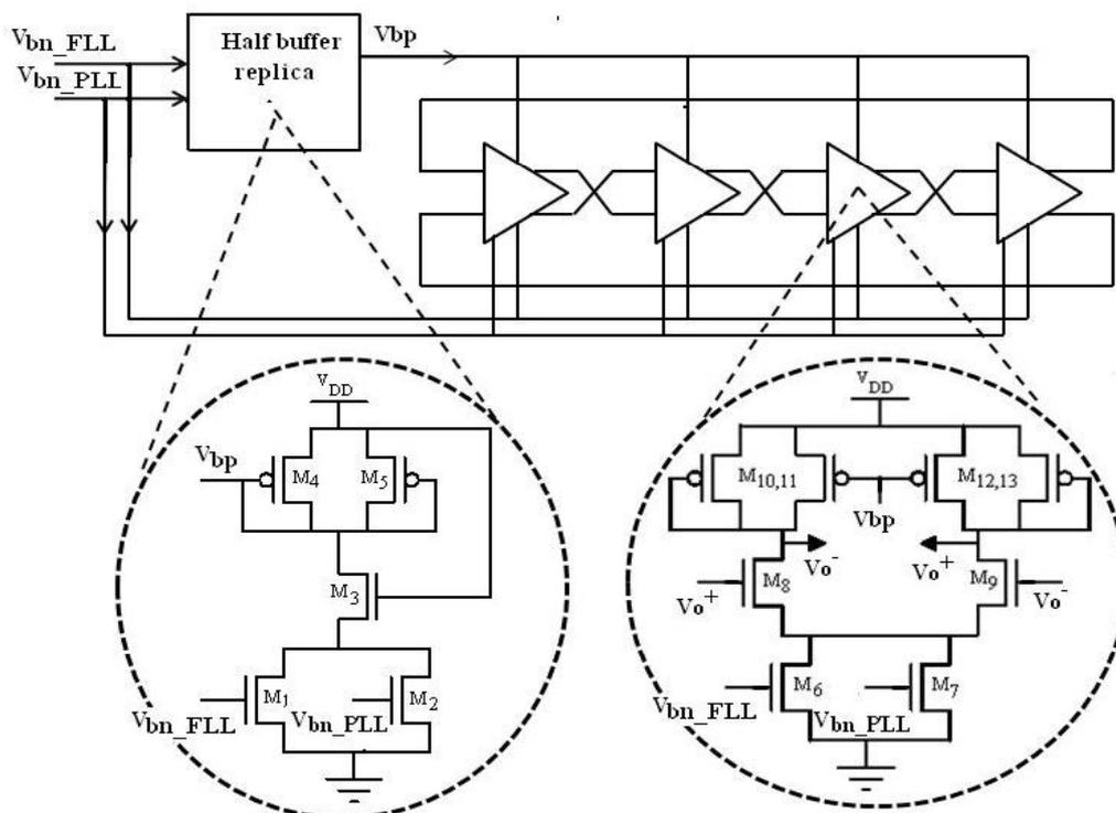
**Figure 4.2 Split Tuned VCO Showing the Modified Circuit of Delay Element and Half Buffer Replica Stage**
