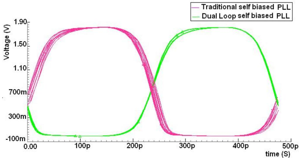
**Figure 4.7 Jitter Comparison of Traditional Self Biased PLL with Dual Loop PLL**
