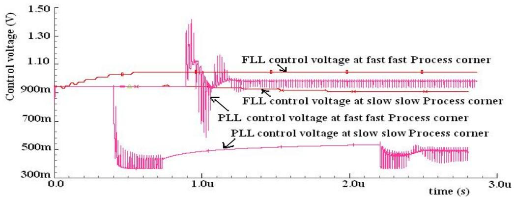
**Figure 4.8 Process Corner Simulation at 1GHz Output**
