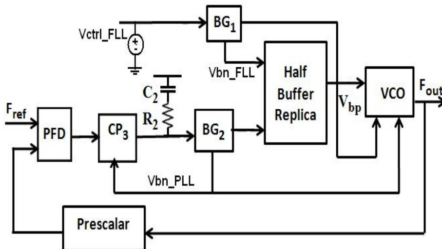
**Figure 4.4** Simulation Setting Used for Measuring Jitter for Different  $K_{VCO}$  Settings
