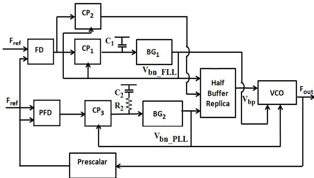
**Figure 4.1 Block Diagram of the Proposed Dual Loop System**
