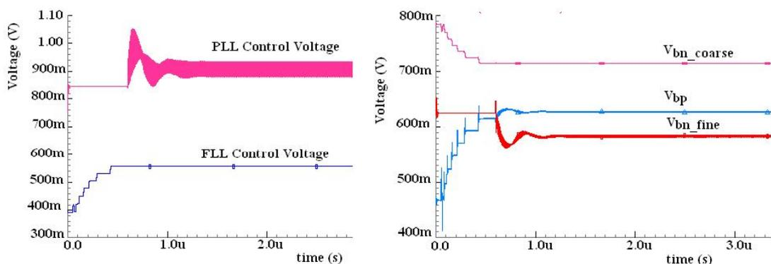
**Figure 4.6 Capture Transients of Dual Loop PLL at 2100MHz Output Frequency**
