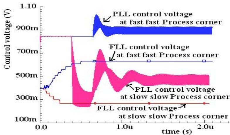
**Figure 4.9 Process Corner Simulation at 2.5 GHz Output**
