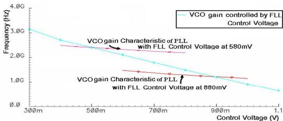
**Figure 4.5 VCO Gain Characteristic of Split Tuned VCO**
