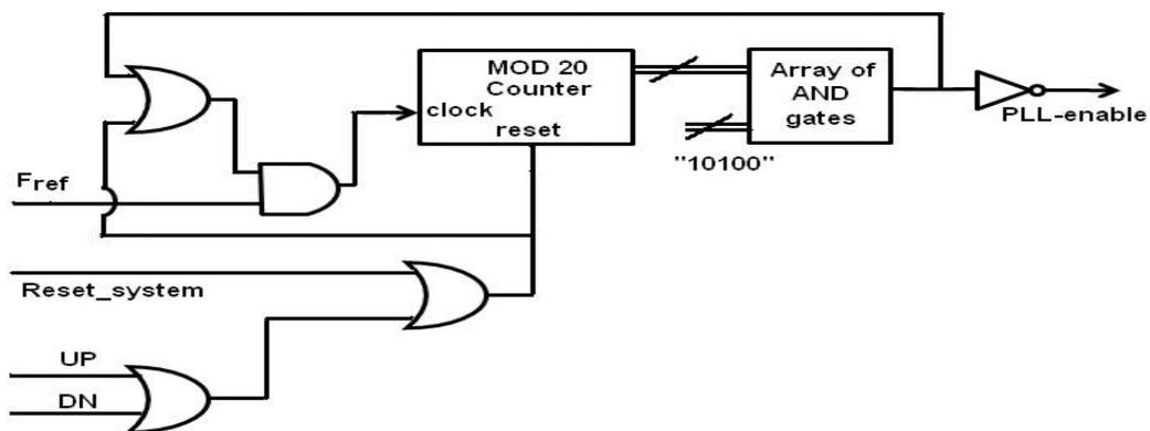
**Figure 4.3 Digital Control Circuit that Controls the Interaction Between FLL and PLL**
