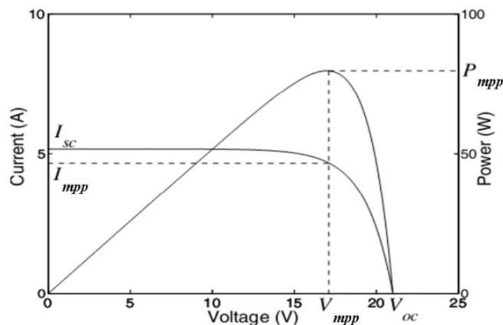
**Figure 4.1 Typical I-V Characteristics of a PV panel**
