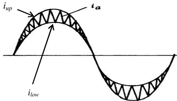
**Figure 4.7 Sinusoidal band hysteresis current controller output**
