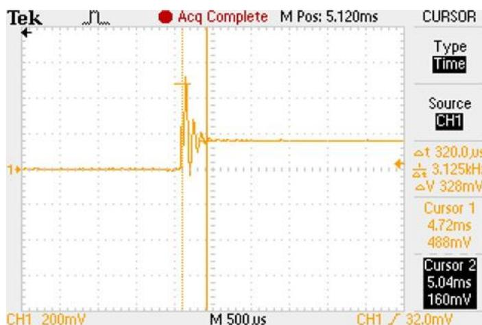
**Figure 4.5 (b) Transition of PV panel current from OC to SC**
