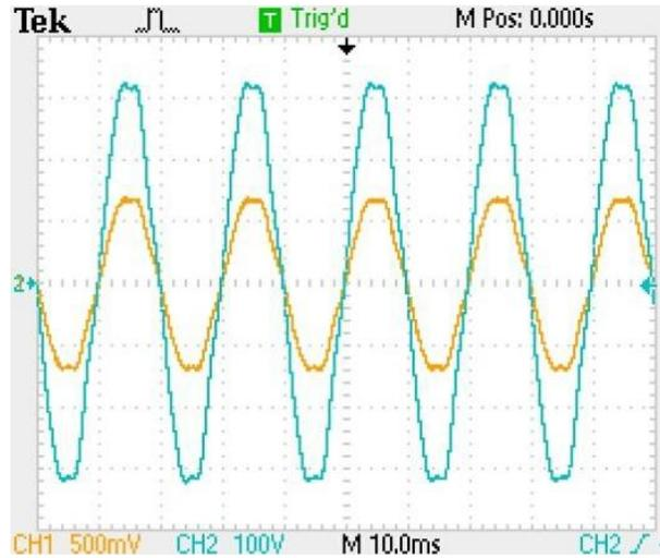
**Figure 4.12 Voltage & current at PCC for 639 W/m<sup>2</sup>**
