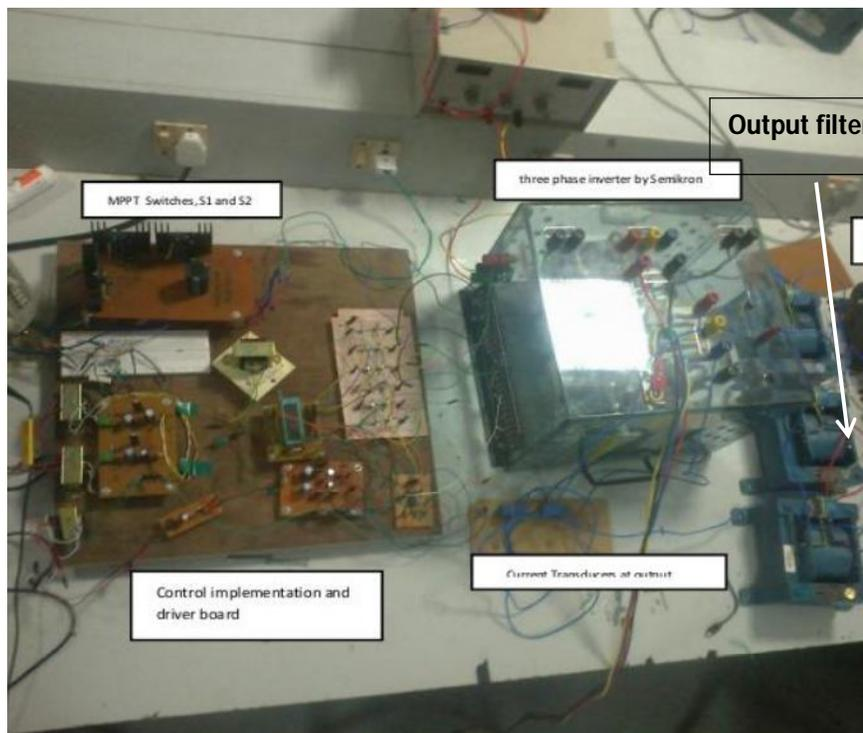
**Figure 4.9** The experimental setup of the proposed MPPT
