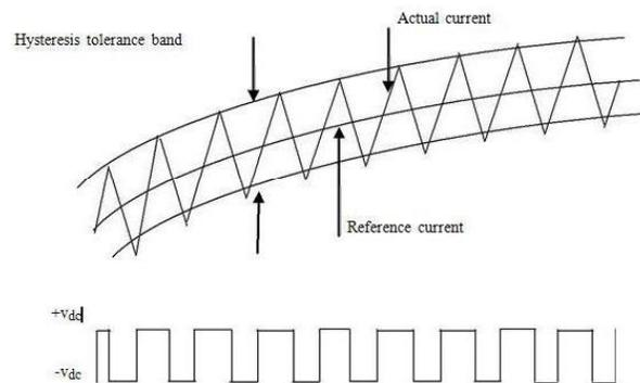
**Figure 4.8 Hysteresis current controlled inverter output voltage**
