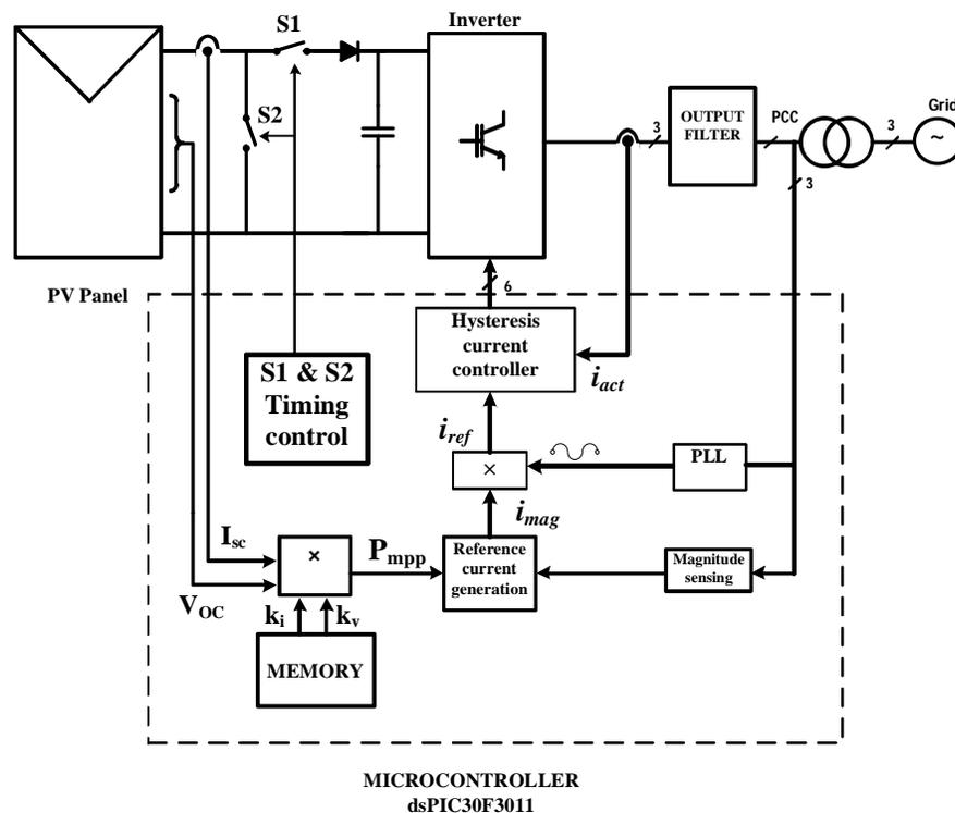
**Figure 4.6 MPPT control of Inverter through current control**
