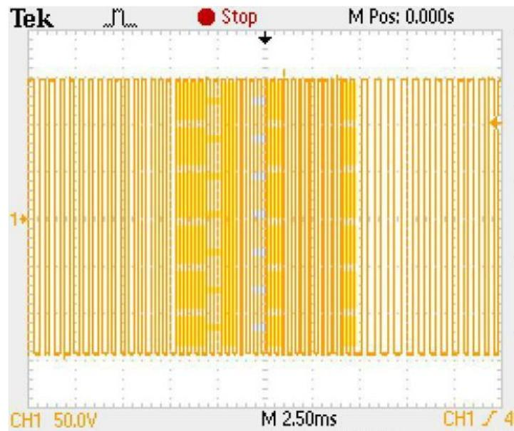
**Figure 4.10 Inverter output voltage**
