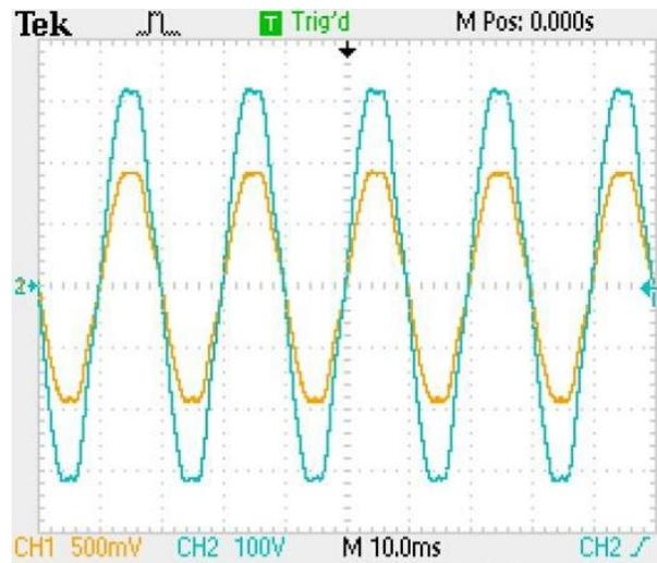
**Figure 4.13 Voltage & current at PCC for 873 W/m<sup>2</sup>**
