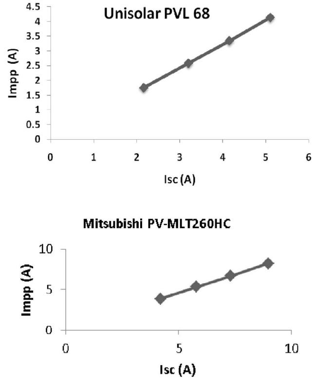
**Figure 4.2** Experimental results of  $I_{SC}$  Vs  $I_{mpp}$
