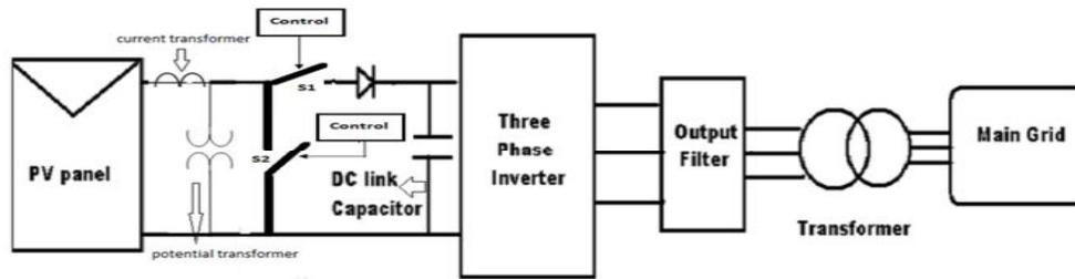
**Figure 4.4 The power circuit of the proposed MPPT system**
