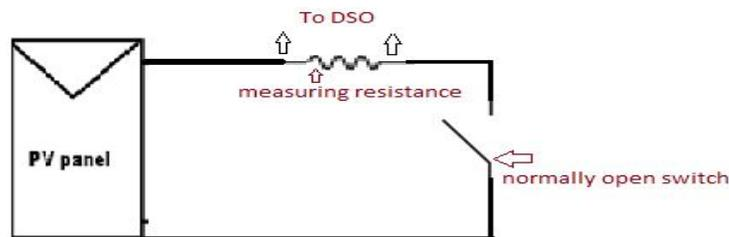
**Figure 4.5 (a) Test circuit to measure PV panel time constant**
