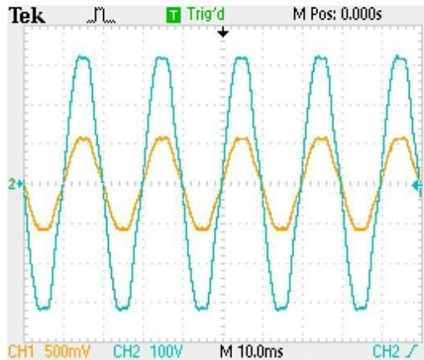
**Figure 4.14 Voltage and current at PCC under partial shading condition.**
