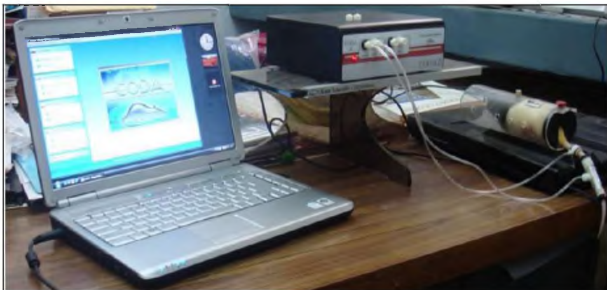
Figure 7. Non-invasive blood pressure recorder
