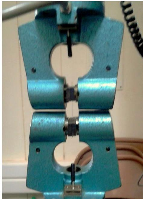
**Figure 3.1** a) Instron Tester 5500R, b) Instron measuring tensile strength at 20mm gauge length
