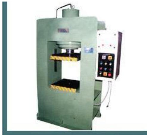
**Figure 3.9 Compression moulding machine**
