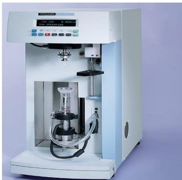
**Figure 3.7 TGA Instrument (Perkin Elmer Inc.)**
