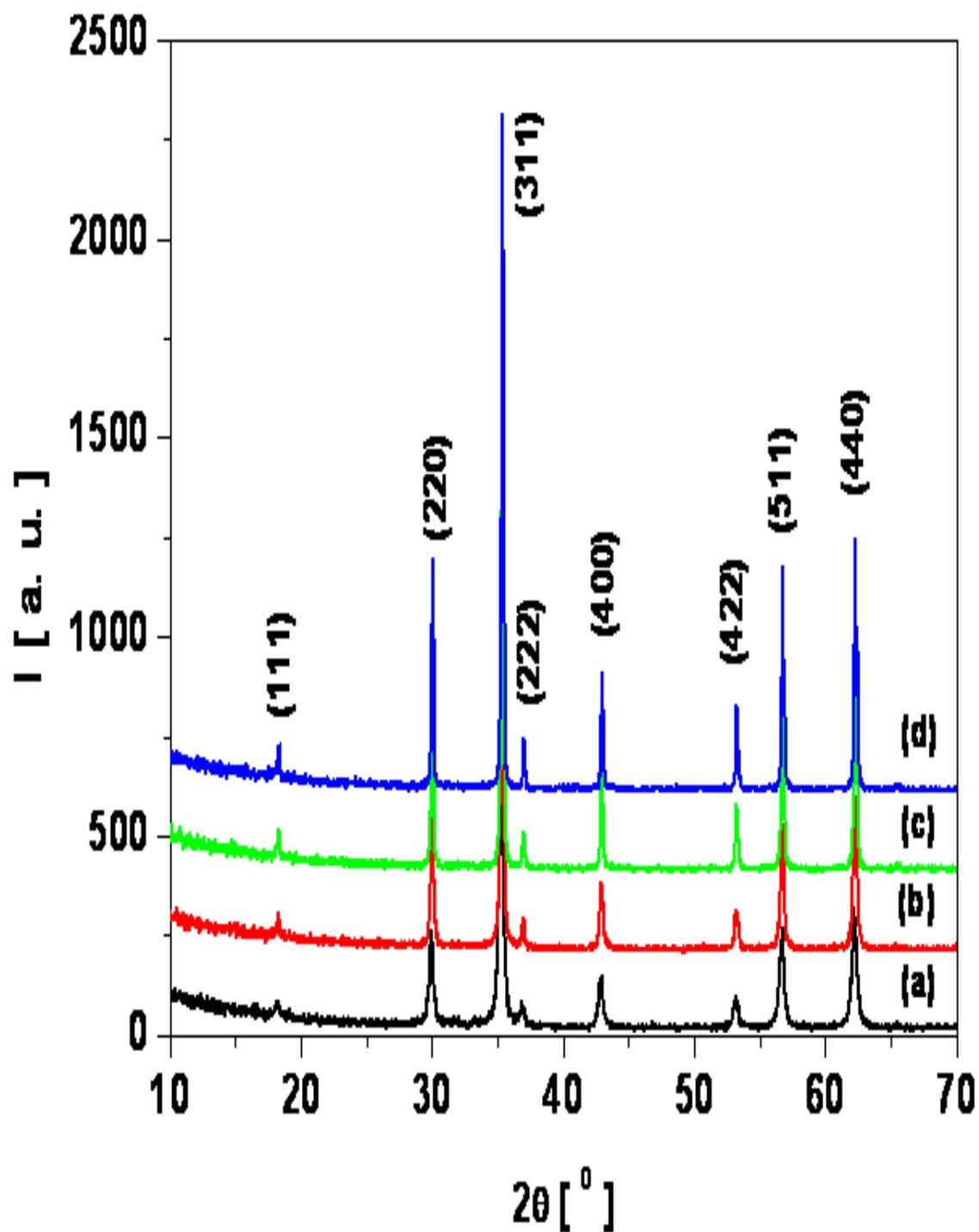
Figure 6.1: X-ray diffraction patterns of ZnFe<sub>2</sub>O<sub>4</sub> nanoparticles annealed at (a) 300°C, (b) 400°C, (c) 500°C and (d) 600°C temperatures.
