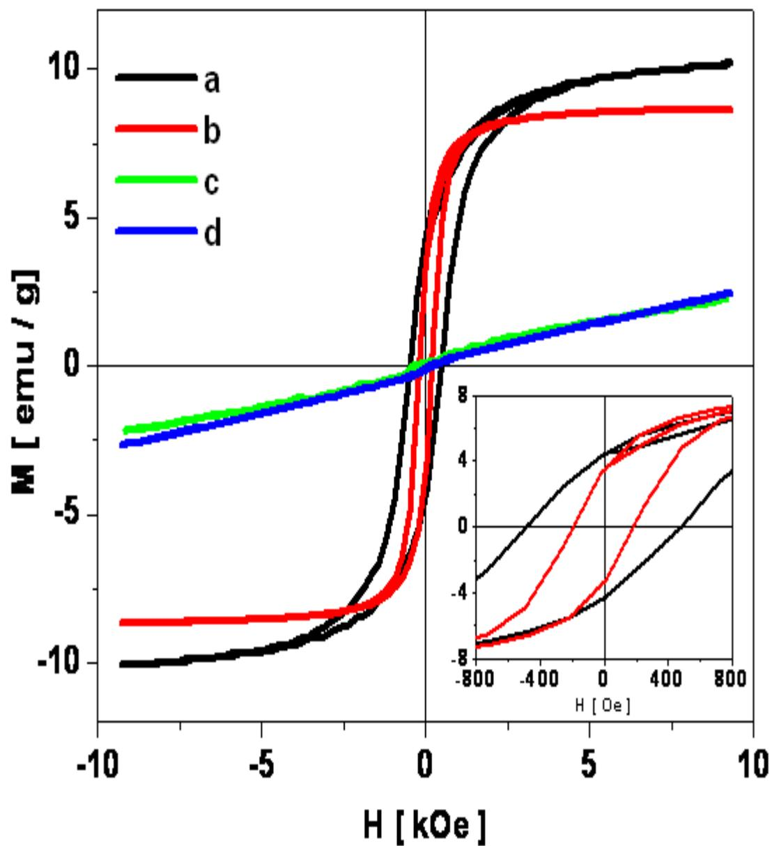
Figure 6.6: Room temperature hysteresis loops at 10kOe for ZnFe<sub>2</sub>O<sub>4</sub> nanoparticles annealed at (a) 300<sup>0</sup>C, (b) 400<sup>0</sup>C, (c) 500<sup>0</sup>C and (d) 600<sup>0</sup>C temperatures.
