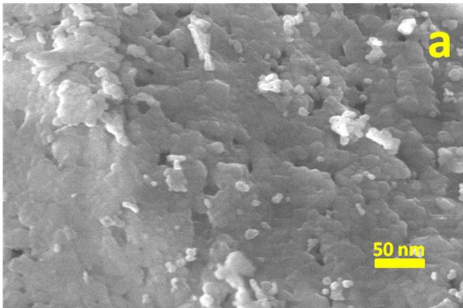
**Figure 6. 4(a): SEM micrographs of ZnFe<sub>2</sub>O<sub>4</sub> nanoparticles annealed at 300<sup>0</sup>C**
