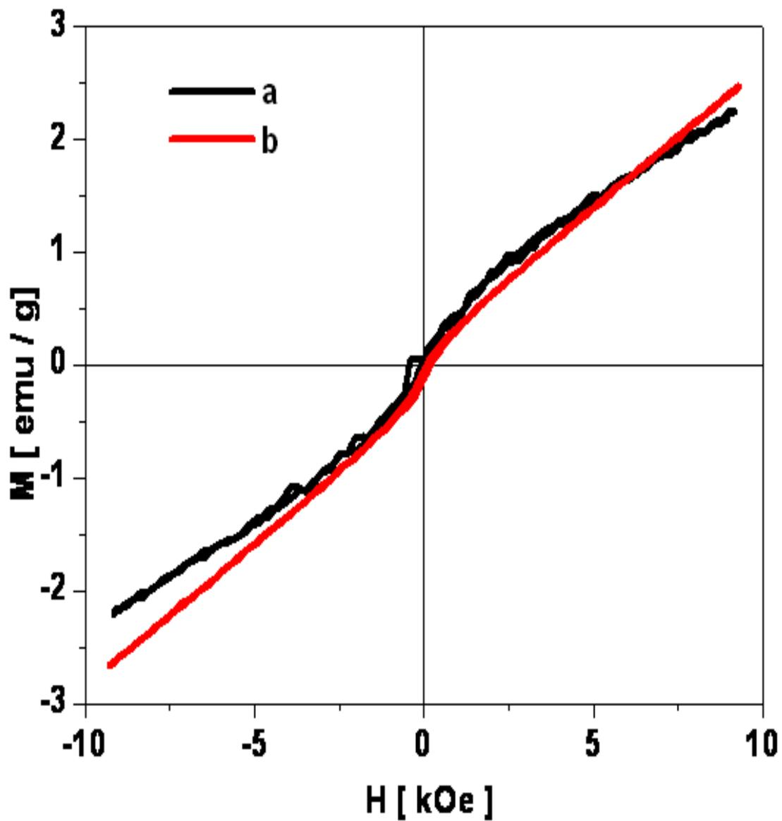
Figure 6.7: Room temperature hysteresis loops at 10kOe for  $\text{ZnFe}_2\text{O}_4$  nanoparticles annealed at (a)  $500^\circ\text{C}$  and (b)  $600^\circ\text{C}$  temperatures.
