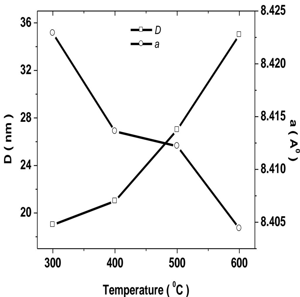
**Figure 6.3: Dependence of particle size  $D$  and lattice constant  $a$  of  $ZnFe_2O_4$  nanoparticles on the annealing temperatures.**
