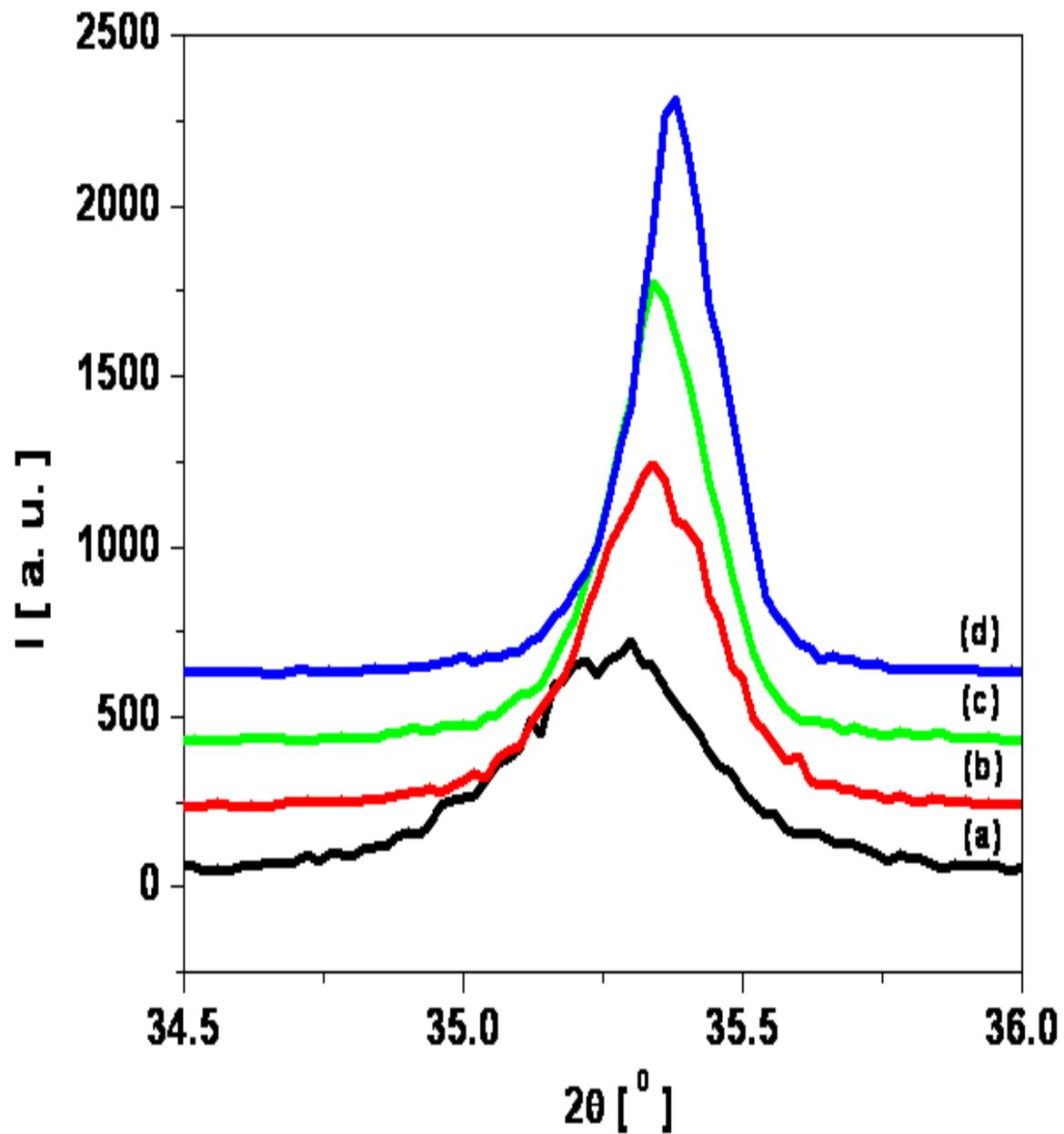
Figure 6.2: X-ray diffraction patterns of most intense (311) peak of ZnFe<sub>2</sub>O<sub>4</sub> nanoparticles annealed at (a) 300<sup>0</sup>C, (b) 400<sup>0</sup>C, (c) 500<sup>0</sup>C and (d) 600<sup>0</sup>C temperatures.
