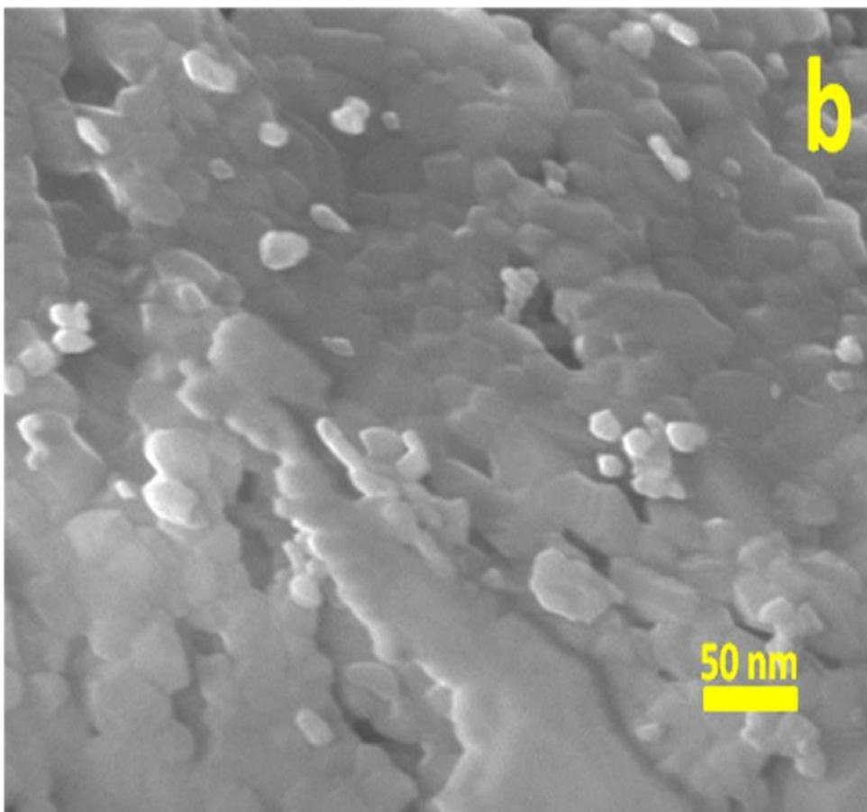
**Figure 6.4.(b): SEM micrographs of ZnFe<sub>2</sub>O<sub>4</sub> nanoparticles annealed at 500<sup>0</sup>C.**
