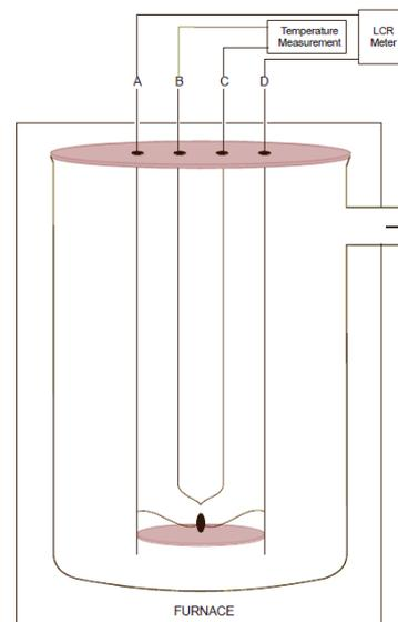
temperature could be controlled. The stray capacitance was subtracted every time to extract the correct capacitance values. The diagram of the sample holder is given in above figure.
