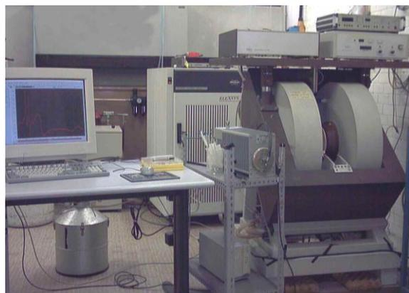
X-band frequency ( $\sim 9.43$  GHz) with a Varian Associates spectrometer (Model No. 109) and the frequency of the resonant cavity was measured by a DPPH marker at  $g = 2.0036$ .
