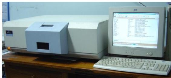
xenon flash tube, which produces an intense, short duration pulse of radiation over the spectral range of the instrument. A small festoon lamp close to the excitation source maintains an even triggering of the xenon flash tube. The Excitation and Emission monochromators can be scanned over their ranges independently, synchronously or driven to selected points in their ranges. Synchronous scanning can be either a fixed
