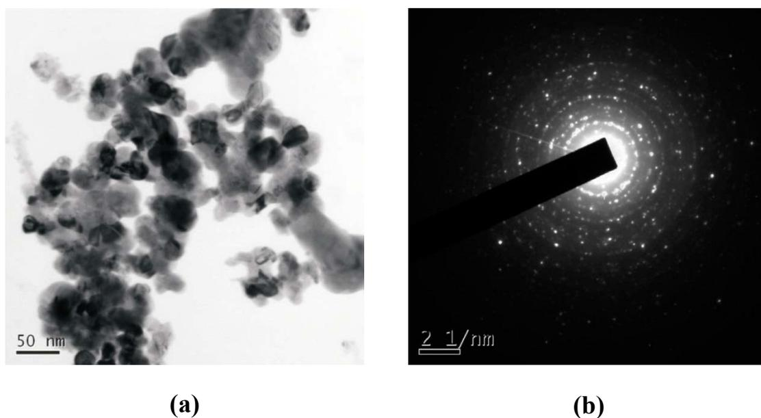
**Figure 7.2** (a) Bright field Transmission Electron Micrographs of 0.6 mole % Co ion doped BT nanocrystals and (b) Selected Area Diffraction patterns of 0.6 mole % Co ion doped BT nanopowders.
