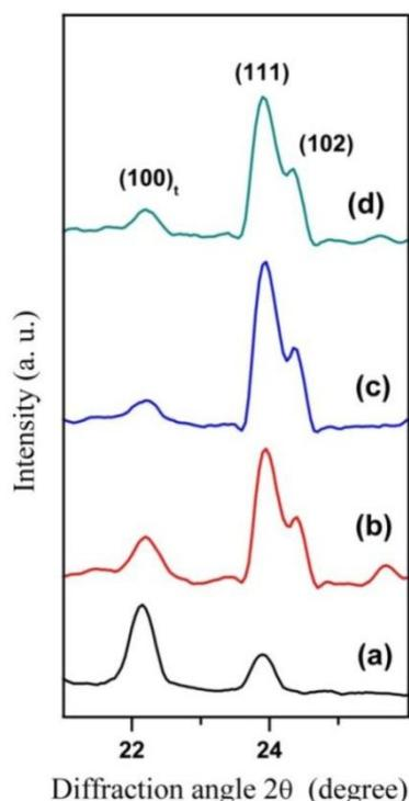
**Figure 7.3** A close-up of view of the XRD patterns in the range  $2\theta = 21^\circ - 26^\circ$  showing shifts in  $(100)_b$ ,  $(111)$  and  $(102)$  peaks of *o*-BT specimens with (b) 0.3 mole % Co ion (c) 0.6 mole % Co ion and (d) 1.6 Co mole % Co ion, comparing with (a) Undoped BT after heating at  $750^\circ\text{C}$  for 2 h in air.
