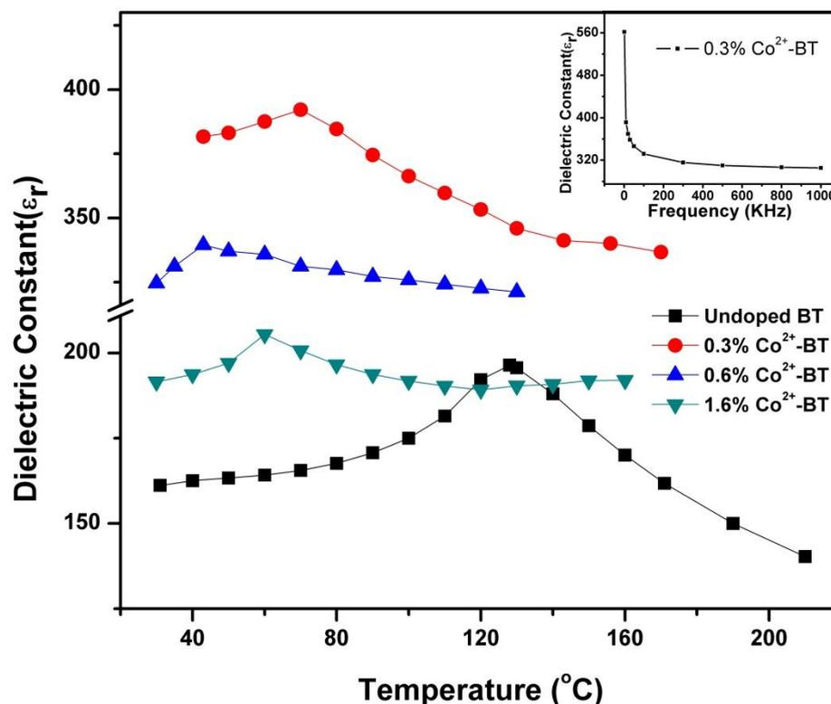
*Figure 7.4* Variation of dielectric constants with temperature obtained at a signal frequency of 10 kHz.
