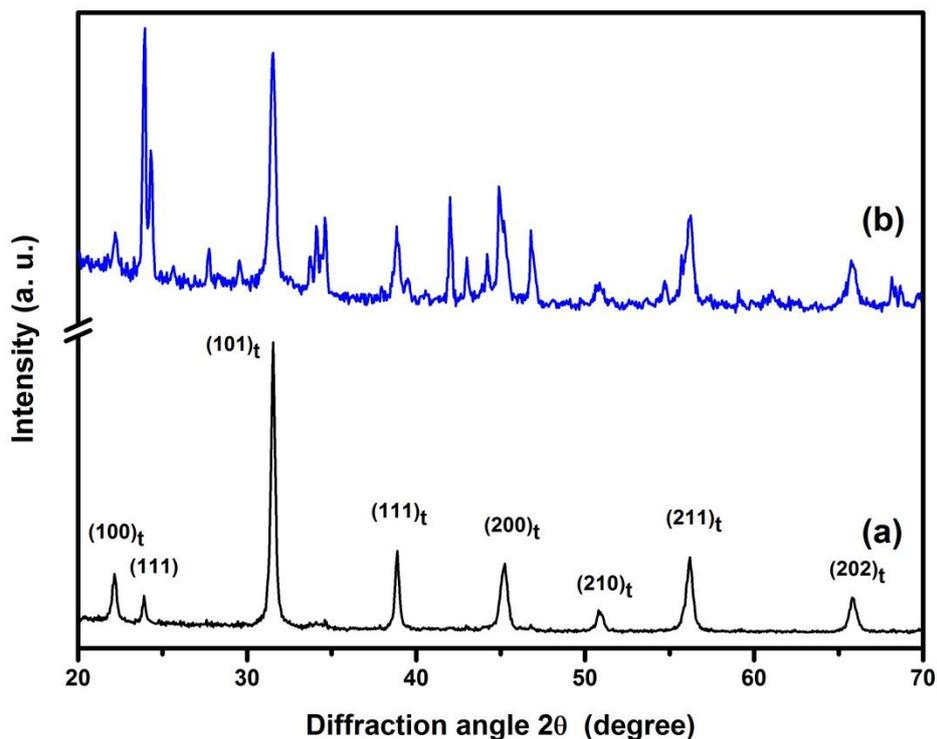
**Figure 7.1** X-ray diffraction patterns showing controlled *t*-BT to *o*-BT phase transition in a nano composite structure after doping with (b) 1.6 mole % Co ion, comparing with (a) Undoped BT.
