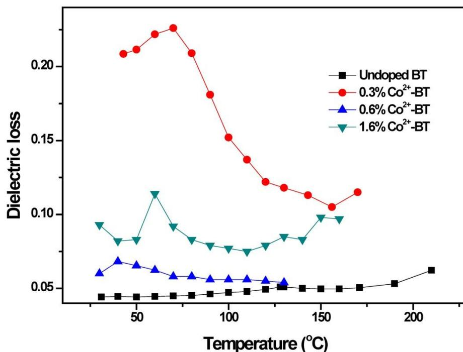
**Figure 7.5** Variation of dielectric loss with temperature obtained from the specimens at 10 kHz signal frequency.
