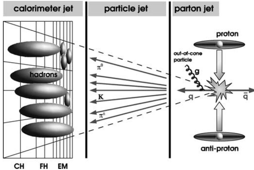
Figure 3.5: Schematic view of the jet development illustrating the idea of jet energy scale corrections, taking energy measurements on the calorimeter level to the particle or the parton level.
