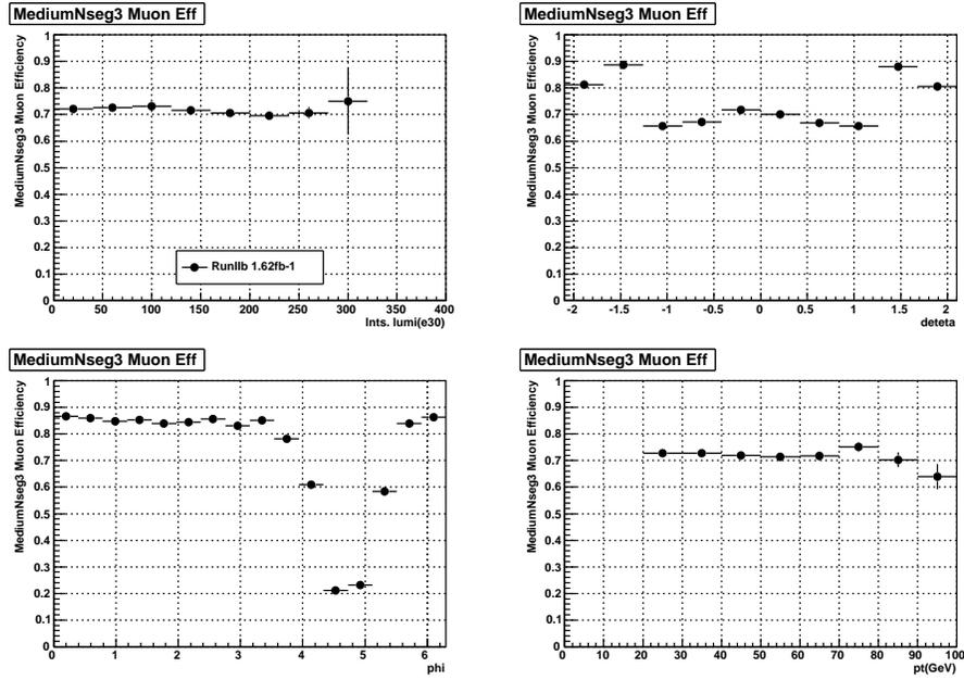
Figure 3.3: The reconstruction efficiency of muons in data for, “medium” muon quality in Run IIb data as a function of *luminosity*,  $\phi_{det}$ ,  $\phi$  and  $p_T$ .
