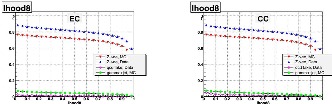
Figure 3.1: The performance of the electron likelihood for  $Z \rightarrow ee$  events in collision data and MC and for background processes of multijet and  $\gamma + jet$  production [62]. The left plot shows the efficiency for the endcaps of the calorimeter and the right plot shows the efficiency for the central part.
