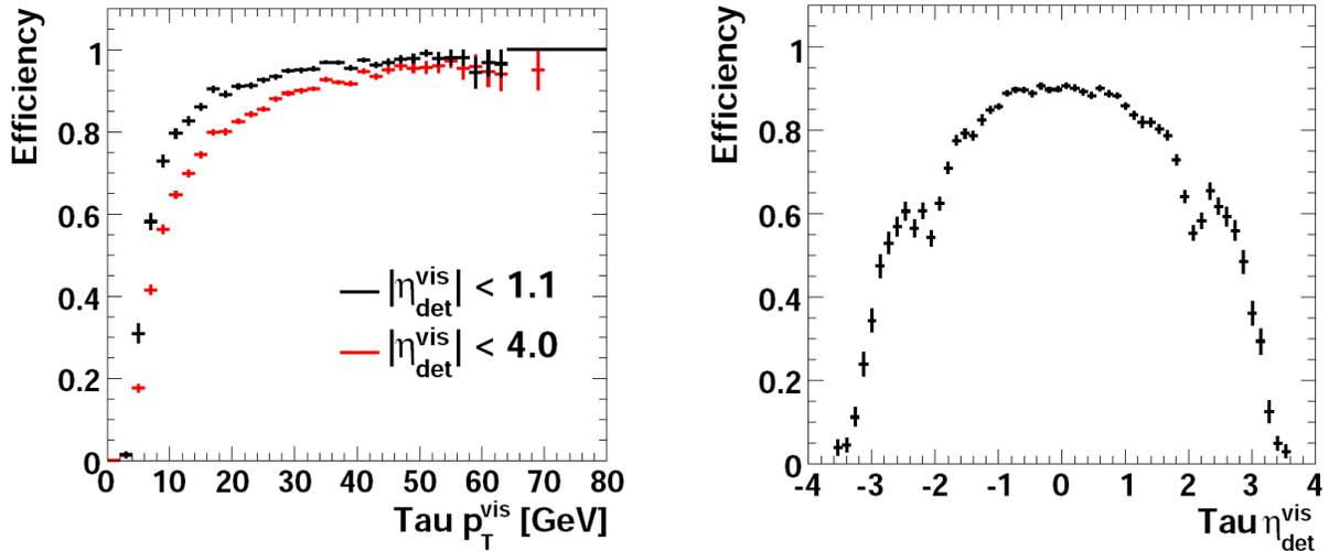
Figure 3.4: Reconstruction efficiency of hadronically decaying tau leptons as a function of  $\tau p_T^{\text{vis}}$  and  $\eta_{\text{det}}$ .
