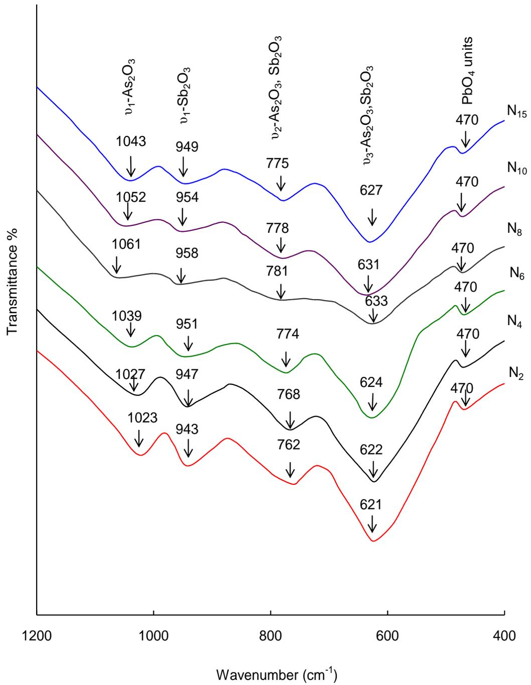
Fig. 5.7 IR spectra of PbO-Sb<sub>2</sub>O<sub>3</sub>-As<sub>2</sub>O<sub>3</sub> :NiO glass ceramics.
