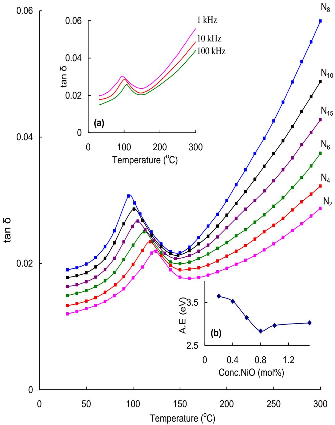
Fig. 5.10 A comparison plot of variation of dielectric loss with temperature at 10 kHz for  $\text{PbO-Sb}_2\text{O}_3\text{-As}_2\text{O}_3\text{: NiO}$  glass ceramics. Inset (a) gives the variation of dielectric loss with temperature at different frequencies of glass ceramic N<sub>10</sub> and inset (b) shows the variation of activation energy for dipoles with the concentration of nucleating agent.
