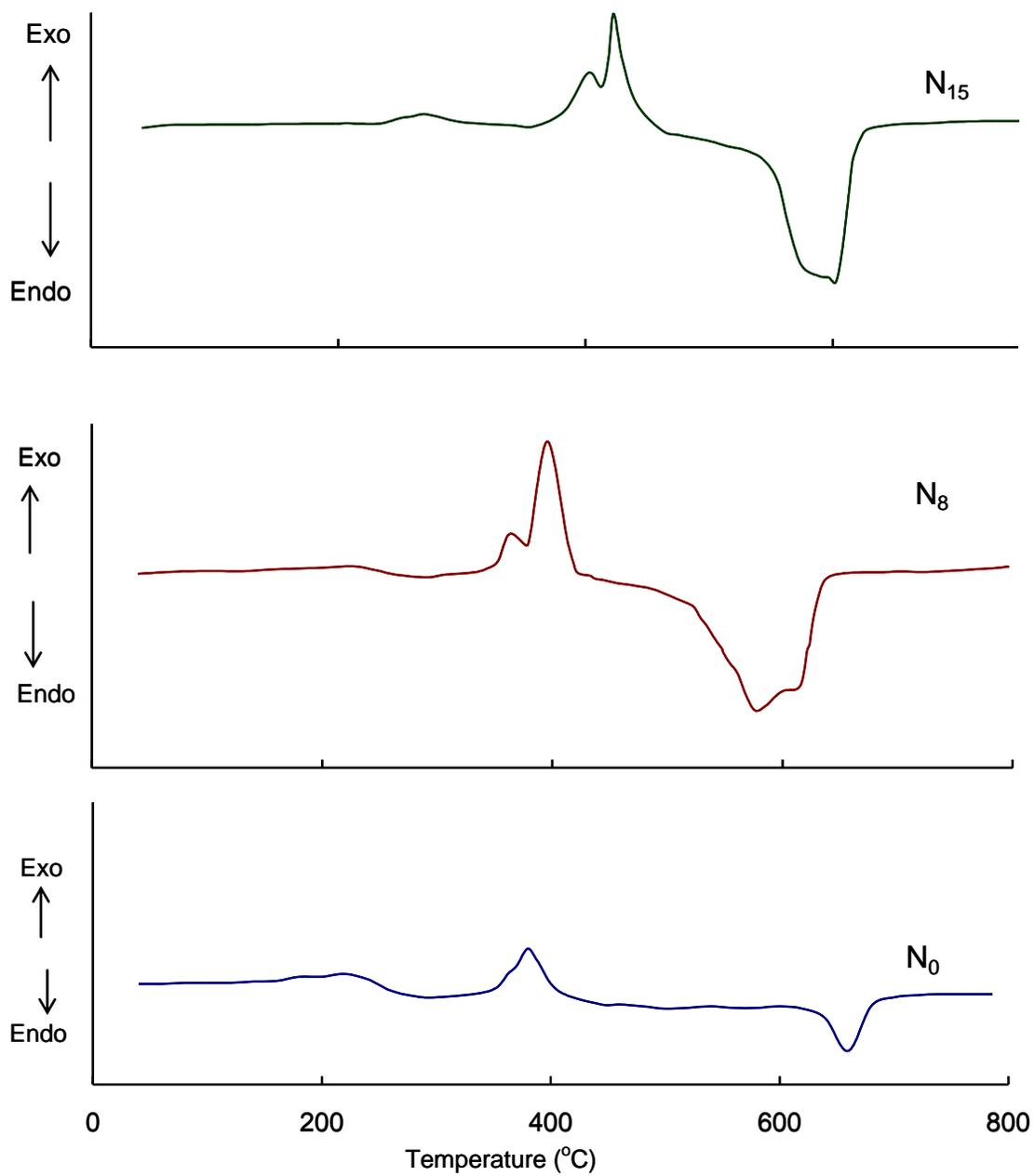
Fig. 5.4 Differential thermal analysis traces (DTA) for some of the PbO-Sb<sub>2</sub>O<sub>3</sub>-As<sub>2</sub>O<sub>3</sub>: NiO glass ceramics.
