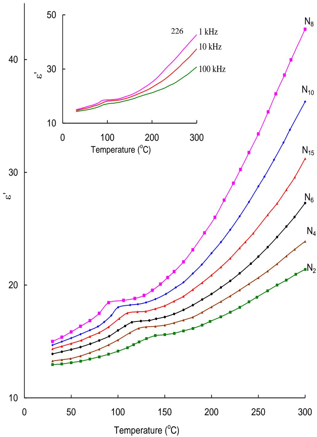
Fig. 5.9 A comparison plot of variation of dielectric constant with temperature at 1 kHz for  $\text{PbO-Sb}_2\text{O}_3\text{-As}_2\text{O}_3\text{: NiO}$  glass ceramics. Inset gives the variation of dielectric constant with temperature at different frequencies of glass ceramic  $N_8$ .
