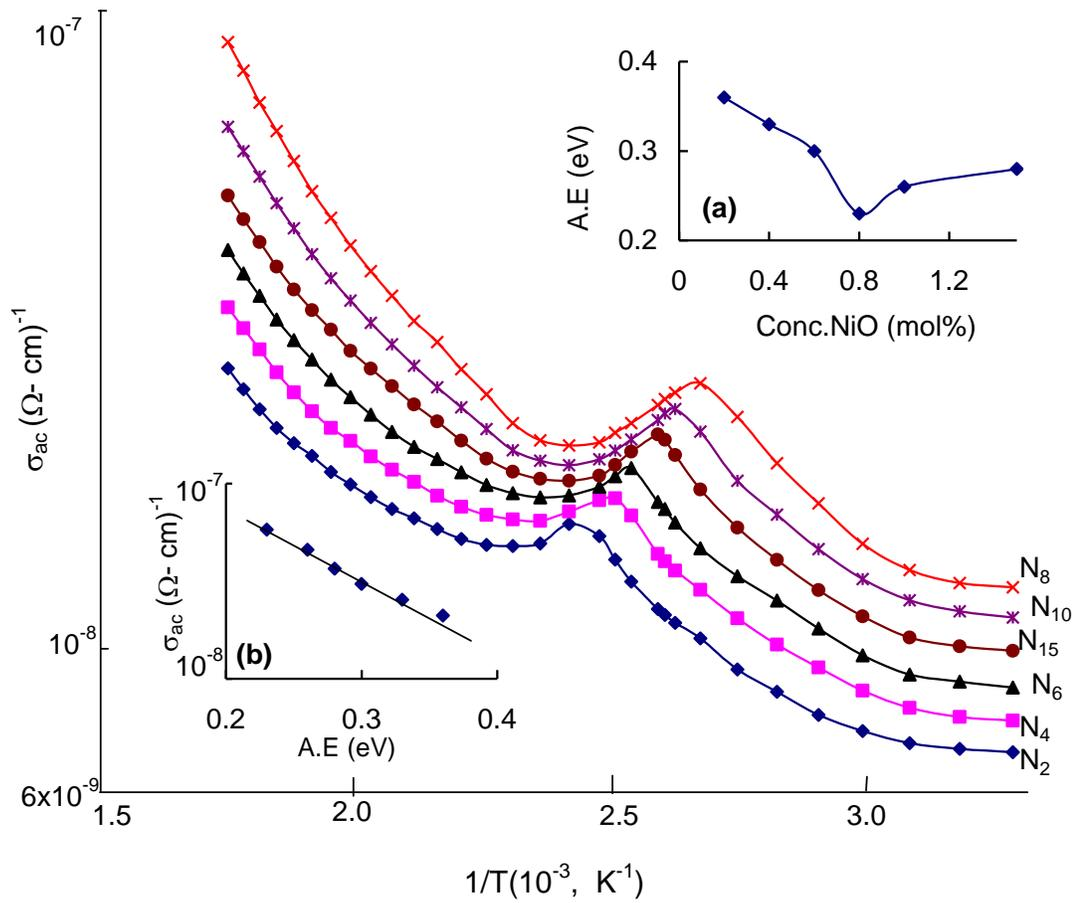
Fig. 5.11 Variation of  $\sigma_{ac}$  with  $1/T$  at 100 kHz of  $\text{PbO-Sb}_2\text{O}_3\text{-As}_2\text{O}_3\text{:NiO}$  glass ceramic. Inset (a) represents the variation of activation energy for conduction with NiO concentration. Inset (b) shows the variation of  $\log \sigma_{ac}(\omega)$  vs. activation energy for conduction.
