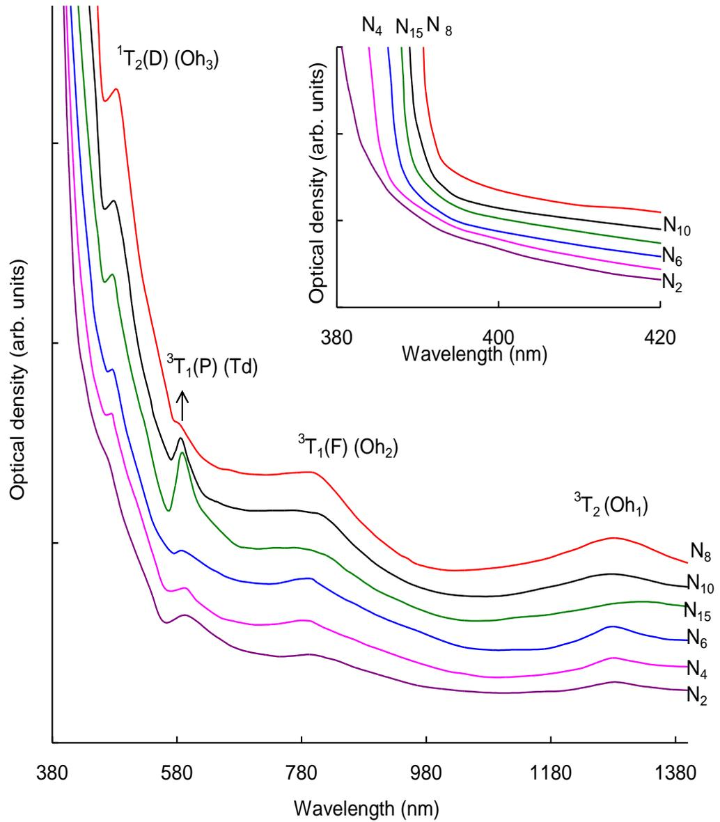
Fig. 5.5 Optical absorption spectra of PbO-Sb<sub>2</sub>O<sub>3</sub>-As<sub>2</sub>O<sub>3</sub>: NiO glass ceramics. Inset represents the absorption near the cutoff wavelength.
