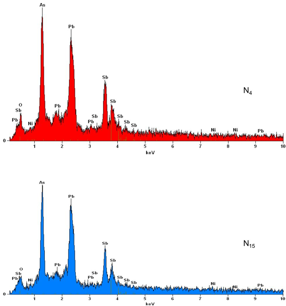
Fig. 5.2 EDS traces for some of the PbO-Sb<sub>2</sub>O<sub>3</sub>-As<sub>2</sub>O<sub>3</sub>: NiO glass ceramic samples.
