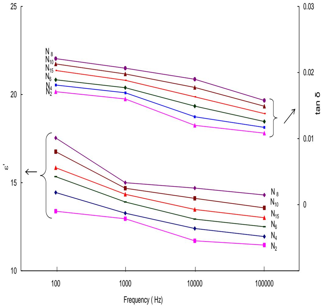
Fig. 5.8 Variation of dielectric constant and loss with frequency of PbO-Sb<sub>2</sub>O<sub>3</sub>-As<sub>2</sub>O<sub>3</sub>: NiO samples measured at room temperature
