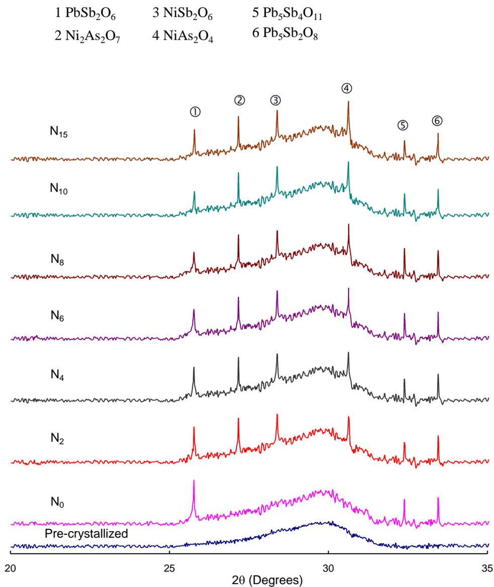
Fig. 5.3 XRD patterns of  $\text{PbO-Sb}_2\text{O}_3\text{-As}_2\text{O}_3$  glasses crystallized with different concentrations of  $\text{NiO}$ .
