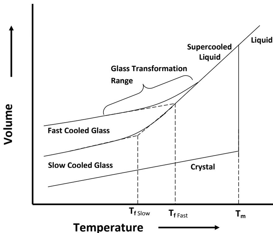
**Figure 1.1:** The two general ways of solidifying a melt namely, slow cooling to the crystalline state and the rapid quenching to the amorphous (glassy) state.
