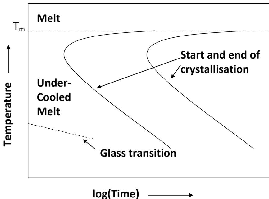
**Figure 1.2:** Schematic time-temperature-transformation diagram (TTT diagram) for the crystallisation of an undercooled melt.
