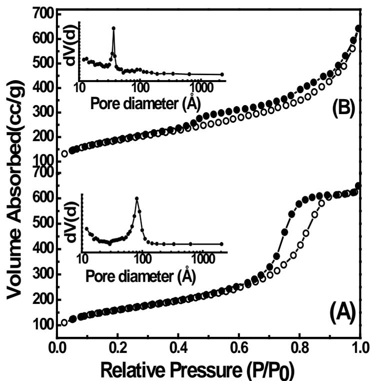
**Figure 6.3:** Nitrogen adsorption-desorption isotherm and pore size distribution (inset) of (A) MBG-75SNP (B) MBG-70SNP glasses.
