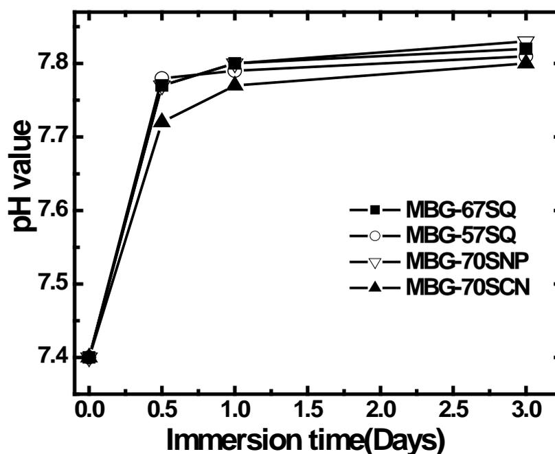
**Figure 6.5:** The variation of pH values of the SBF with soaking time on different MBG's.
