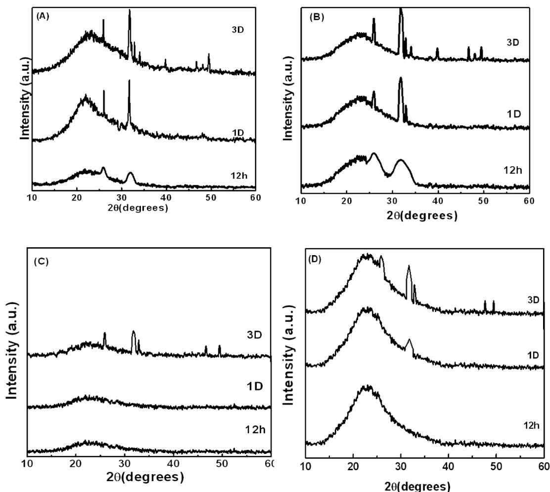
**Figure 6.7:** XRD pattern of (A) MBG-70SNP (B) MBG-75SNP (C) MBG-75SNC (D) MBG-70SNC after soaking in SBF for 12h, 1D and 3D.
