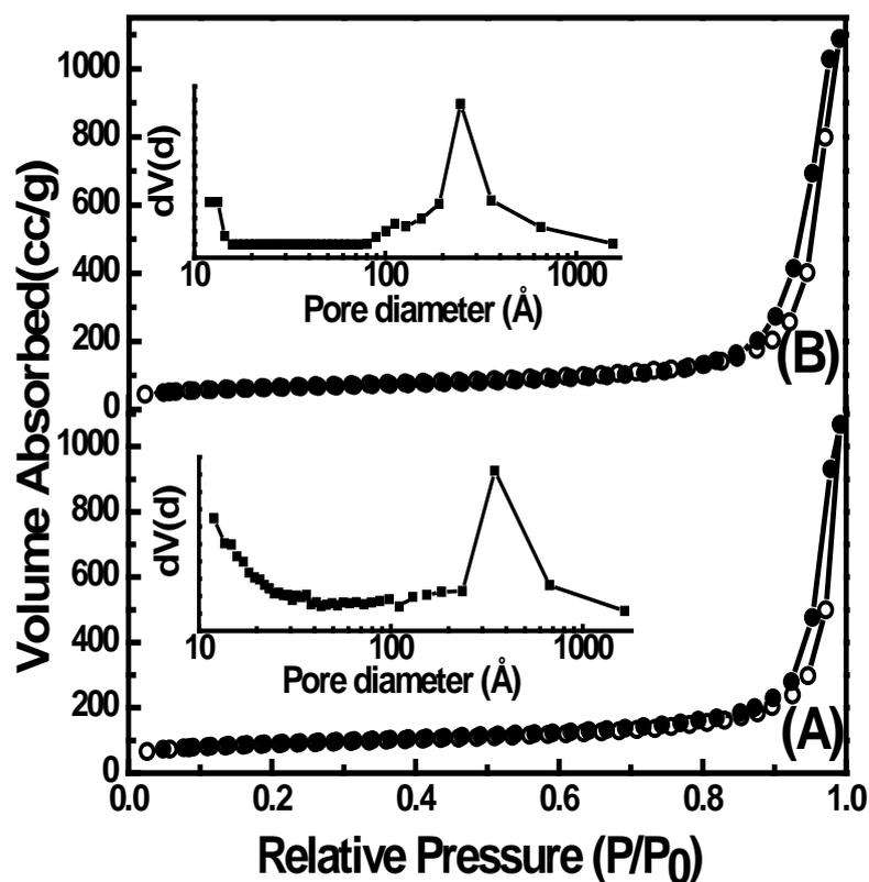
**Figure 6.2:** Nitrogen adsorption-desorption isotherm and pore size distribution (inset) of (A) MBG-67SQ (B) MBG-57SQ glasses.
