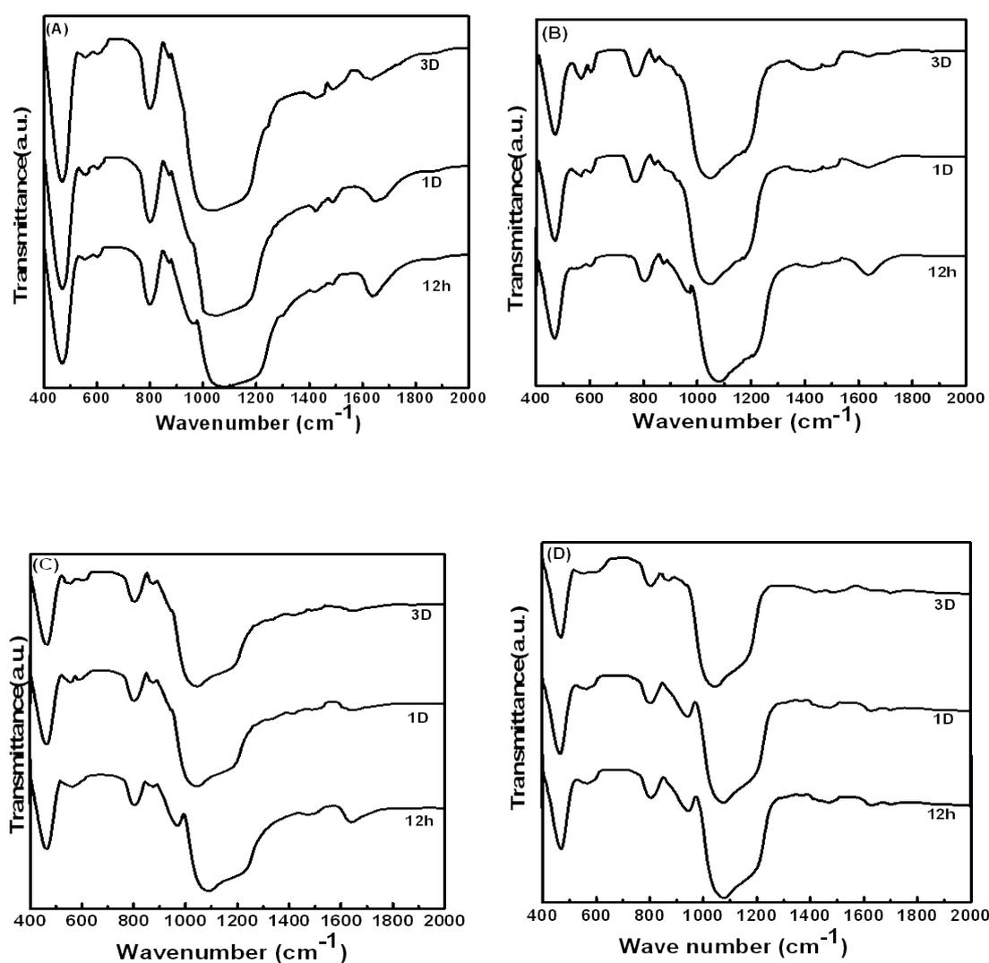
**Figure 6.8:** FTIR Spectra of (A) MBG-67SQ (B) MBG-62SQ (C) MBG-70SNP (D) MBG-70SNC glasses as a function of soaking time in SBF for 12h, 1D and 3D.
