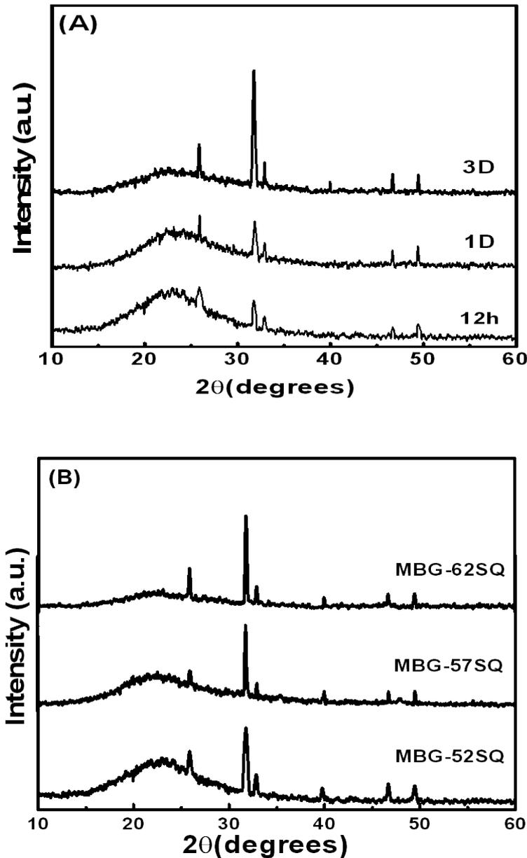
**Figure 6.6:** XRD pattern of (A) MBG-67SQ glass after soaking in SBF for 12h, 1D and 3D (B) MBG-62SQ, MBG-57SQ, and MBG-52SQ glass after soaking in SBF for 3D.
