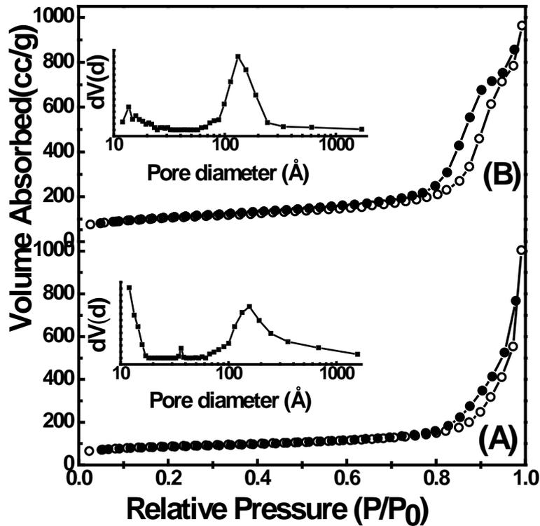
**Figure 6.4:** Nitrogen adsorption-desorption isotherm and pore size distribution (inset) of (A) MBG-75SNC (B) MBG-70SNC glasses.
