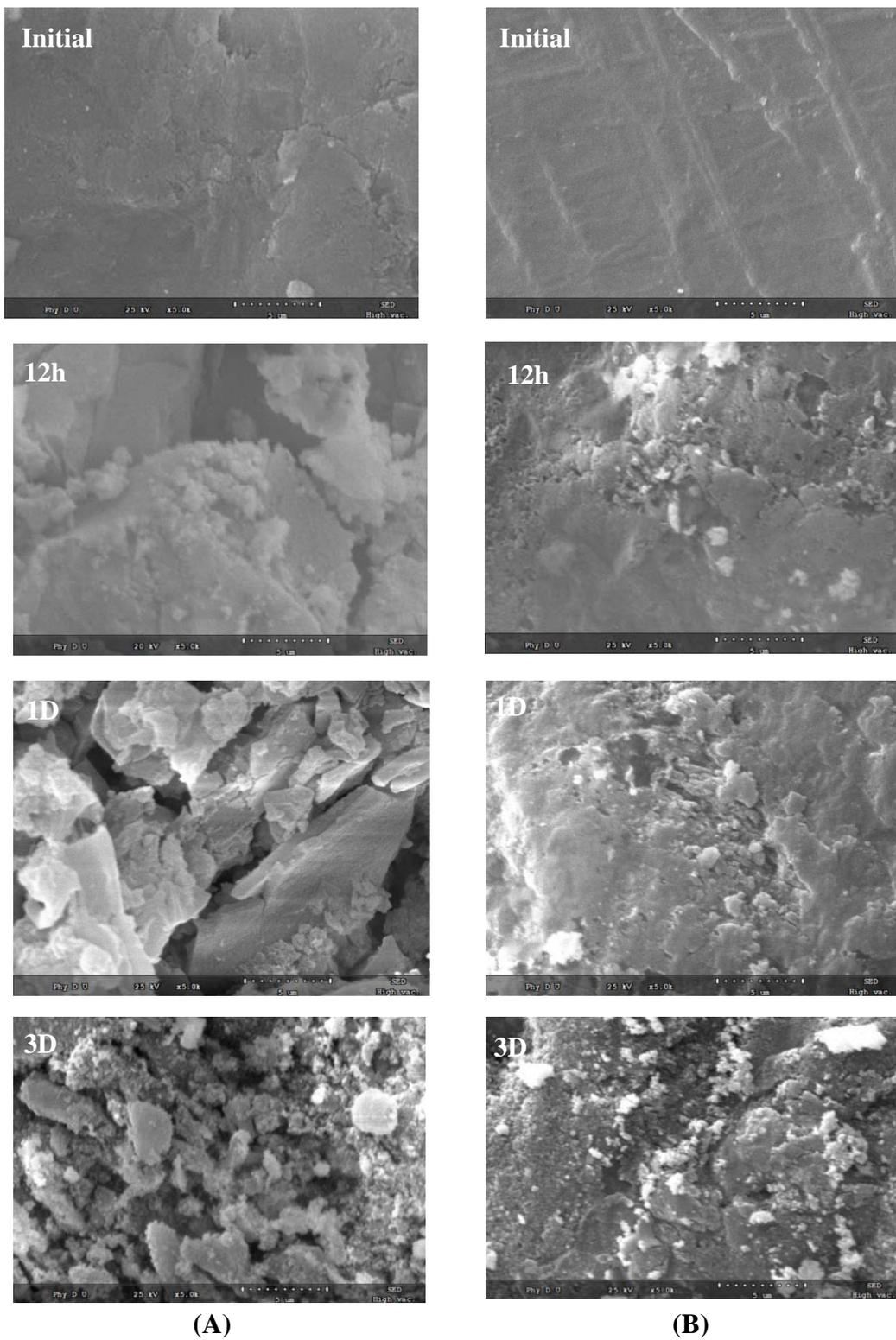
**Figure 6.10:** SEM micrographs of (A) MBG-70SNP (B) MBG-70SNC glasses before and after soaking in SBF for 12h, 1D and 3D.
