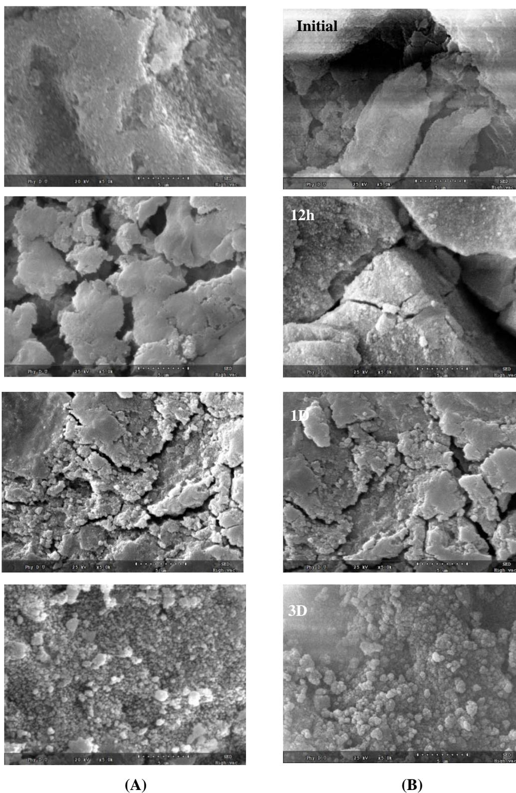
**Figure 6.9:** SEM micrographs of (A) MBG-67SQ (B) MBG-62SQ glasses before and after soaking in SBF for 12h, 1D and 3D.
