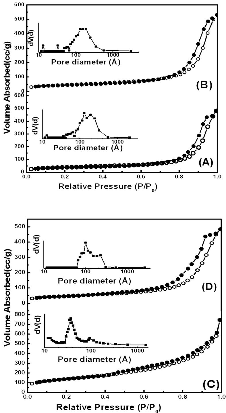
**Figure 6.11:** Nitrogen adsorption-desorption isotherm and pore size distribution (inset) of (A) MBG-67SQ (B) MBG-57SQ (C) MBG-70SNP (D) MBG-70SNC glasses after soaking in SBF for 3 days.
