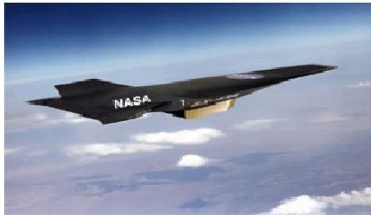
**Figure 1.3 NASA's X-43A-Hypersonic scramjet powered research aircraft designed to fly at speeds upto Mach 10 (Source:[http://www.nasa.gov/missions/research/f\\_scramjets.html](http://www.nasa.gov/missions/research/f_scramjets.html))**
