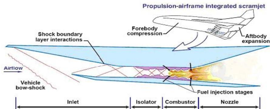
**Figure 1.2** The schematic diagram of the scramjet engine used in hypersonic vehicles (Source: <http://www.nasa.gov/centers/dryden/news/FactSheets/FS-040-DFRC.html>)
