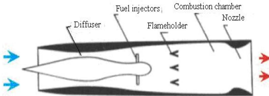
**Figure 1.1** The schematic diagram of the ramjet engine (Source://[www.aerospaceweb.org/question/propulsion/q0175.shtml](http://www.aerospaceweb.org/question/propulsion/q0175.shtml))
