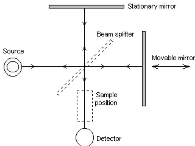
Figure 3.3 Schematic diagram of the operation of FTIR spectrometer
