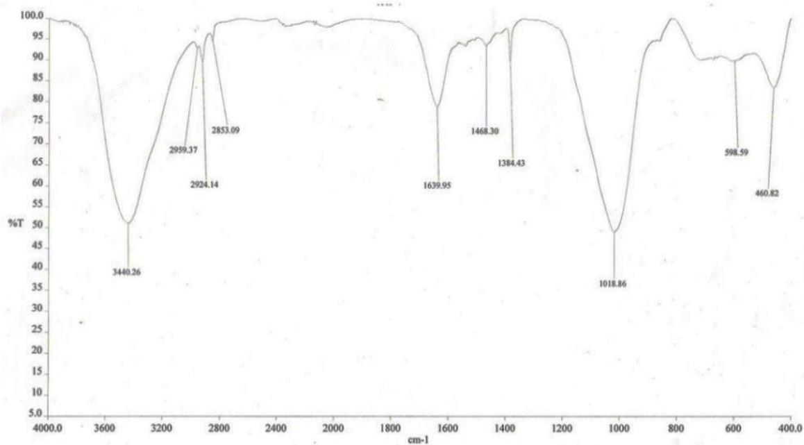
Figure 3.7 FTIR absorption spectrum of MgFZBFA
