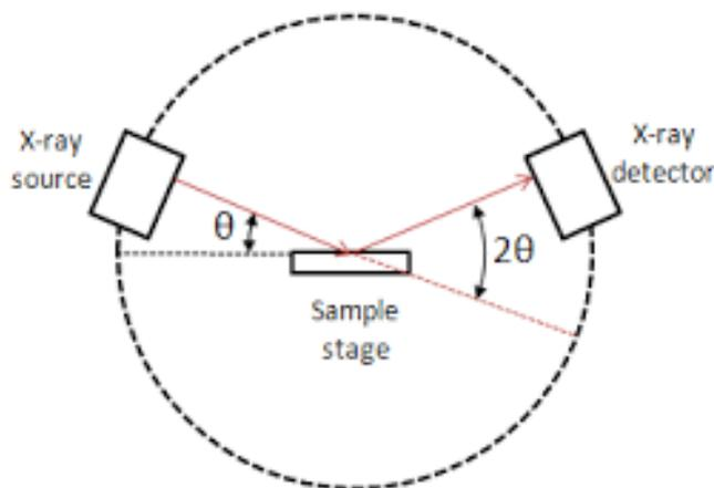
Figure 3.2 Schematic diagram of X-ray diffraction spectroscopy
