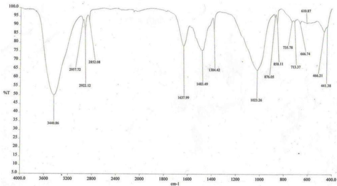
Figure 3.6 FTIR absorption spectrum of CaFZBFA
