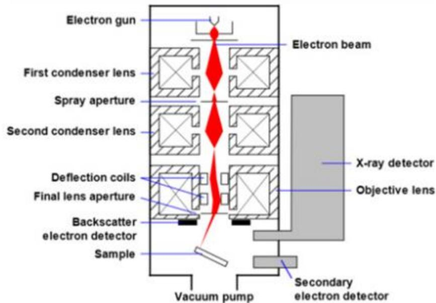
Figure 3.4 Diagrammatic illustration for scanning electron microscope
