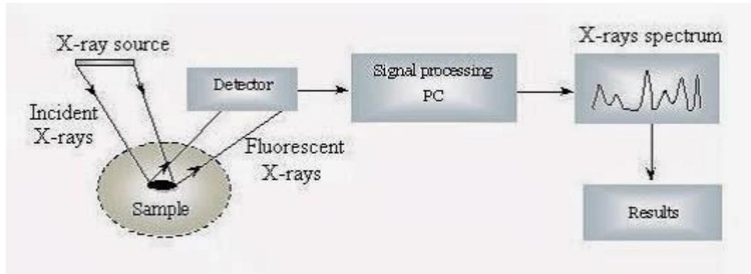
Figure 3.1 Schematic diagram of X-ray fluorescence instrumentation and technique
