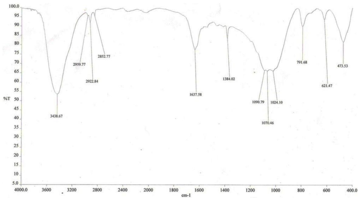
Figure 3.8 FTIR absorption spectrum of CaMZBFA
