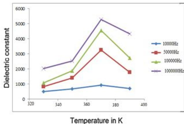
**Figure 7.11 Variation of dielectric constant vs. Temperature**
