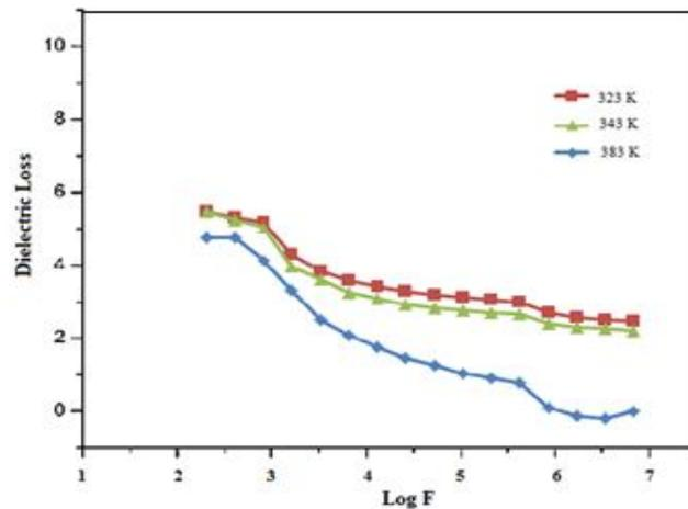
**Figure 7.10 Variation of dielectric loss vs. Log frequency**
