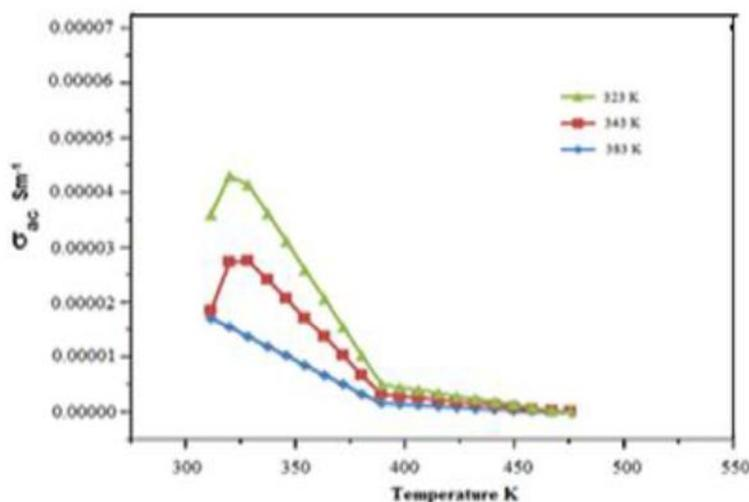
**Figure 7.12 Temperature variation of A.c. conductivity**
