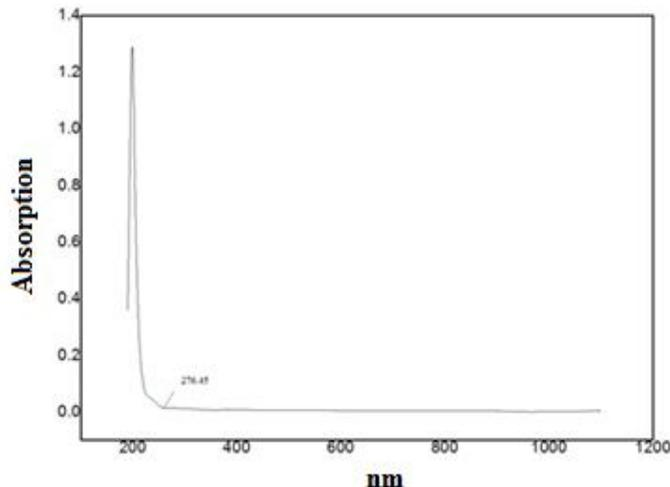
**Figure 7.4 Absorption spectra of GMnAc**
