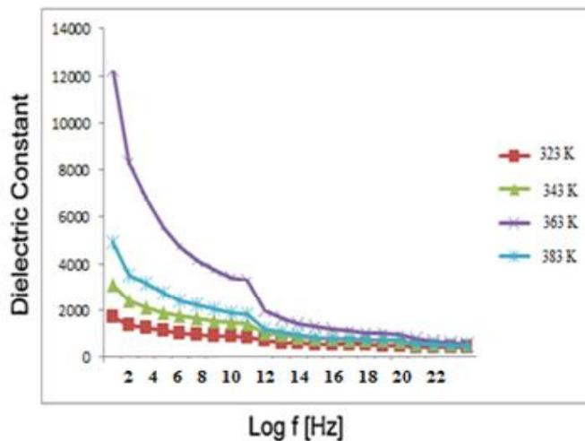
**Figure 7.9 Variation of dielectric constant vs. Log frequency**
