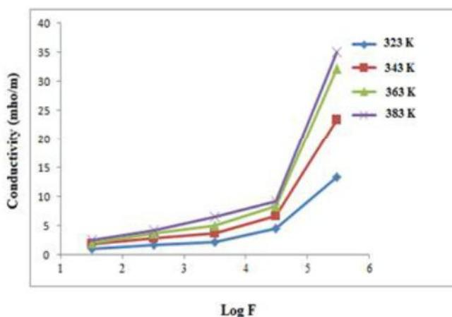
**Figure 7.17 Variation of Conductivity with Frequency**
