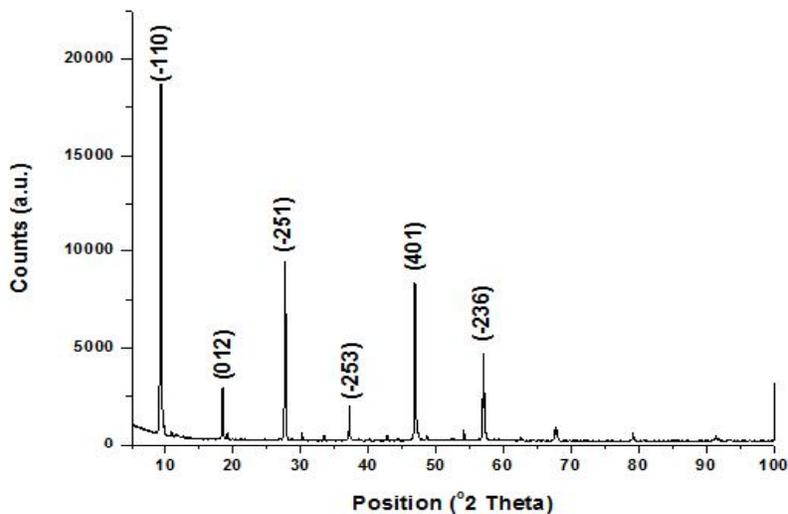
**Figure 7.2 Powder XRD pattern of GMnAc**
