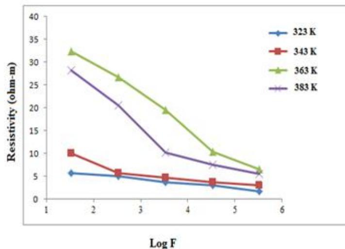
**Figure 7.16** Variation of Frequency with resistivity
