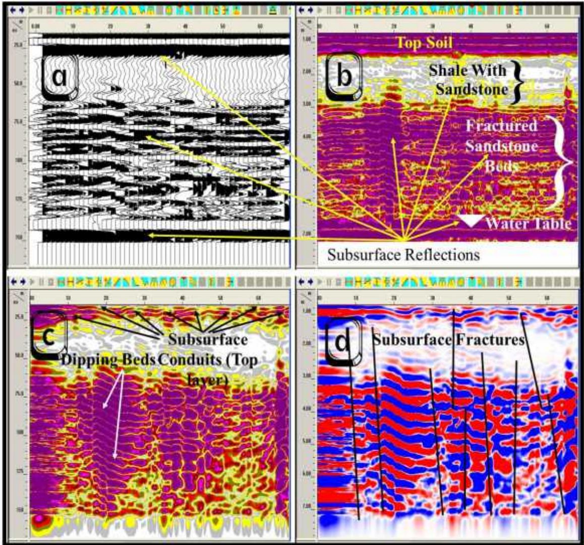
**Fig. 3.9** GPR profile image of South Point showing (a) wiggle trace format and processed and interpreted images (b, c and d) using RADAN software.
