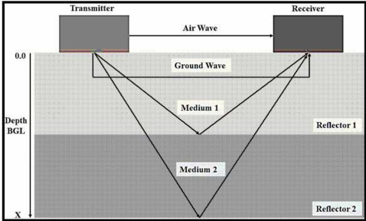
**Fig. 3.8** Theoretical principle of EM pathways between transmitter and receiver of a bistatic antenna configuration.
