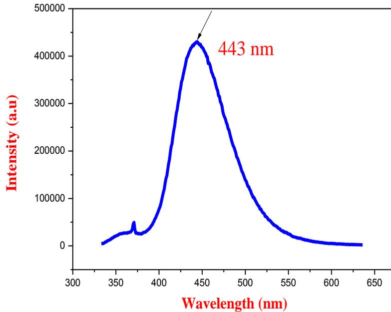
**Fig.5.12 Photoluminescence spectrum of C5SS crystal**
