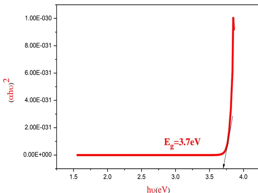
**Fig.5.11 Tauc's plot drawn between  $(\alpha h\nu)^2$  and  $h\nu$  of C5SS crystal**
