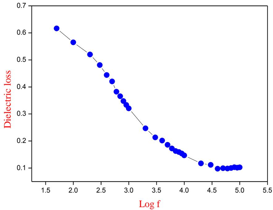
**Fig.5.14 Plot of dielectric loss vs log frequency of C5SS crystal**
