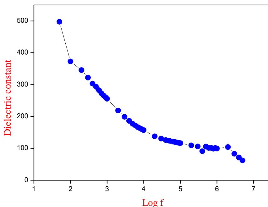
**Fig.5.13 Plot drawn between dielectric constant and log frequency of C5SS crystal**
