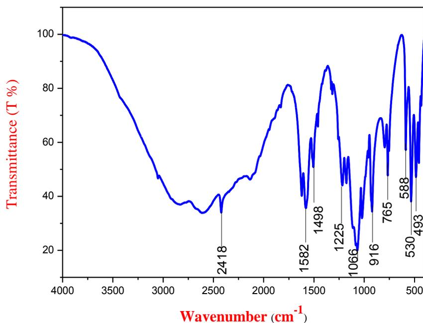
**Fig.5.8 FTIR spectrum of C5SS crystal**
