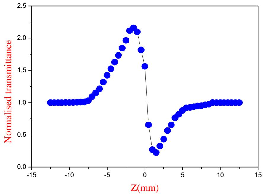
**Fig.5.17 Z-scan plot traced for C5SS crystal in closed aperture mode**
