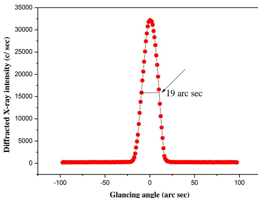
**Fig.5.7 HRXRD curve of C5SS crystal**
