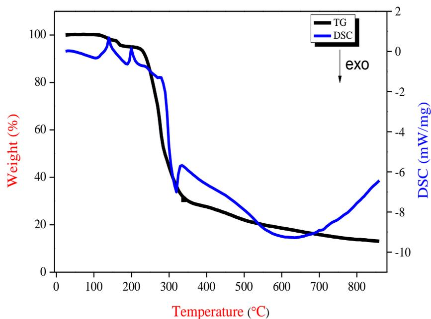
**Fig.5.9 TG-DSC thermogram of C5SS crystal**
