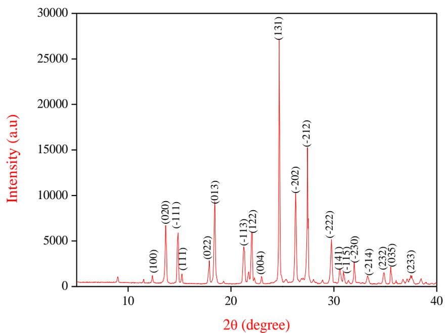
**Fig.5.6** Powder X-ray diffraction pattern of C5SS crystal
