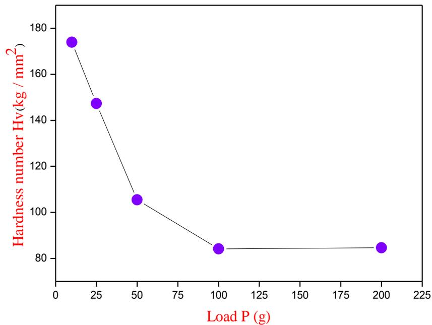
**Fig.5.15 Plot drawn between Vicker's hardness number ( $H_v$ ) and load (P) of C5SS crystal**
