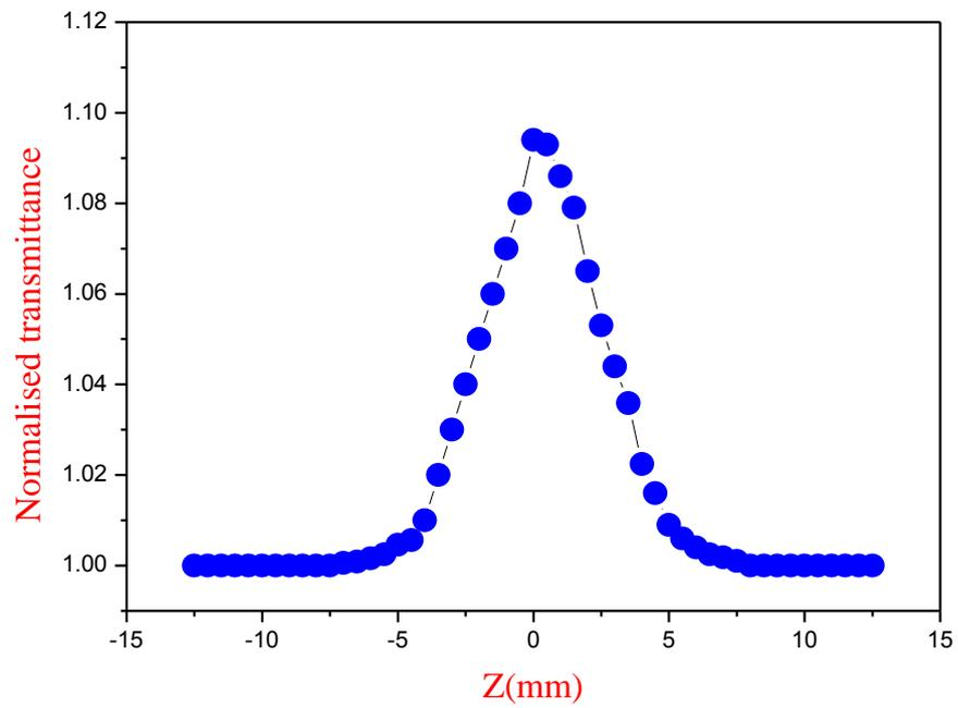
**Fig.5.18 Z-scan plot traced for C5SS crystal in open aperture mode**
