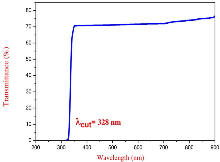
**Fig.5.10 UV-Visible transmission spectrum of C5SS crystal**
