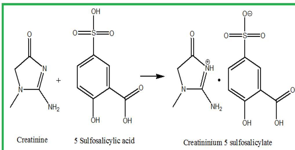
**Fig.5.1 Material synthesis scheme for C5SS compound**
