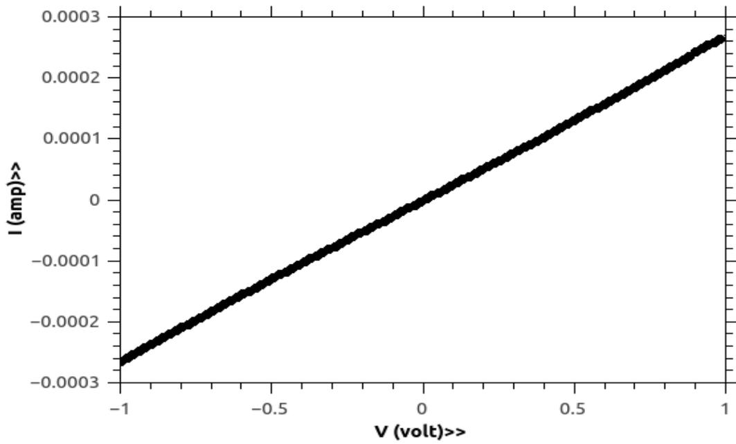
Fig. 6.3: Current- Voltage (I-V) Characteristics of LN0MT film
