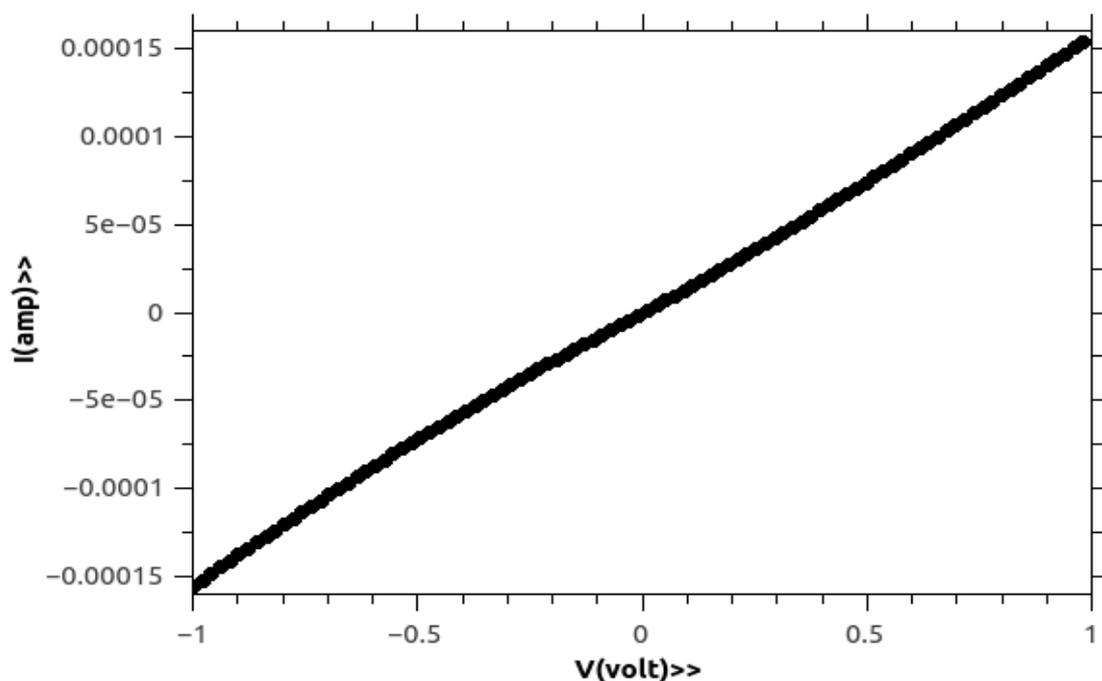
Fig. 6.6: Current- Voltage (I-V) Characteristics of LA0MT film
