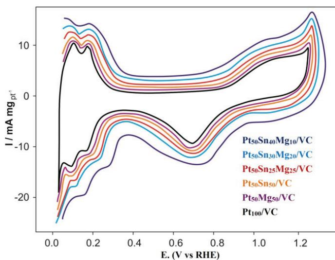
**Fig. 4.5-(a) Cyclic voltammogram representations of Pt<sub>50</sub>Sn<sub>40</sub>Mg<sub>10</sub>/VC, Pt<sub>50</sub>Sn<sub>30</sub>Mg<sub>20</sub>/VC, Pt<sub>50</sub>Sn<sub>25</sub>Mg<sub>25</sub>/VC, Pt<sub>50</sub>Sn<sub>50</sub>/VC, Pt<sub>50</sub>Mg<sub>50</sub>/VC and Pt<sub>100</sub>/VC nanoparticles in the absence of fuel.**
