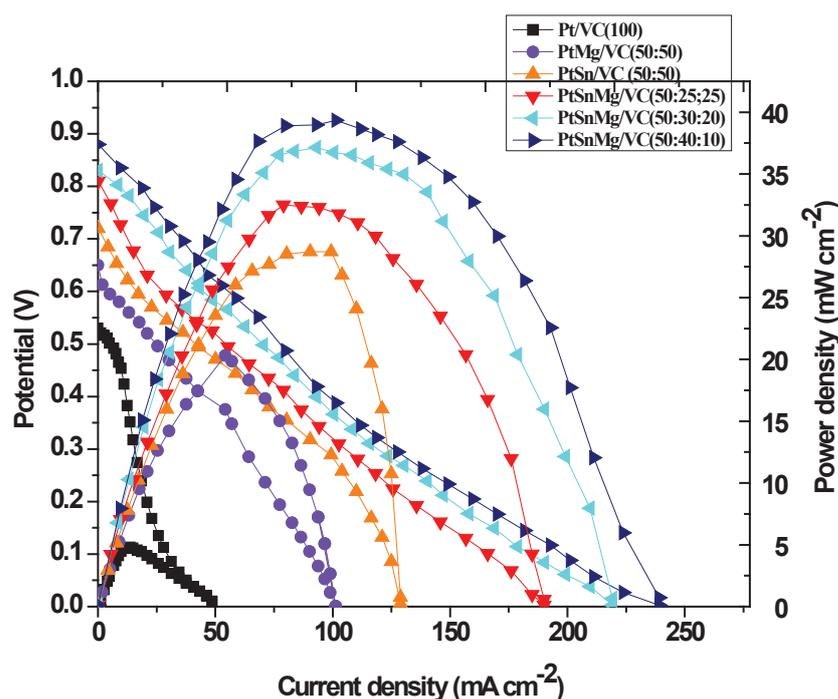
**Fig 4.7 Potential difference and power density curves for Pt<sub>50</sub>Sn<sub>40</sub>Mg<sub>10</sub>/VC, Pt<sub>50</sub>Sn<sub>30</sub>Mg<sub>20</sub>/VC, Pt<sub>50</sub>Sn<sub>25</sub>Mg<sub>25</sub>/VC, Pt<sub>50</sub>Sn<sub>50</sub>/VC, Pt<sub>50</sub>Mg<sub>50</sub>/VC and Pt<sub>100</sub>/VC nanoparticles.**
