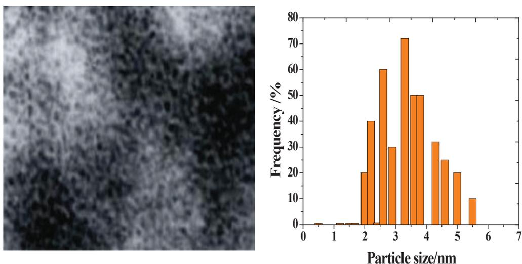
**Fig. 4.3** Micrographs of transmission electron microscopy and its histograms of Pt/Sn/Mg alloyed nanoparticles on VC support.
