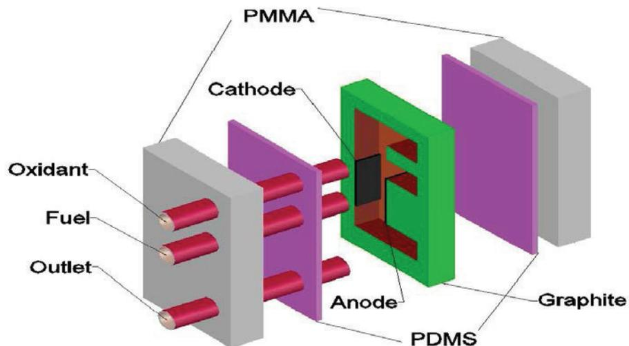
**Fig. 4.1 Schematic of the E-shaped membraneless laminar flow based fuel cell with graphite plates molded with poly(dimethylsiloxane) and sealed with poly(methylmethacrylate).**
