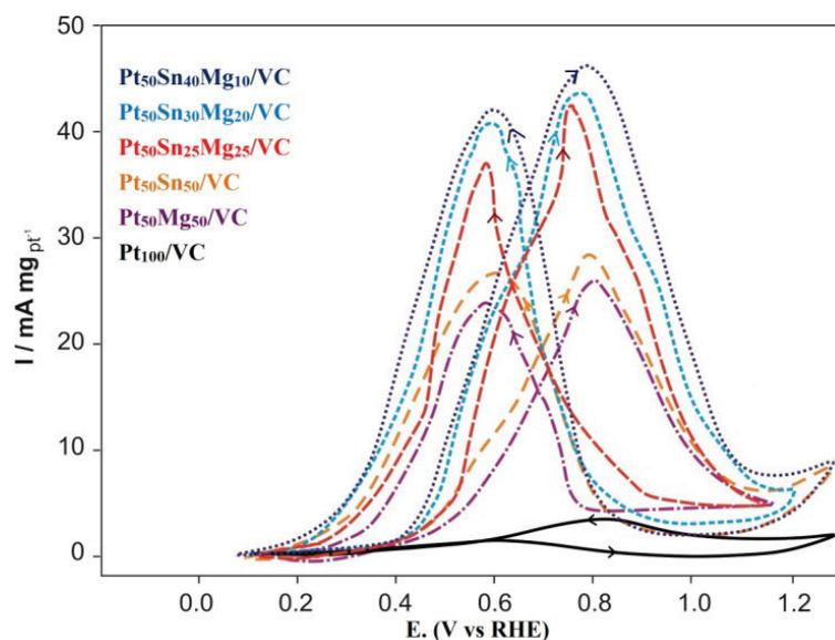
**Fig 4.5-(b) Cyclic voltammogram representations of Pt<sub>50</sub>Sn<sub>40</sub>Mg<sub>10</sub>/VC, Pt<sub>50</sub>Sn<sub>30</sub>Mg<sub>20</sub>/VC, Pt<sub>50</sub>Sn<sub>25</sub>Mg<sub>25</sub>/VC, Pt<sub>50</sub>Sn<sub>50</sub>/VC, Pt<sub>50</sub>Mg<sub>50</sub>/VC and Pt<sub>100</sub>/VC nanoparticles in the presence of fuel.**
