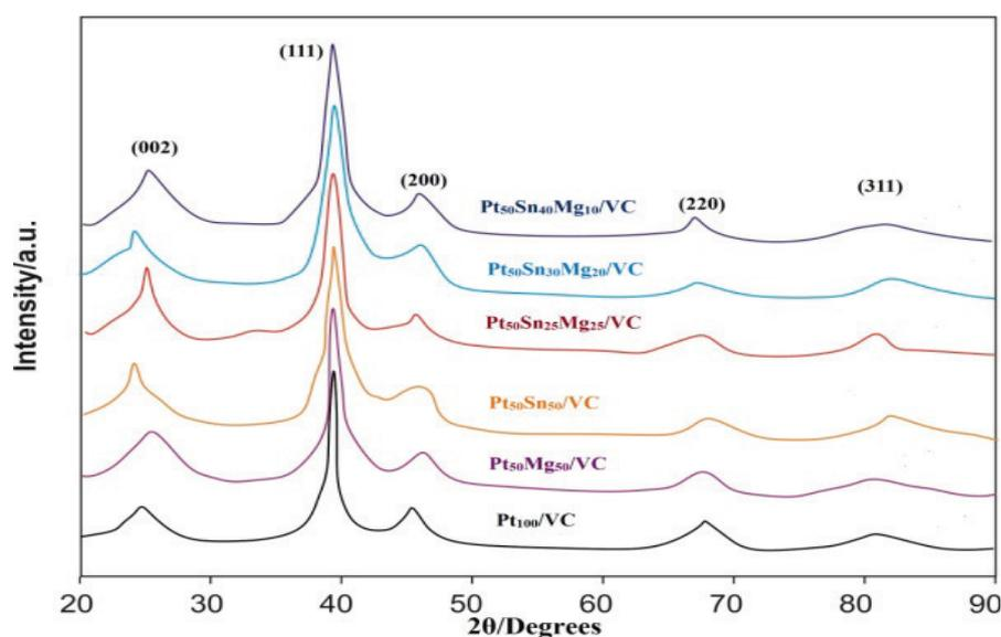
Fig. 4.2 X-ray diffraction peaks of Pt–Sn–Mg (50:40:10), Pt–Sn–Mg (50:30:20), Pt–Sn–Mg (50:25:25), Pt–Mg (50:50), Pt–Sn (50:50) and Pt (100) nanoparticles.
