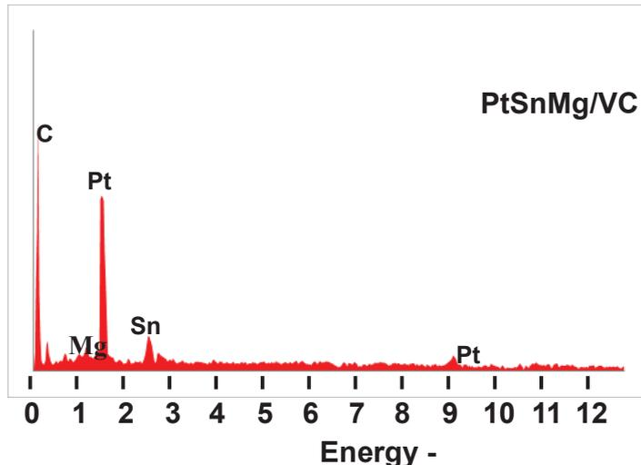
**Fig. 4.4** Microanalysis spectrum of EDX for Pt/Sn/Mg nanoparticles on VC support.
