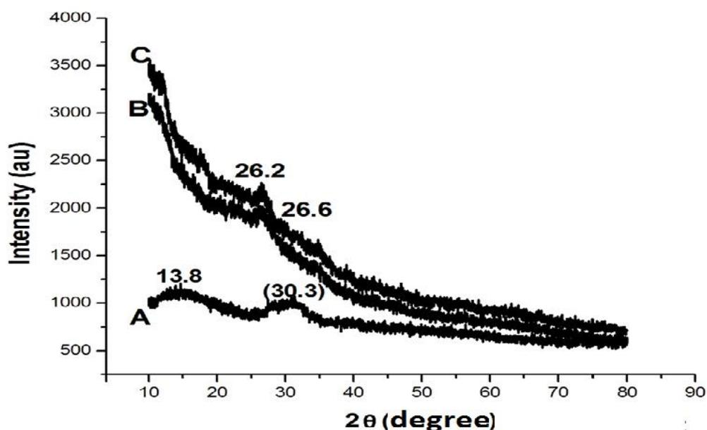
Fig. 5.4 XRD spectra for A, B and C (A for  $t = 6$  hours, B for 24 hours, C for 48 hours)
