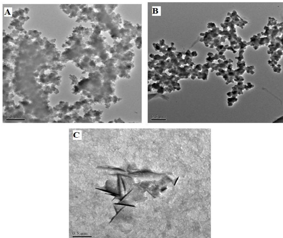
**Fig. 5.2 TEM micrographs of the samples A, B and C (A for polymerization time  $t= 6$  hours, B for  $t= 24$  hours, C for  $t= 48$  hours)**
