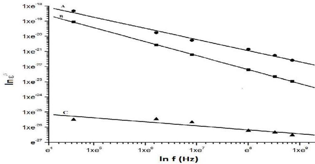
**Fig. 5. 6 Dielectric loss vs. frequency for A, B and C (A for t = 6 hours, B for 24 hours, C for 48 hours)**
