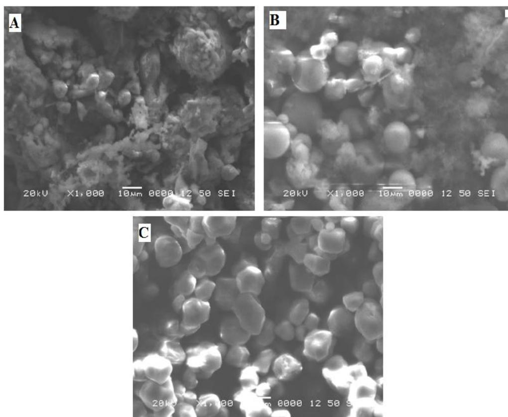
**Fig.5. 1 SEM micrograph of the composite samples A, B and C (A for polymerization time  $t = 6$  hours, B for  $t = 24$  hours, C for  $t = 48$  hours)**
