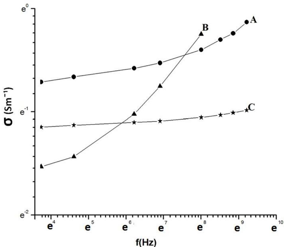
**Fig. 5.7** Conductivity vs. Frequency for A, B and C (A for polymerization time  $t= 6$  hours, B for  $t= 24$  hours, C for  $t= 48$  hours)
