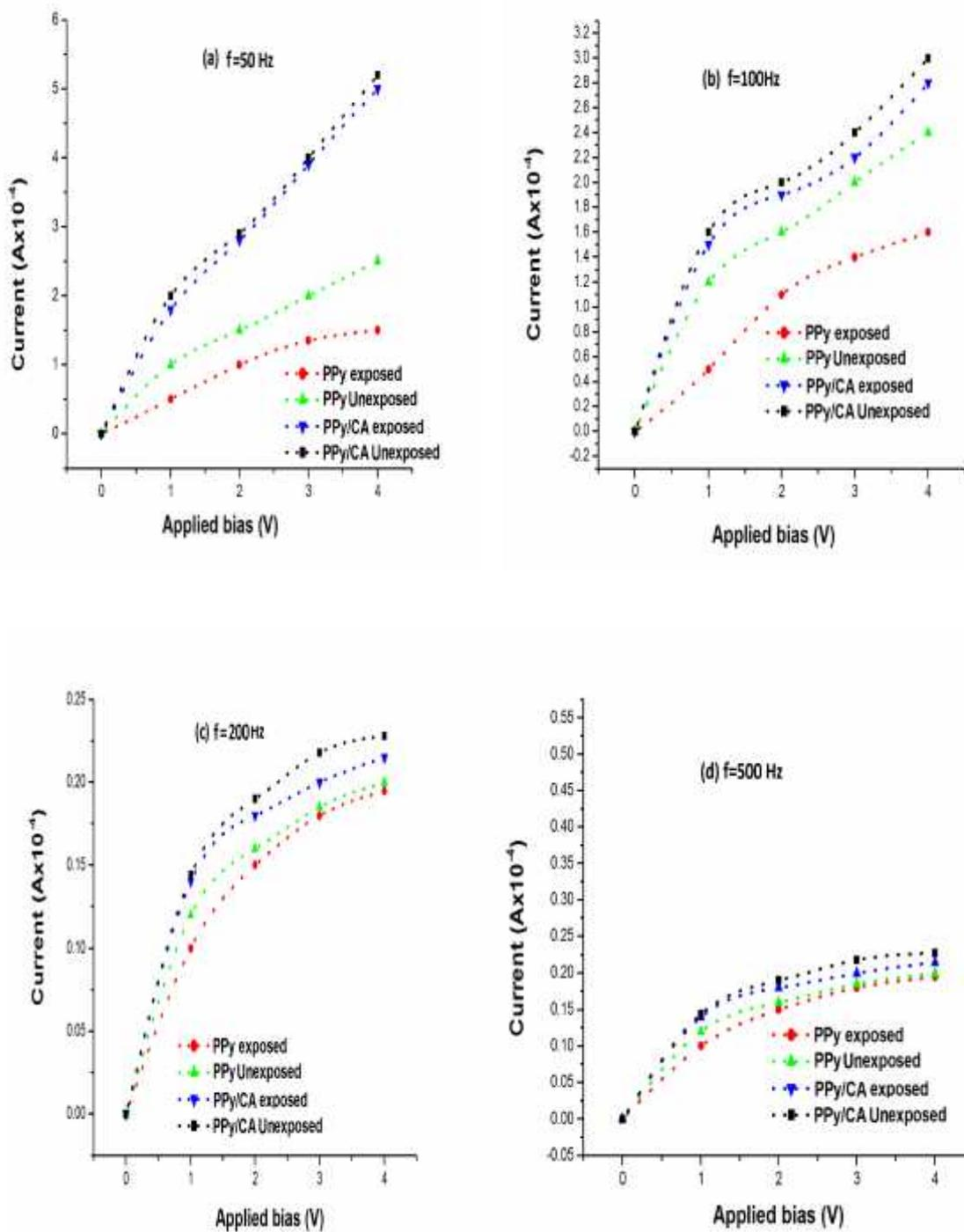
**Fig.3.8 I-V characteristics of PPy and PPy/CA composite for applied frequencies of (a) 50Hz (b) 100 Hz (c) 200 Hz and (d) 500 Hz**
