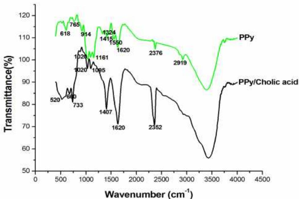
Fig. 3.2 FTIR spectra of PPy and PPy-cholic acid composite
