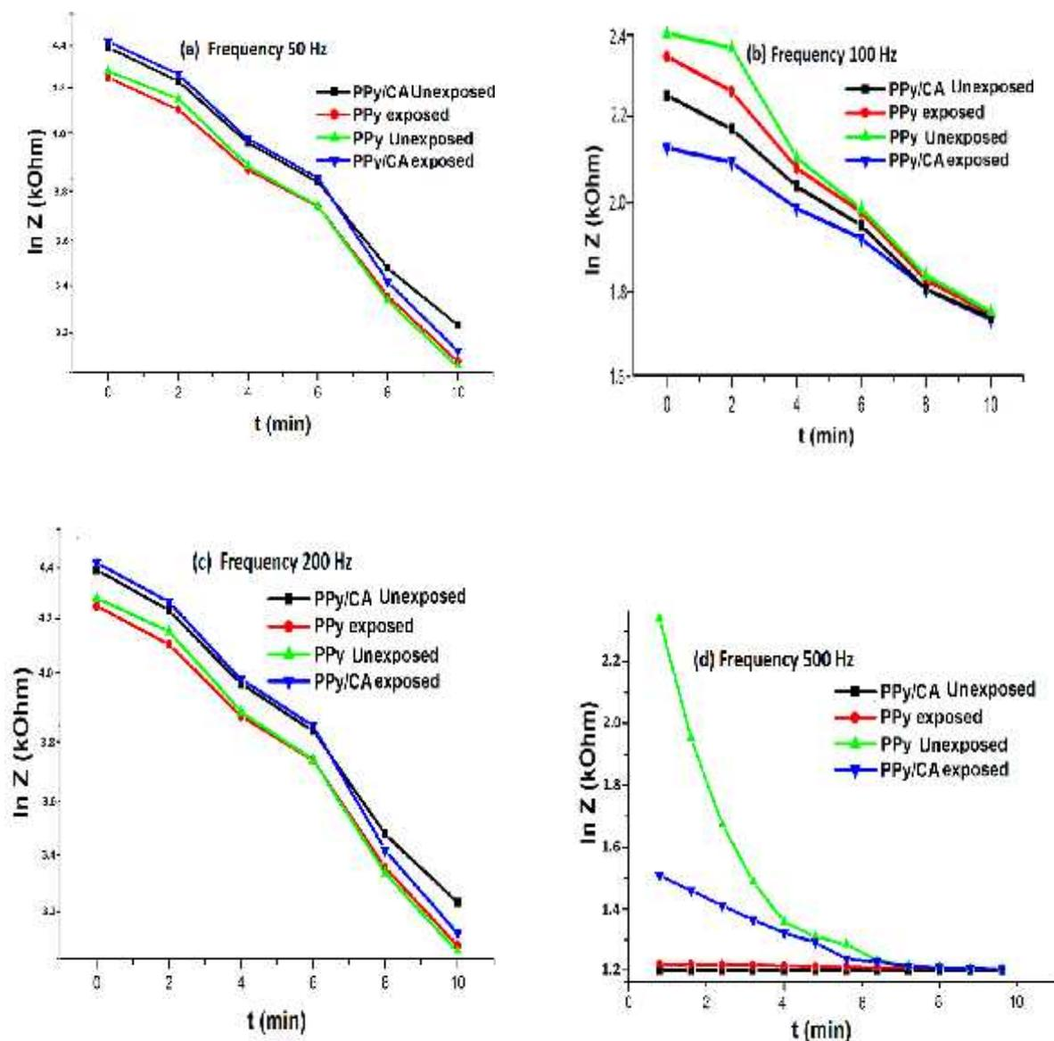
Fig. 3.9 Impedance vs time in four different applied frequencies (a) 50Hz (b) 100 Hz (c) 200 Hz and (d) 500 Hz
