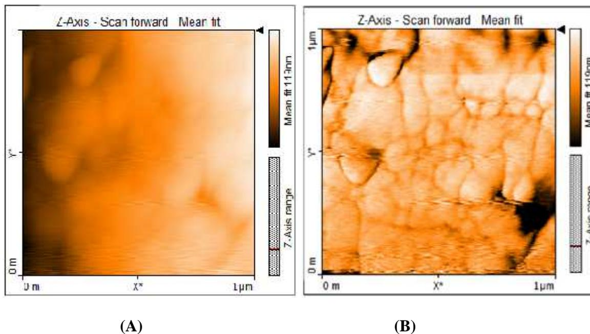
**Fig.3.5 AFM images of DBSA doped PPy (A) and PPy/Cholic Acid composite (B)**
