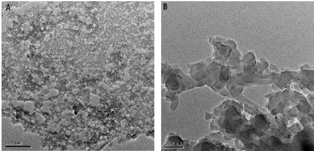
**Fig.3.4 TEM images of PPy (A) and PPy/Cholic Acid composite (B)**
