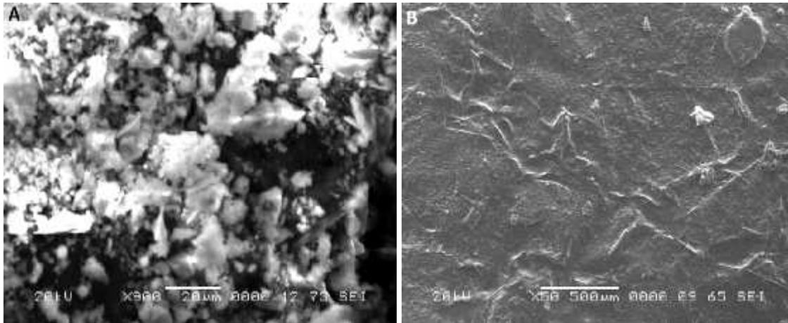
**Fig. 3.3 SEM images of PPy (A) and PPy/cholic acid composite (B)**
