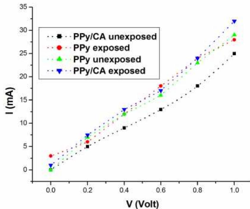
**Fig. 3.6 I-V characteristics for DBSA doped PPy and PPy/ Cholic Acid composite**
