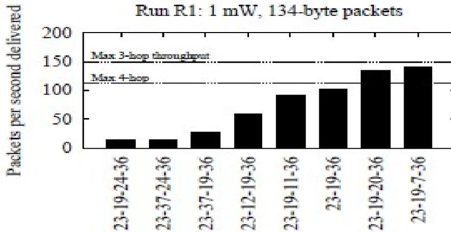
**Figure 6.2:** Throughput available between one pair of nodes, 23 and 36, along the best eight routes tested. The shortest of the routes does not perform the best, and there are a number of routes with the same number of hops that provide very different throughput.
