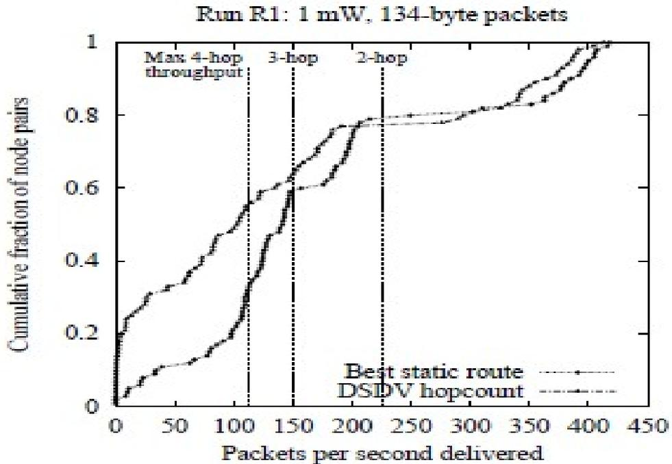
**Figure 6.1:** When using the minimum hop-count metric, DSDV chooses paths with far less throughput than the best available routes. Each line is a throughput CDF for the same 100 randomly selected node pairs. The left curve is the throughput CDF of DSDV with minimum hop-count. The right curve is the CDF of the best throughput between each pair, found by trying a number of promising paths. The dotted vertical lines mark the theoretical maximum throughput of routes of each hop-count.
