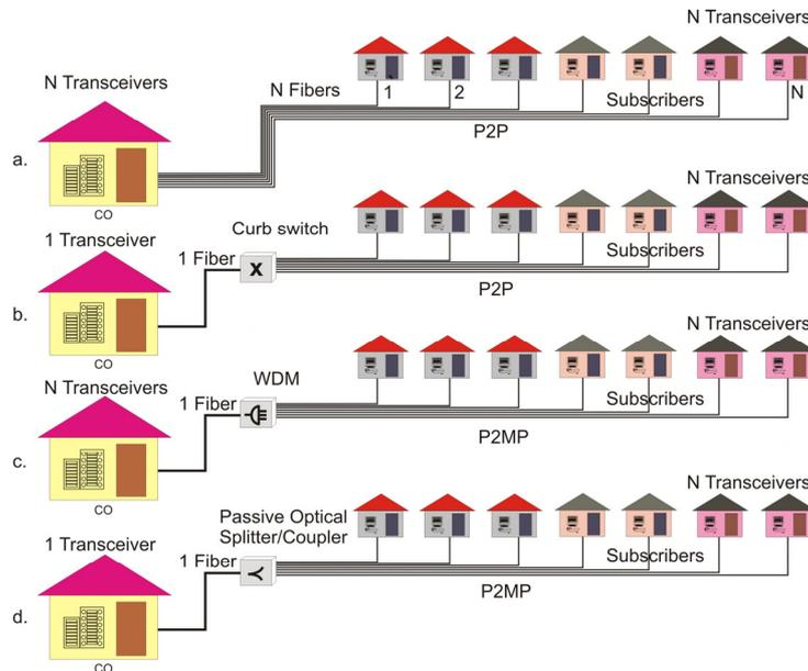
Figure 1.1: Different architectures of access network
