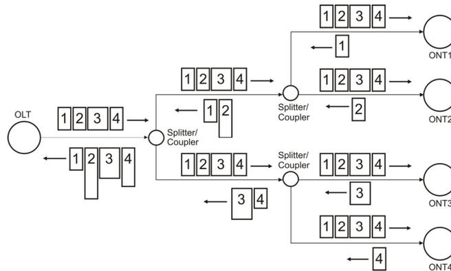
Figure 1.3: Signal transmission in a TDM/TDMA PON
