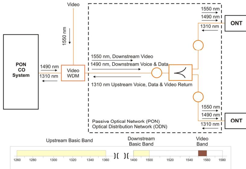
Figure 1.4: ITU-T G.983.3 PON Wavelength Allocation Scheme
