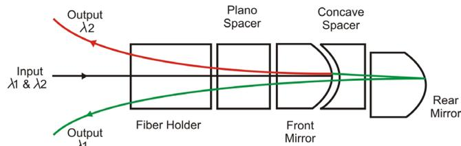
Figure 1.10: Reflective Optics based WDM
