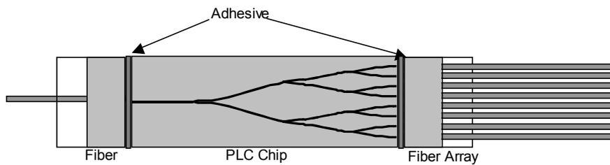
Figure 1.8: Internal structure of a 1x8 PLC splitter
