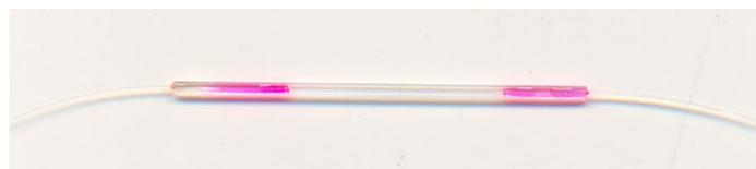
Figure 1.7: Photograph of a 1x2 Fused Coupler
