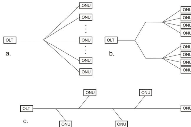
Figure 1.5: Splitting strategies in a TDM-PON: (a) one-stage splitting
