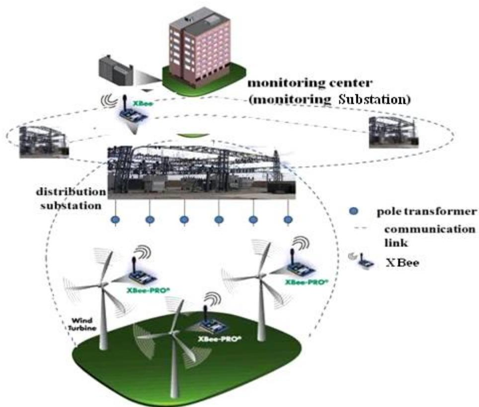
**Figure 1.1 Wireless Personal Area Network (WPAN) for Electrical Grid Monitoring (Smart Energy Monitoring)**
