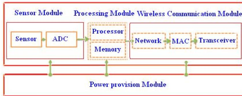
**Figure 1.2 Functional Block Diagram of Wireless Sensor Node**
