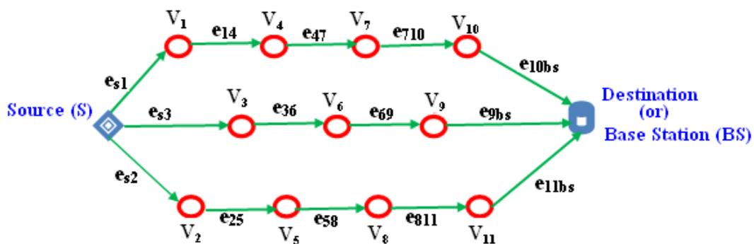
**Figure 4.2 Network Model for Multipath Routing**
