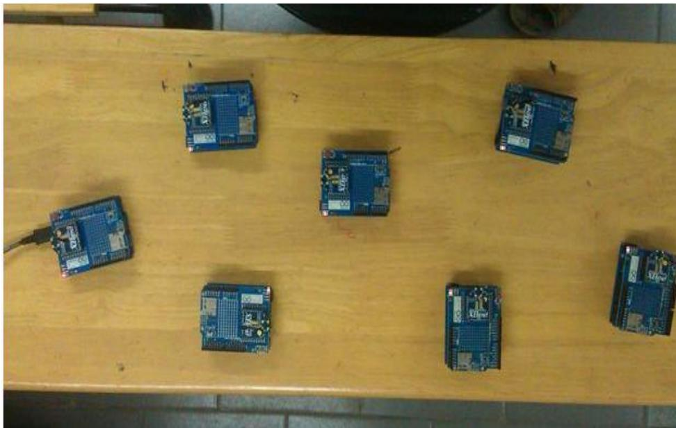
**Figure 3.6 Experiment on Networking with XBEE Series2**
