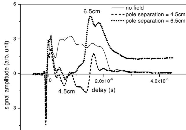
Fig.3.11: Effect of magnetic field on the signal. Two different field strengths are applied.
