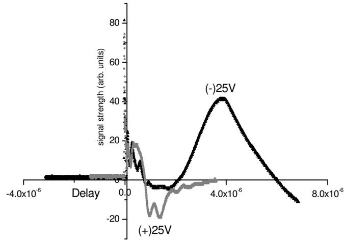
Fig.3.6: Signals with positive and negative bias
