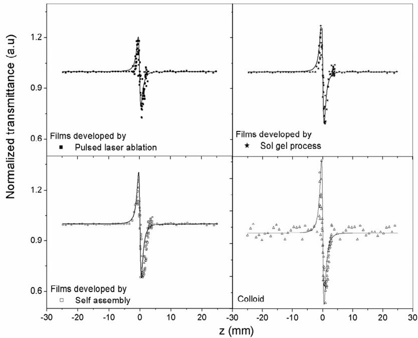
Figure 4.7: Closed aperture z-scan traces of ZnO thin films and colloid at an intensity of 220 MW/cm<sup>2</sup> for an irradiation wavelength of 532 nm
