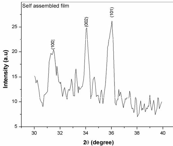
Figure 4.3: XRD pattern of ZnO self assembled film
