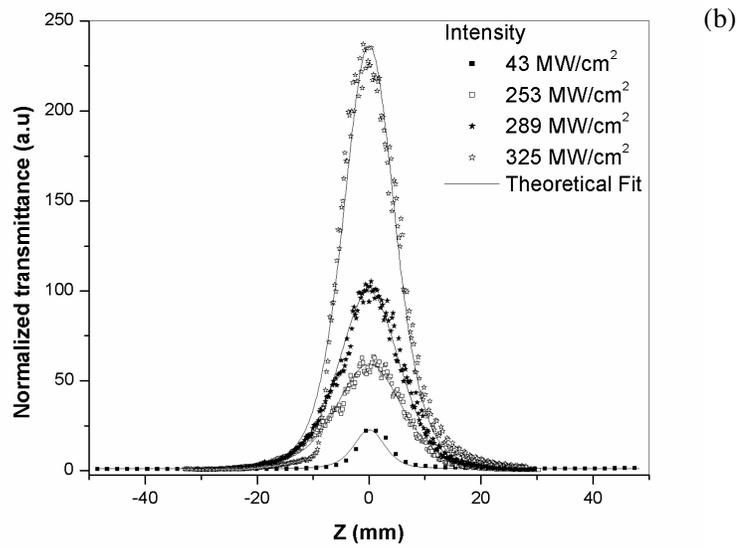
Figure 4.9: Open aperture z-scan curves of (a): ZnO colloid (b): ZnO self assembled films of size 300 nm at a wavelength of 532 nm for different irradiation intensities
