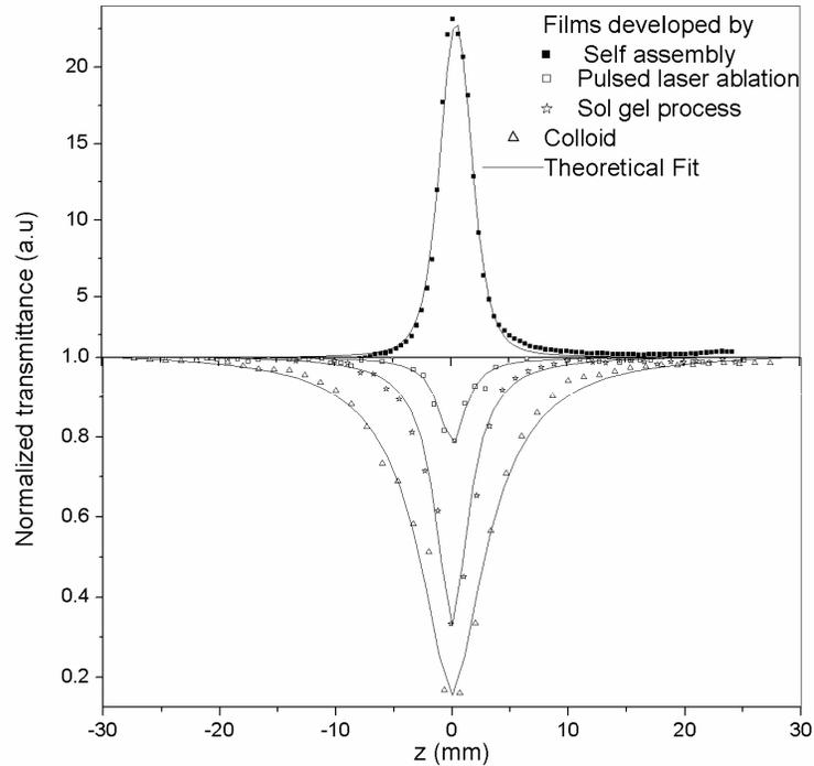
Figure 4.6: Open aperture z-scan traces of ZnO thin films and colloid at an intensity of  $220 \text{ MW/cm}^2$  for an irradiation wavelength of 532 nm
