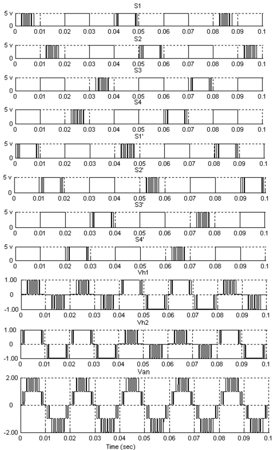
**Figure 3.6 Five-level sequential switching HAPOD pulse pattern**
