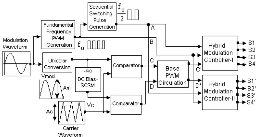
**Figure 3.7 Scheme of five-level sequential switching HSCSM**
