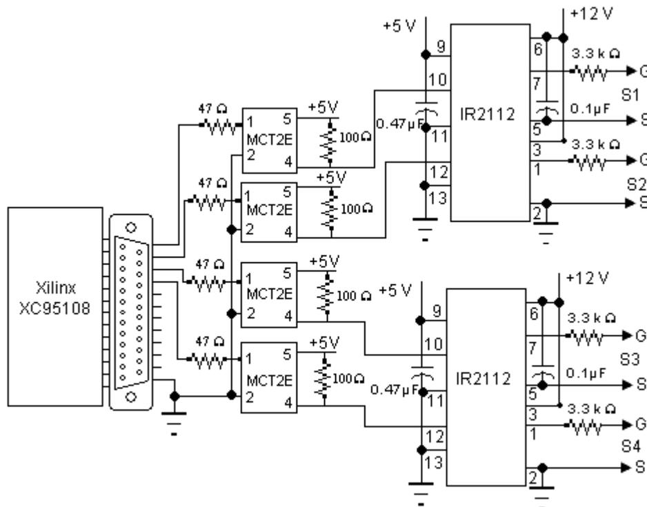
**Figure 3.17 Isolation and driver circuit for one inverter cell**
