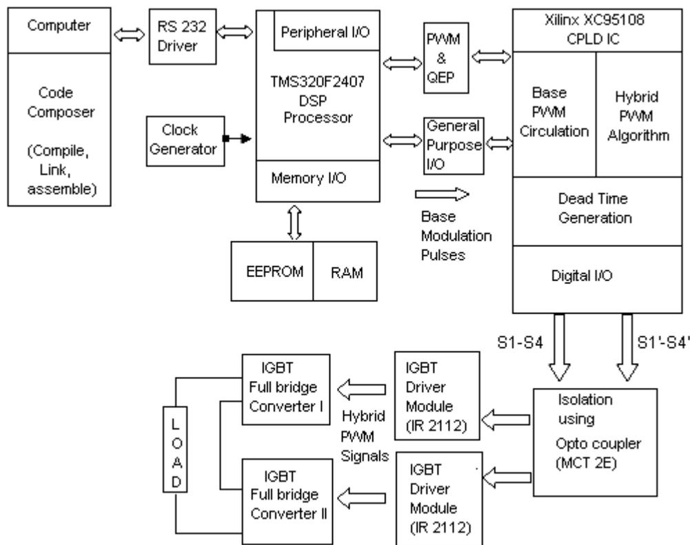
**Figure 3.15 Experimental setup for SSHSM controller implementation for five-level inverter**
