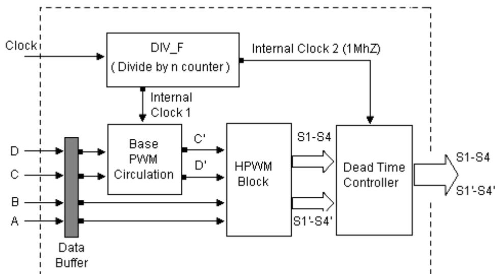
**Figure 3.16 Functional block diagram of control algorithm realization in CPLD**
