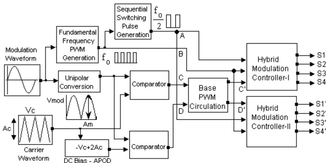
**Figure 3.4 Scheme of five-level sequential switching HAPOD modulation**
