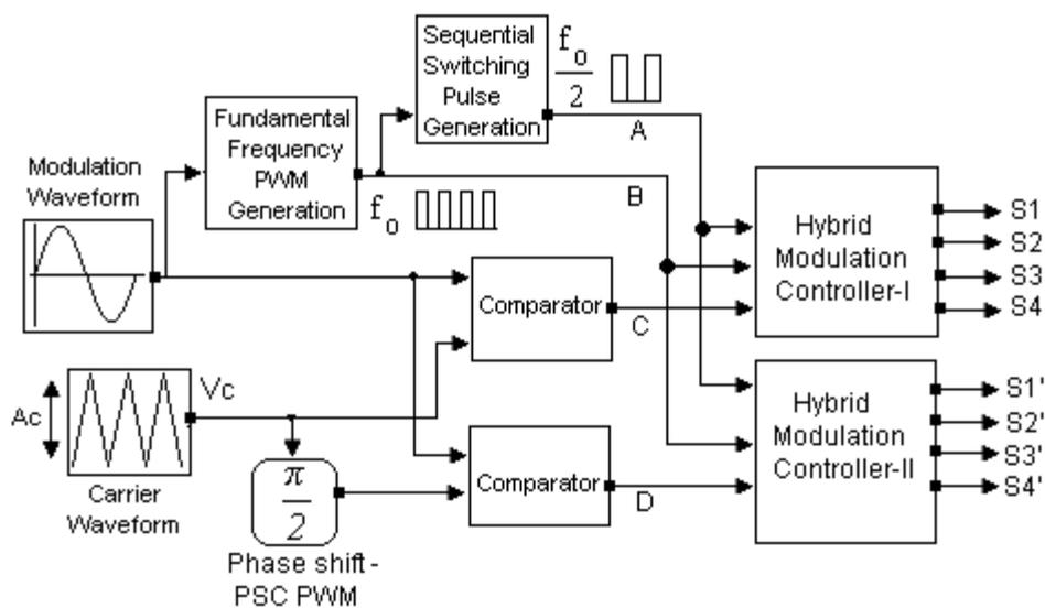
**Figure 3.13** Scheme of hybrid phase shifted carrier modulation
