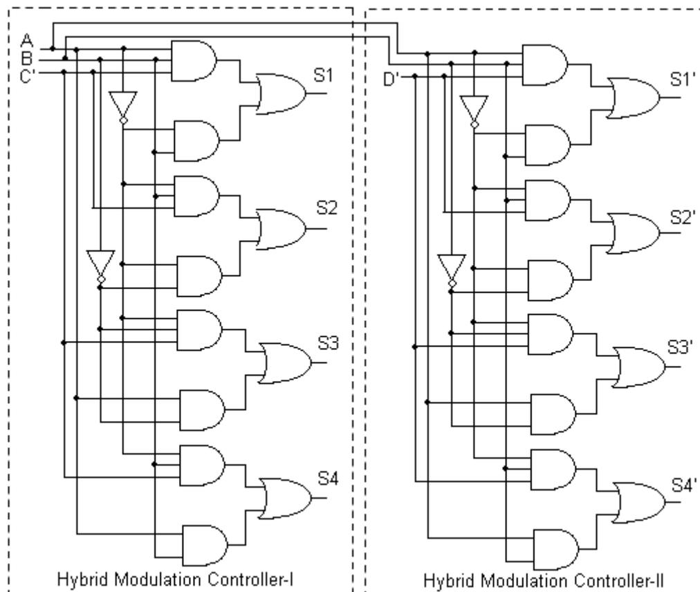
**Figure 3.3 Functional logic diagram of five-level hybrid modulation controller**
