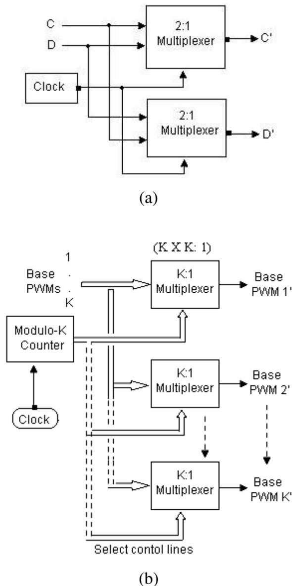
**Figure 3.2** Scheme of base MSPWM circulation: (a) five-level (b) N-level inverter
