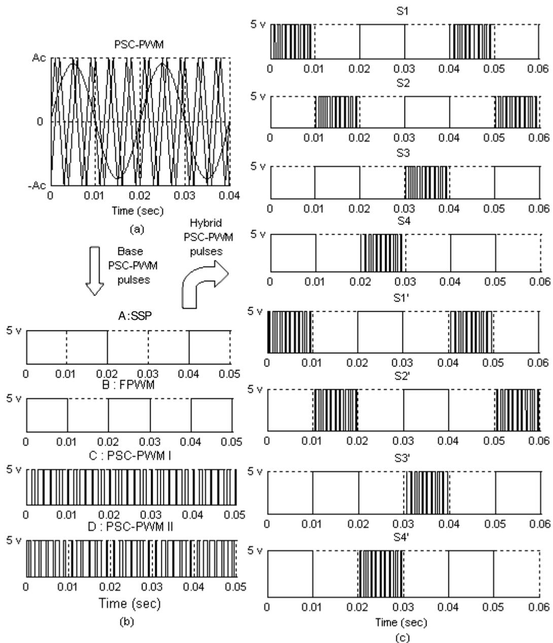
**Figure 3.14 (a) Phase shifted carrier and modulation waveforms
