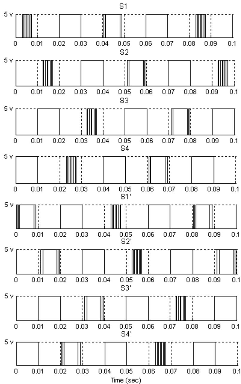
**Figure 3.9 Five-level sequential switching HSCSM pulse pattern**
