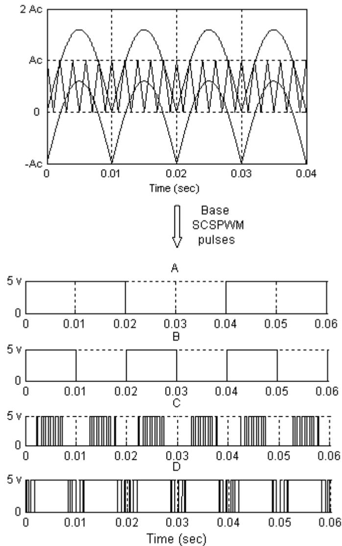
**Figure 3.8 Five-level base SCSM pulse pattern**
