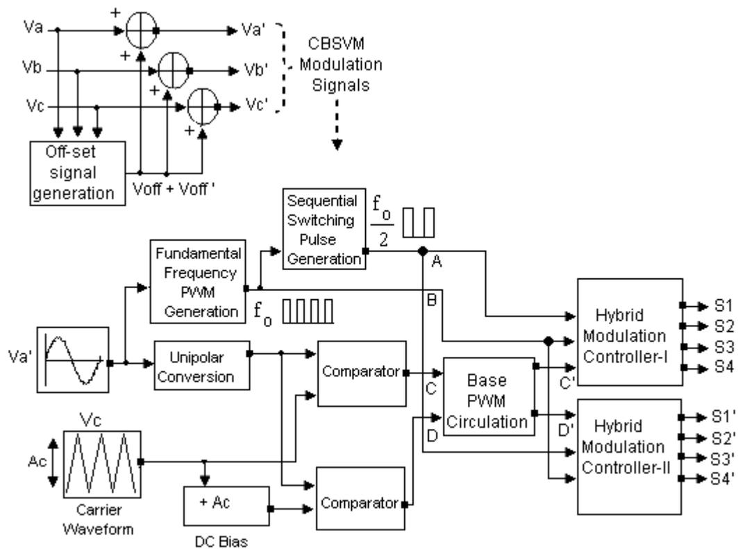
**Figure 3.10 Scheme of hybrid carrier based space vector modulation**
