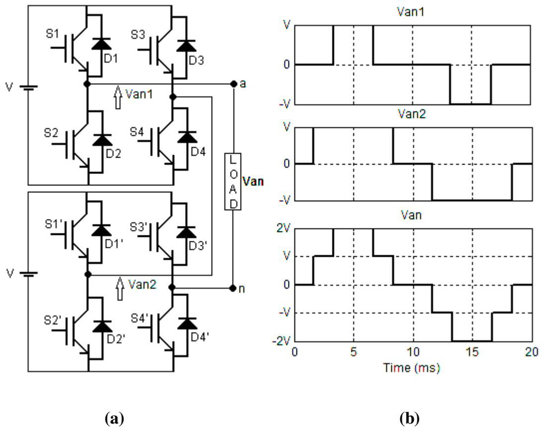
**Figure 1.2 (a) Schematic diagram of the five-level cascaded multilevel inverter (b) Output voltage waveform**
