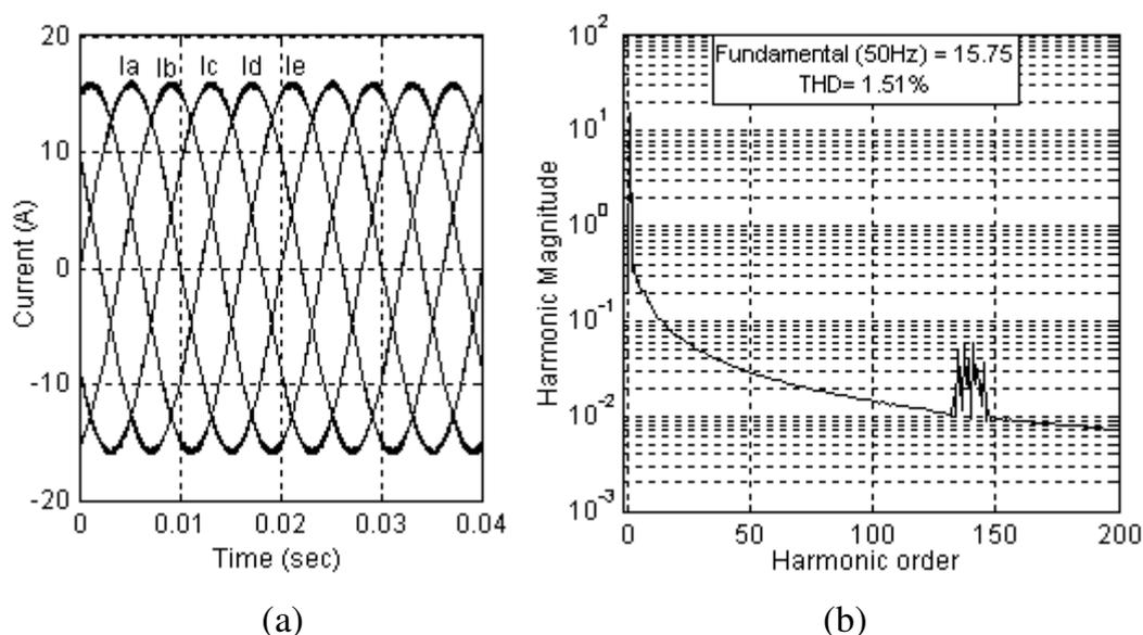
**Figure 6.13 Five phase sequential switching HPSC operation: (a) Five phase current waveforms (b) Spectrum of the phase current**
