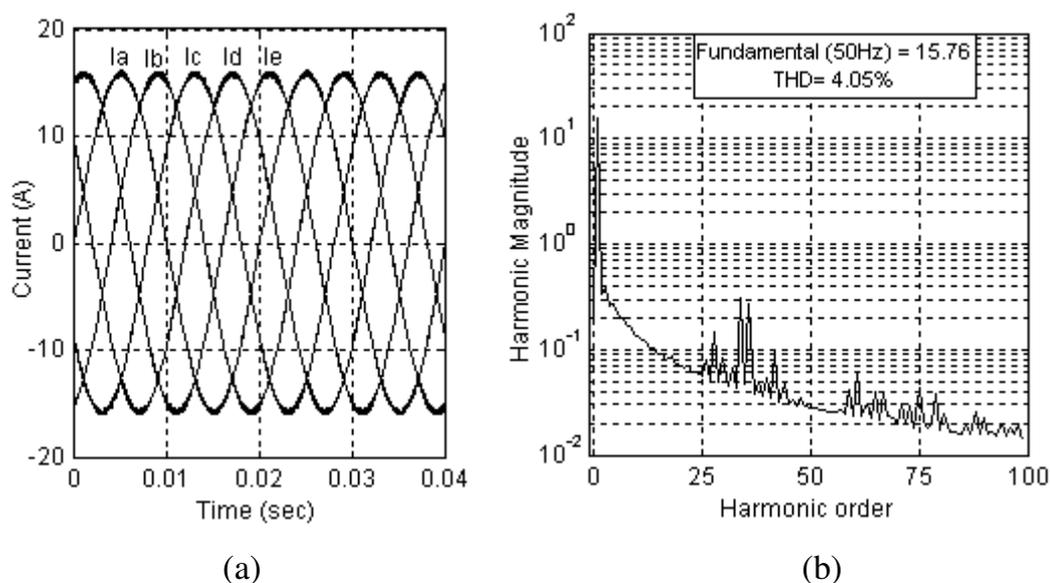
**Figure 6.7 Five phase sequential switching HSCSM operation (a) Five phase current waveforms (b) Spectrum of the phase current.**
