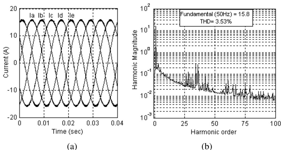
**Figure 6.4 Five phase sequential switching HAPOD operation: (a) Five phase current waveforms (b) Spectrum of the phase current**
