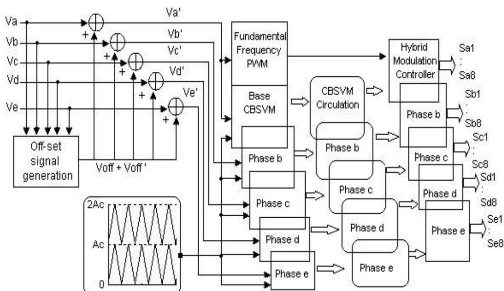
**Figure 6.8 Scheme of five-phase sequential switching HCBSVM**
