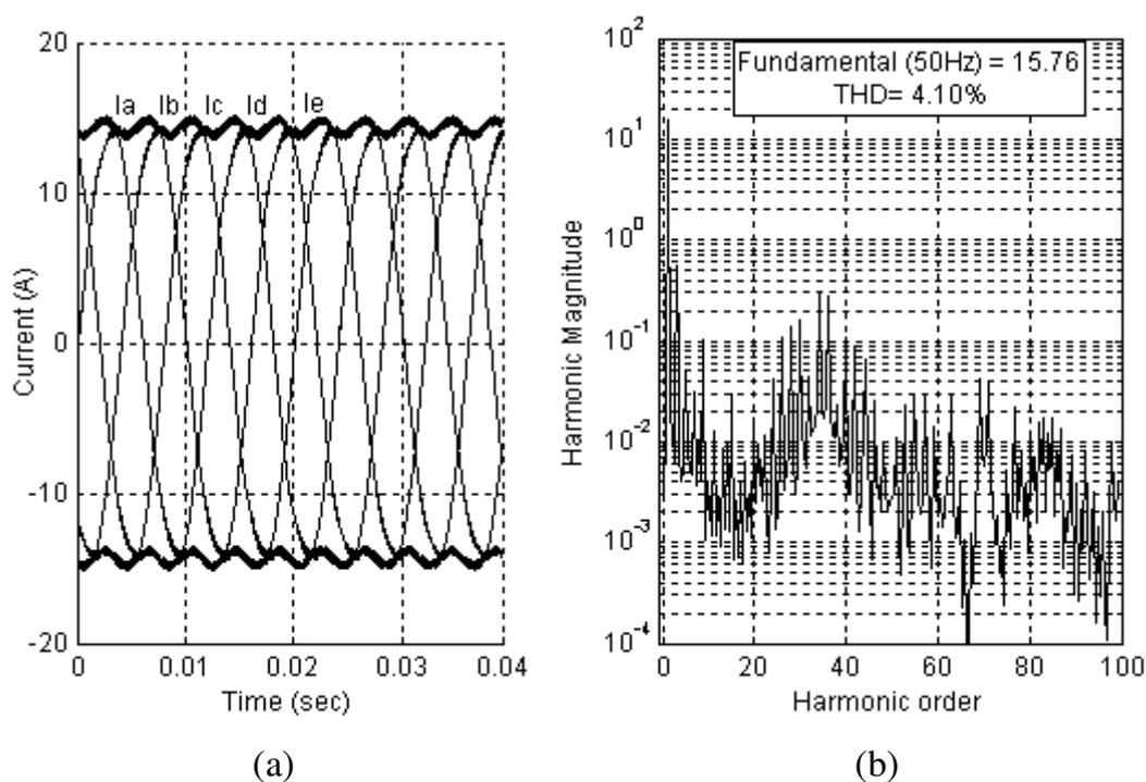
**Figure 6.10 Five phase sequential switching HCBSVM operation:**
