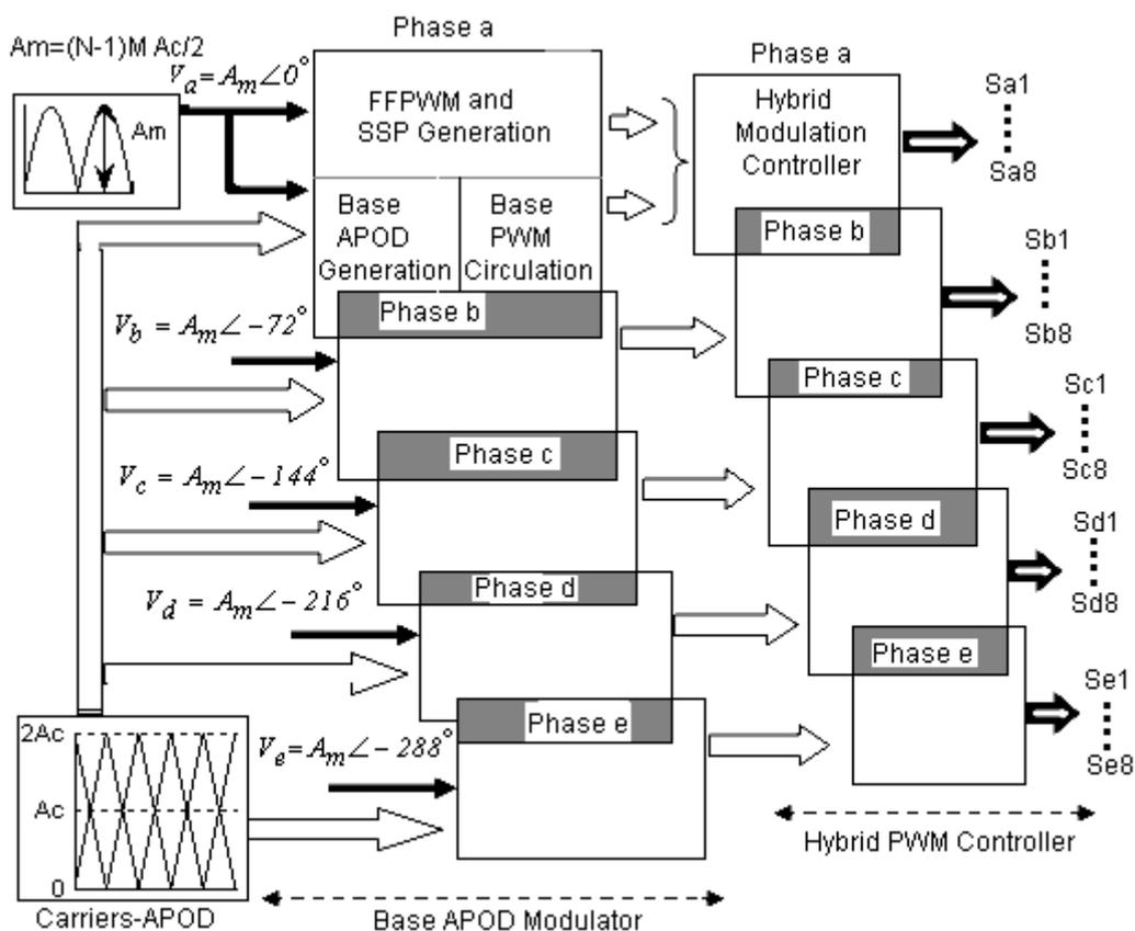
**Figure 6.2 Scheme of five-phase sequential switching HAPOD modulation**
