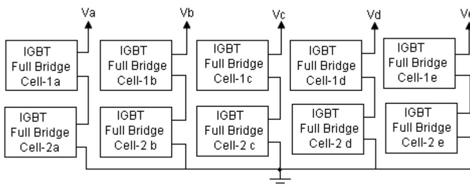
**Figure 6.1 Schematic diagram of the five-phase five-level inverter**
