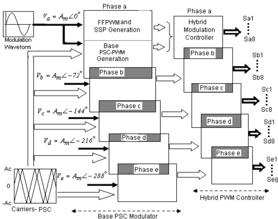
**Figure 6.11 Scheme of five-phase sequential switching HPSC modulation**
