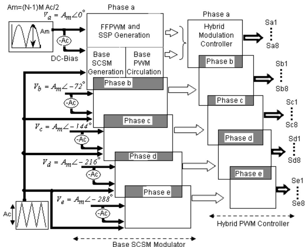
**Figure 6.5 Scheme of five-phase sequential switching HSCSM**
