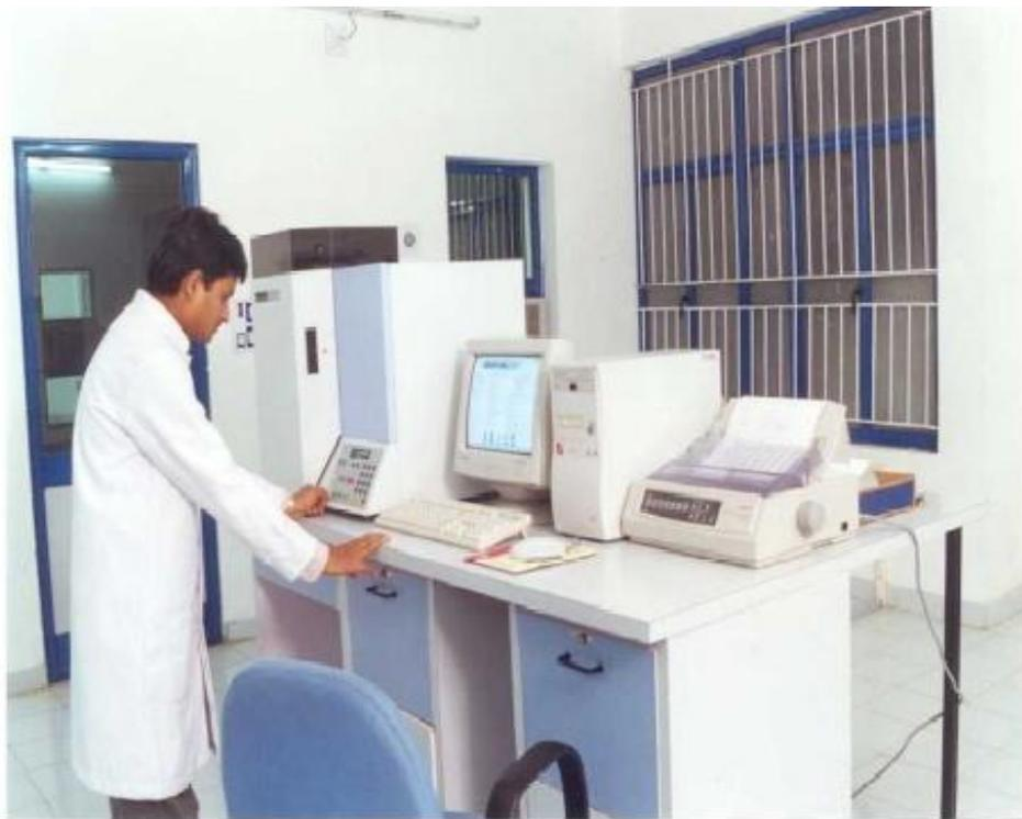
**Figure 6.1: C-H-N-S-O Analyzer at SICART, V.V.Nagar, Gujarat**
