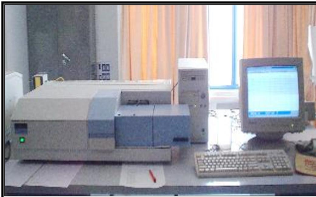
**Figure 4.5 UV-VIS-NIR Spectrophotometer**
