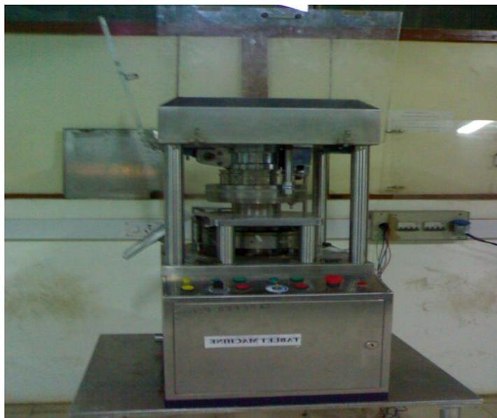
**Figure 3.7: Rotary Tablate Machine**
