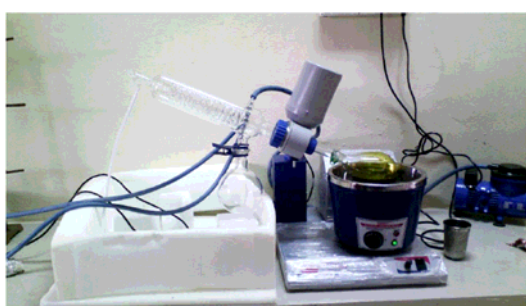
Photograph showing rotary vacuum evaporator (Model: Superfit, PBU -6) used for the condensation of the crude extracts.
