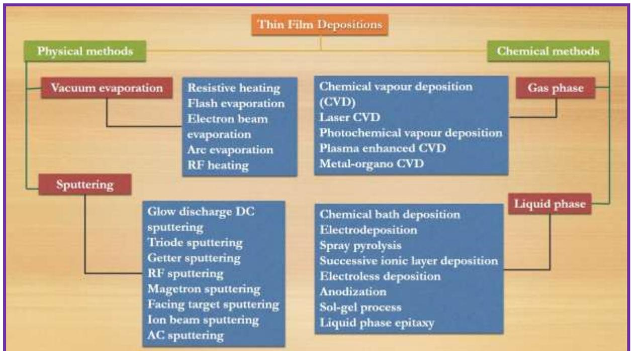
**Figure 1.1.** Classification of thin film deposition techniques.
