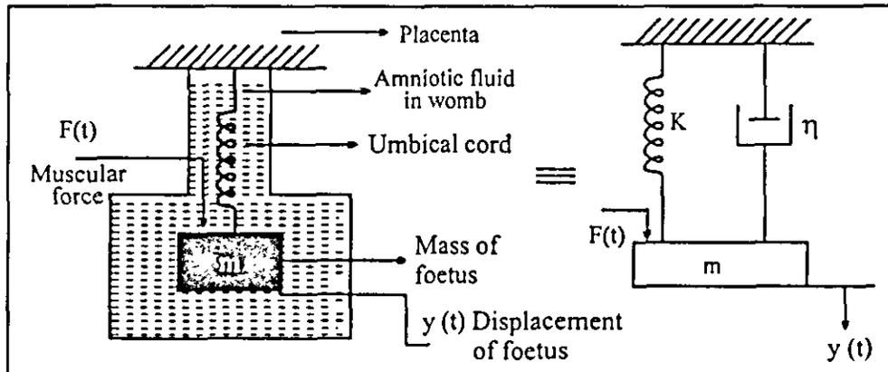
Fig. 4.9 : Equivalent mechanical spring-mass dashpot system of womb (at any stage of pregnancy)
