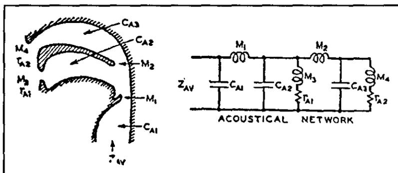
Fig. 4.4 : Schematic sectional view and the acoustical network of the vocal cavities.
