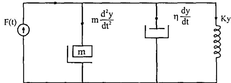
Fig. 4.10 : Mechanical circuit diagram of womb
