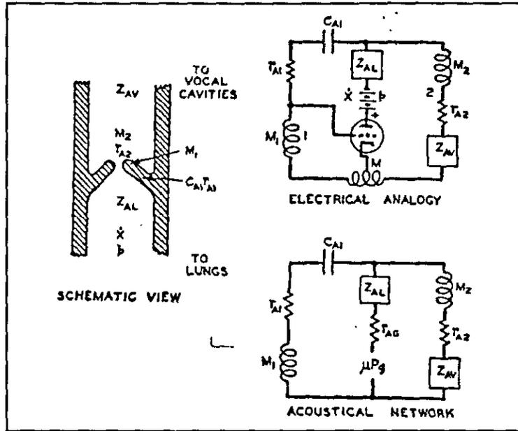
Fig. 4.3 : Sectional view of a vibrating system approximating the larynx.
