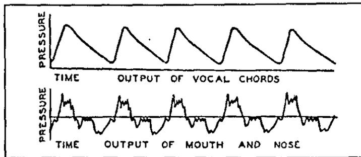
**Fig. 4.5 : Wave shapes of the output of the vocal cords and the mouth and nose for the vowel sound.**
