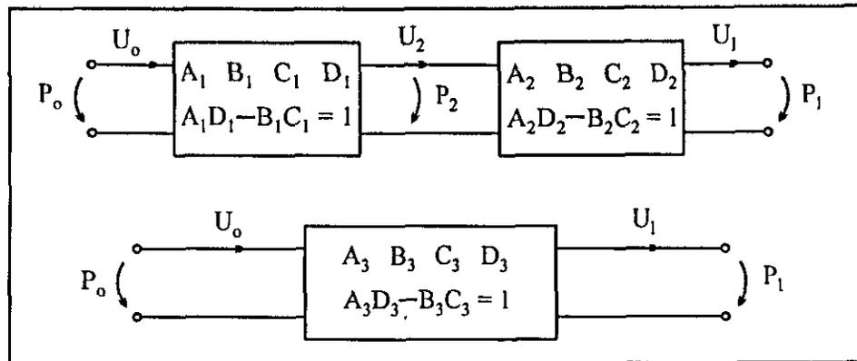
Fig. 4.8 : Twin tube resonator seen as a single resultant network
