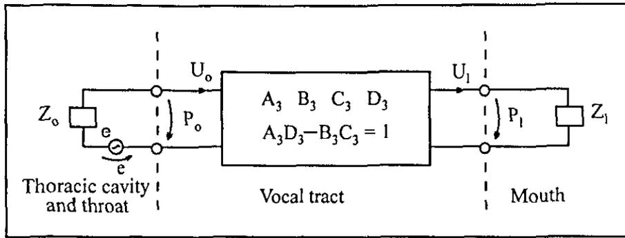
Fig. 4.12 : The throat considered as a source of sinusoidal vibrations
