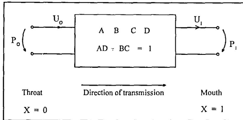
**Fig. 4.7 : Equivalent electric four terminal network of the vocal tract**
