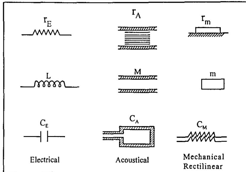
**Fig. 4.2 : Graphical representation of the three basic elements in Electrical, Mechanical rectilinear and Acoustical system**
