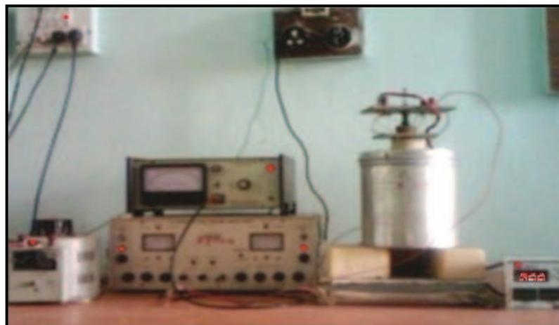
**Fig.3.10** Experimental setup for d.c. electrical resistivity
