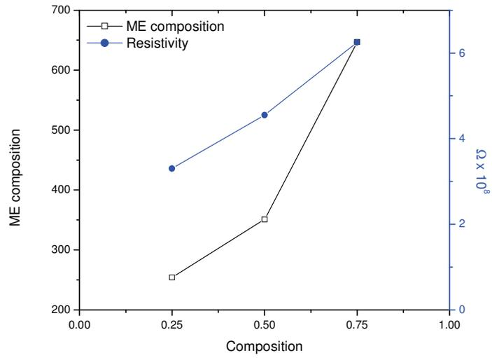
Fig 5.11 Variation of resistivity and Magneto electric effect with composition for  $(1-x) \text{Co}_{1.2}\text{Mn}_{0.2}\text{Fe}_{1.6}\text{O}_4 + (x) \text{BaTiO}_3$ .
