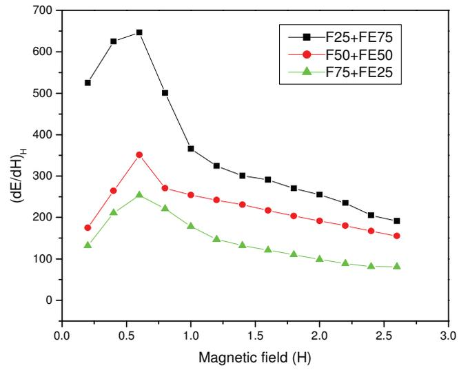
Fig 5.10 Variation of magneto-electric conversion factor with magnetic field for  $(1-x) \text{Co}_{1.2}\text{Mn}_{0.2}\text{Fe}_{1.6}\text{O}_4 + (x) \text{BaTiO}_3$ .
