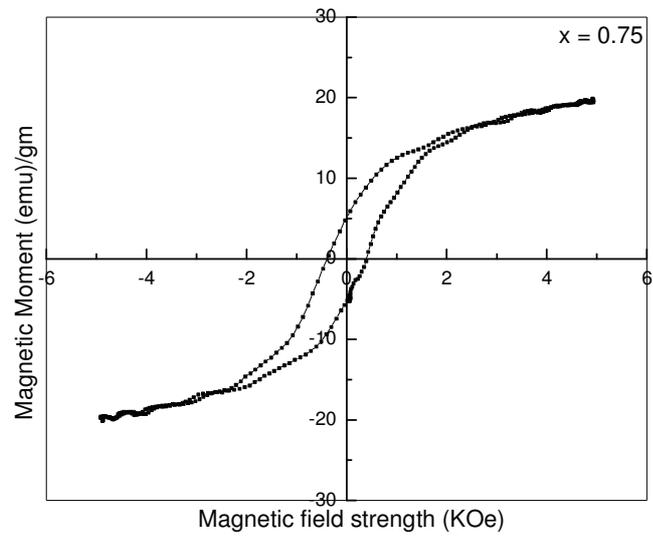
Fig. 5.4 Hysteresis loop for  $(1-x) \text{Co}_{1.2}\text{Mn}_{0.2}\text{Fe}_{1.6}\text{O}_4 + (x) \text{BaTiO}_3$  ( $x = 0.75$ ) Composite.
