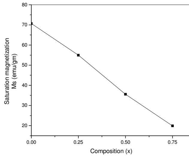
Fig 5.5 Variation of saturation magnetization with composition for  $(1-x) \text{Co}_{1.2}\text{Mn}_{0.2}\text{Fe}_{1.6}\text{O}_4 + (x) \text{BaTiO}_3$ .
