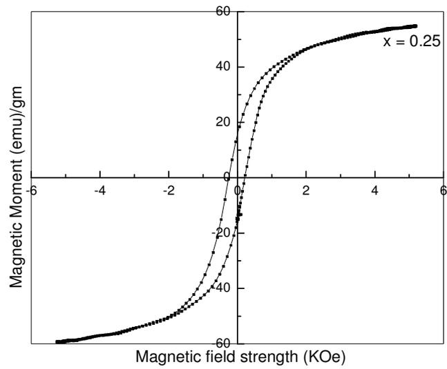
Fig. 5.2 Hysteresis loop for  $(1-x) \text{Co}_{1.2}\text{Mn}_{0.2}\text{Fe}_{1.6}\text{O}_4 + (x) \text{BaTiO}_3$ . ( $x = 0.25$ )
