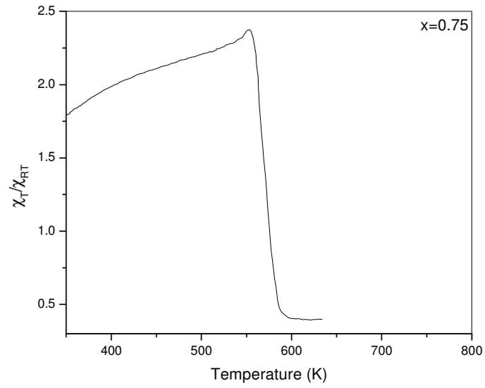
Fig 5.9 Variation of  $\chi_T/\chi_{RT}$  versus temperature of system  $(1-x) \text{Co}_{1.2}\text{Mn}_{0.2}\text{Fe}_{1.6}\text{O}_4 + (x) \text{BaTiO}_3$  ( $x = 0.75$ ) composite.
