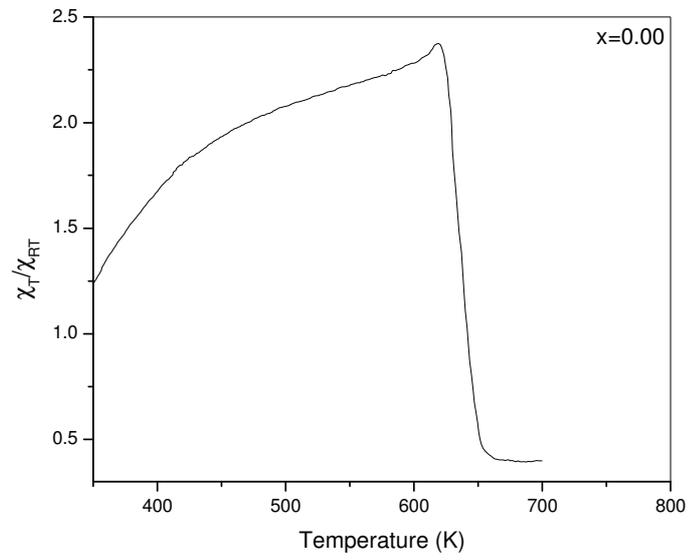
Fig 5.6 Variation of  $\chi_T/\chi_{RT}$  versus temperature of system  $(1-x)\text{Co}_{1.2}\text{Mn}_{0.2}\text{Fe}_{1.6}\text{O}_4 + (x)\text{BaTiO}_3$ . ( $x = 0.0$ ) composite.
