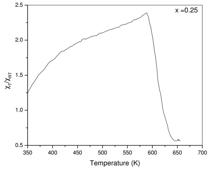
Fig 5.7 Variation of  $\chi_T/\chi_{RT}$  versus temperature of system  $(1-x) \text{Co}_{1.2}\text{Mn}_{0.2}\text{Fe}_{1.6}\text{O}_4 + (x) \text{BaTiO}_3$ . ( $x = 0.25$ ) composite.
