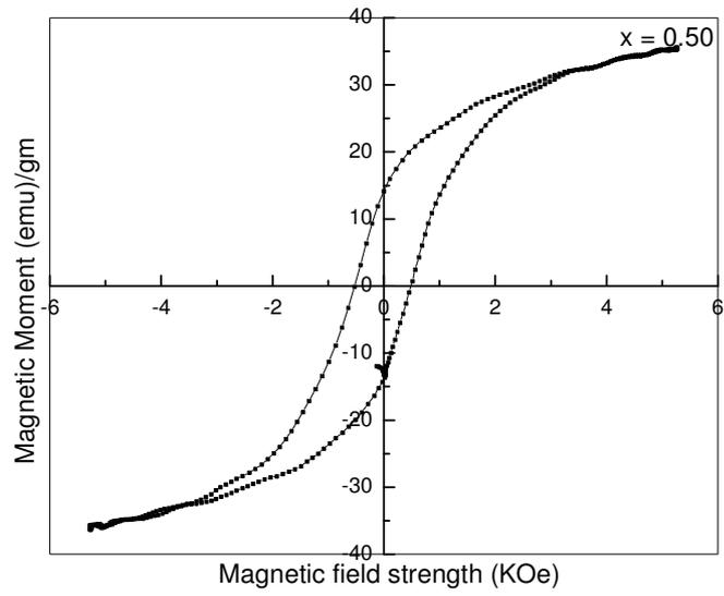
Fig. 5.3 Hysteresis loop for  $(1-x) \text{Co}_{1.2}\text{Mn}_{0.2}\text{Fe}_{1.6}\text{O}_4 + (x) \text{BaTiO}_3$ . ( $x = 0.50$ )
