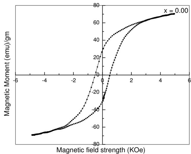
Fig. 5.1 Hysteresis loop for  $(1-x) \text{Co}_{1.2}\text{Mn}_{0.2}\text{Fe}_{1.6}\text{O}_4 + (x) \text{BaTiO}_3$ . ( $x = 0.00$ )
