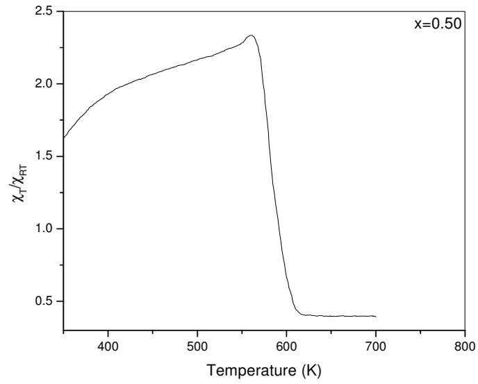
Fig 5.8 Variation of  $\chi_T/\chi_{RT}$  versus temperature of system  $(1-x) \text{Co}_{1.2}\text{Mn}_{0.2}\text{Fe}_{1.6}\text{O}_4 + (x) \text{BaTiO}_3$ . ( $x = 0.50$ ) composite.
