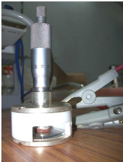
**Figure 4.13** A sample holder for dielectric measurement
