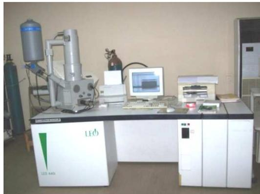
**Figure 4.11** Photograph of LEO 440i instrument used for SEM
