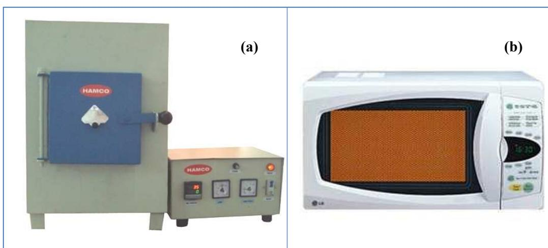
**Figure 4.5** Sintering equipments (a) Muffle furnace and (b) Microwave oven
