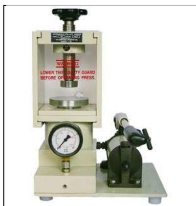
**Figure 4.9** Photograph of Hydraulic Press used to make pellets
