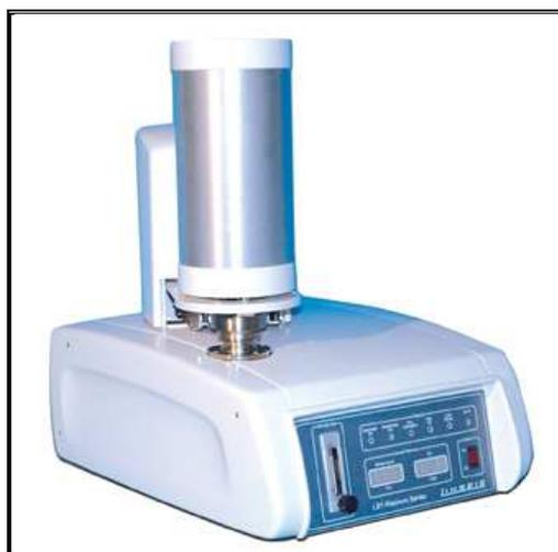
**Figure 4.8** Photograph of Linseis STA PT1600 used for TG-DTA
