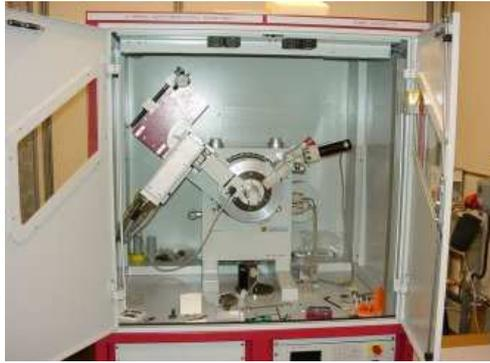
**Figure 4.10** Photograph of XRD unit used for characterizations
