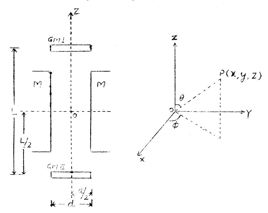
The various lengths have been explained in the figure itself. The problem is the following: Suppose a particle impinges on the upper GM-counter anywhere between -d/2 to +d/2. What is the probability that after passing through the magnetic field whose strength is  $\phi$  H.dl, it is recorded by the lower counter
