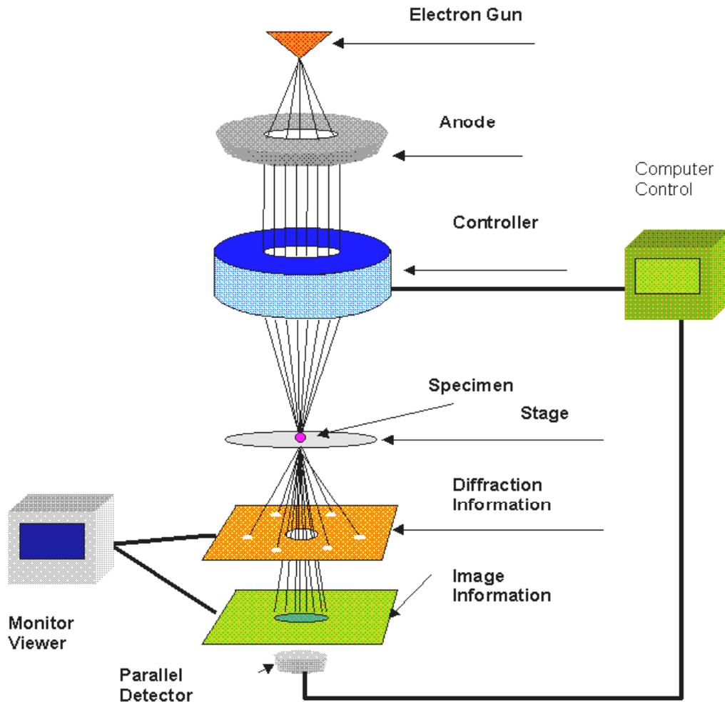
Figure 4.3: Block diagram of Transmission Electron Microscope (TEM)
