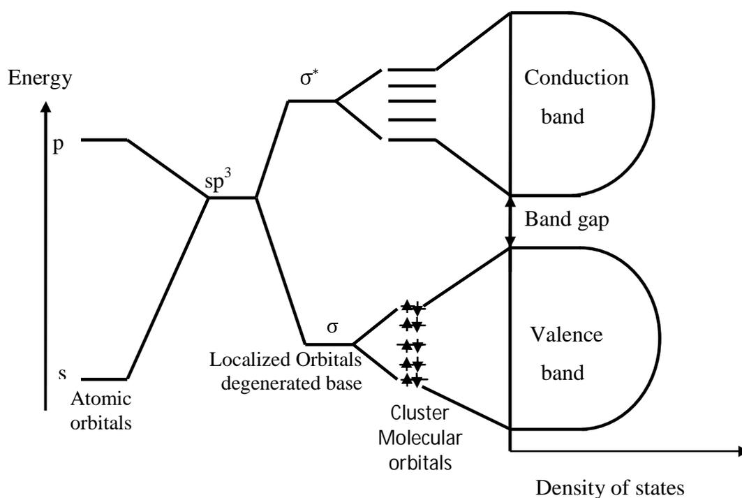
Figure 4.8: Evolution from molecular orbitals into bands
