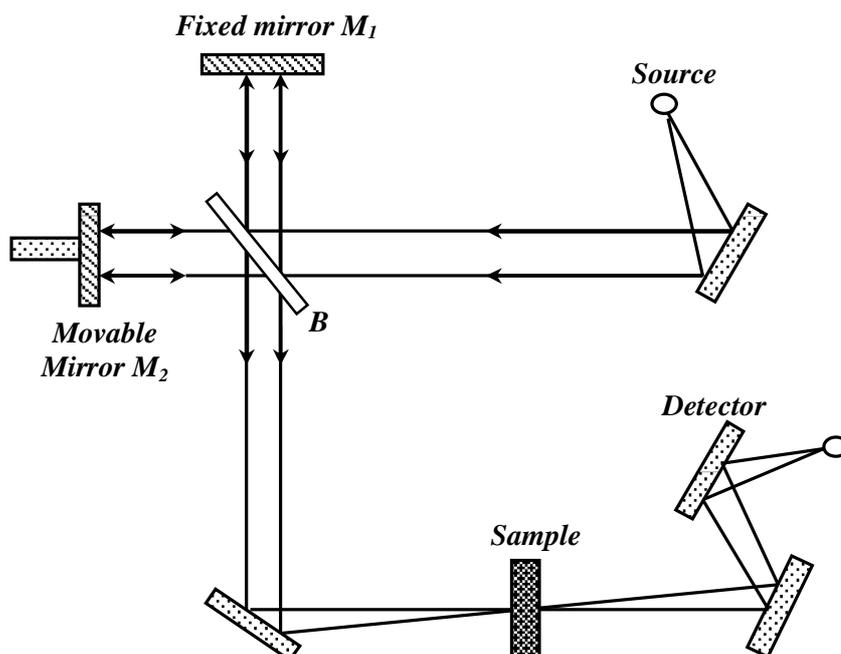
Figure 4.10: Schematic diagram of Fourier transform infrared (FTIR) spectrometer
