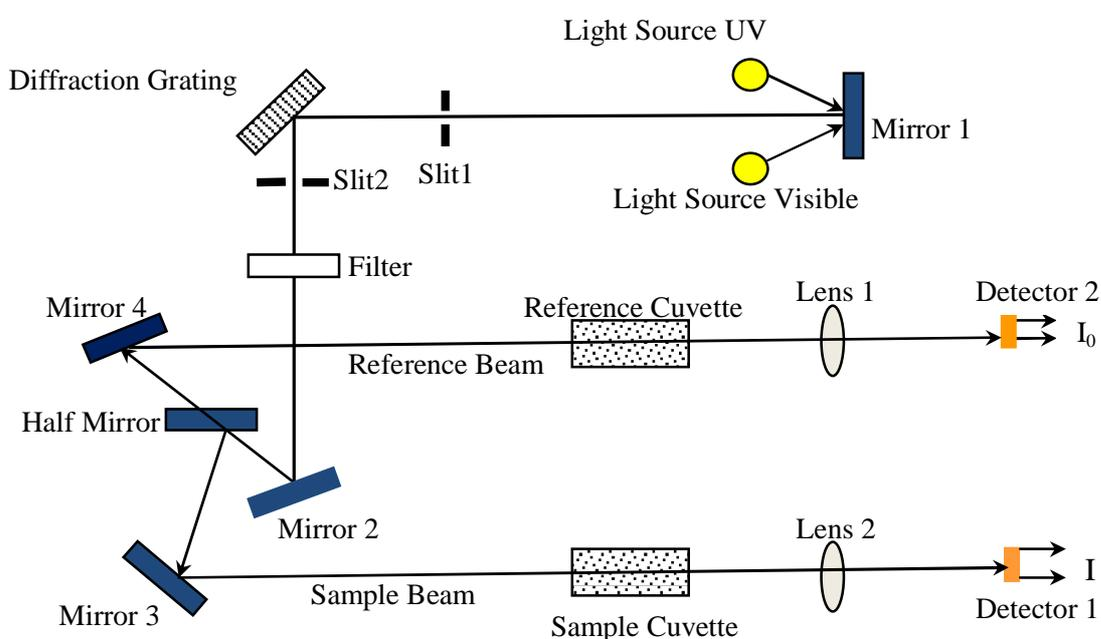
Figure 4.7: Schematic diagram of UV-visible spectrophotometer (double beam)
