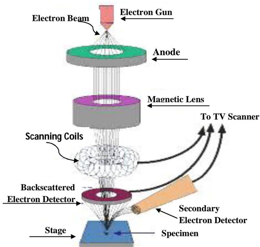
Figure 4.5: Schematic Diagram of Scanning Electron Microscope (SEM)
