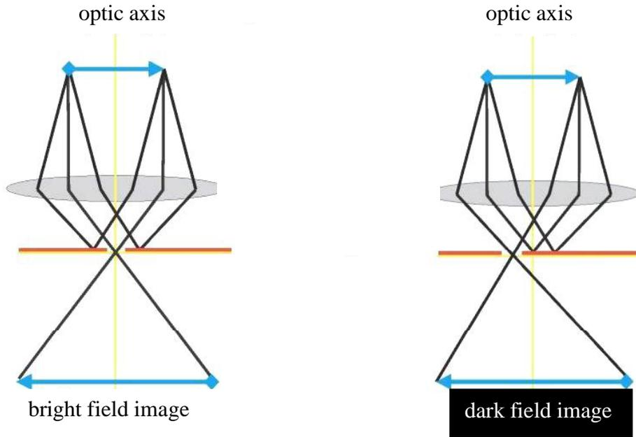
Figure 4.4: Bright field imaging and dark field imaging
