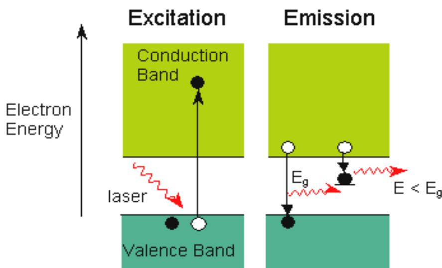
Figure 4.9: Mechanism of photoluminescence
