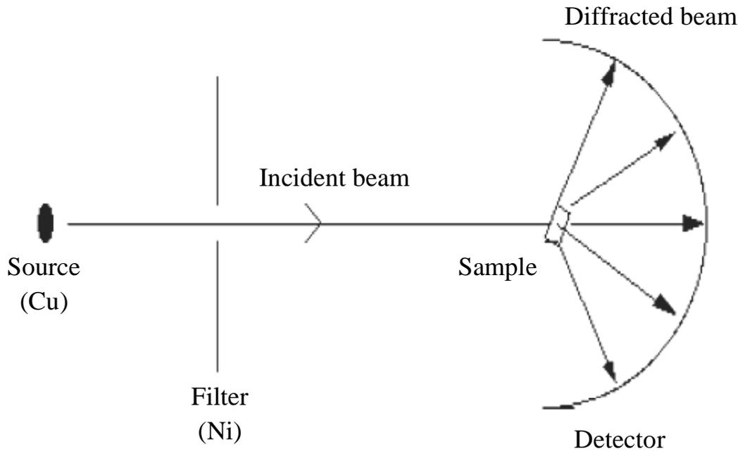
Figure 4.1: Schematic diagram of X-ray powder diffraction
