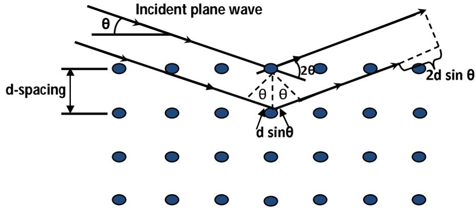
Figure 4.2: Schematic diagram for deriving Bragg's law
