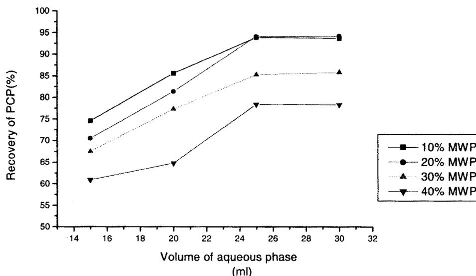
**Figure 4.12** The influence of variation of aqueous phase volume on the recovery of spiked PCP using n-octane 1 ml and duration of 3 min
