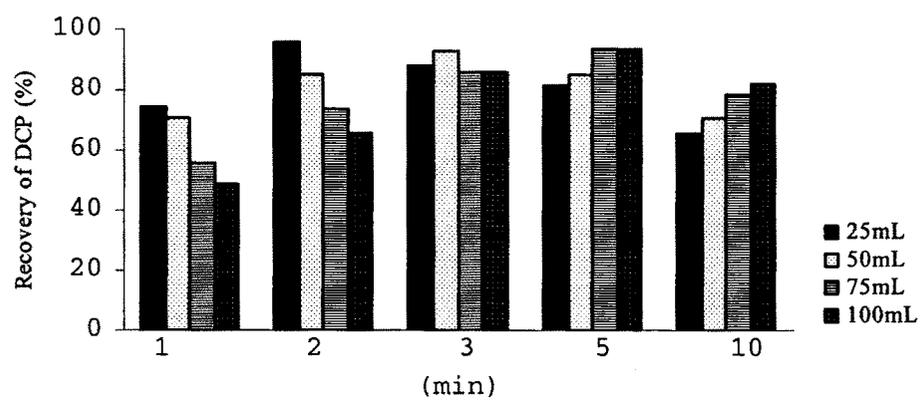
**Figure 4.5** Dependency of recovery of DCP on sample volume in water sample in correlation to MW heating duration (MWP 10%)
