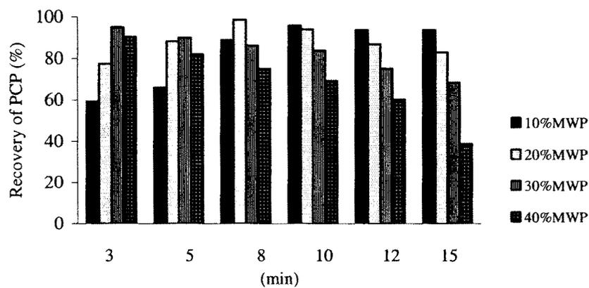
**Figure 4.4** Dependency of recovery of PCP from leather on MW heating duration
