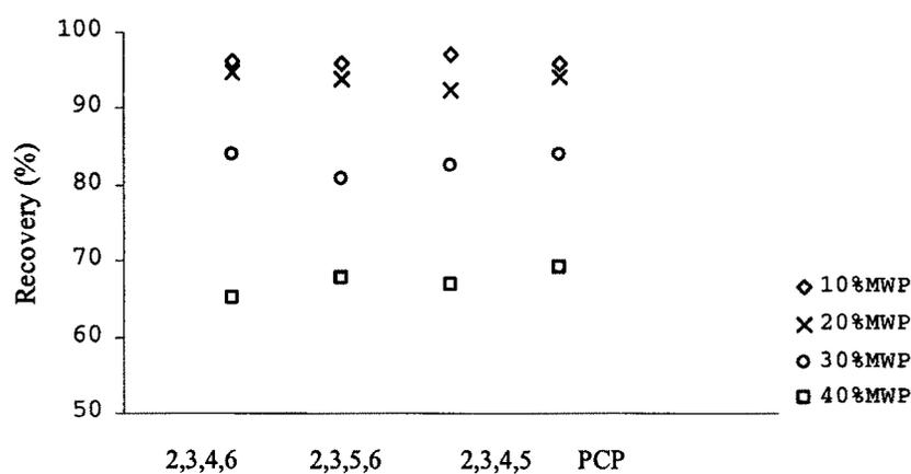
**Figure 4.11 Recovery data of TeCPs and PCP from leather on varying MW heating**
