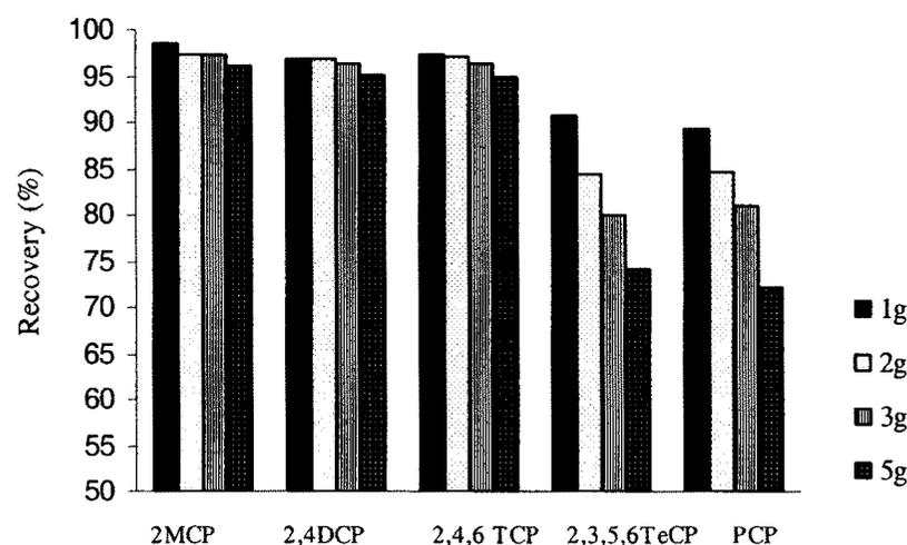
**Figure 4.14 Influence of weight of soil sample on Microwave extraction. Conditions:- 10-40% MWP was varied for a fixed duration of 8min (as that is suitable for volatiles) 25 ml of aqueous phase was used with 1 ml n-octane as trap.**
