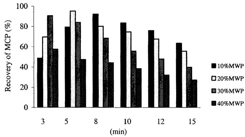
**Figure 4.1** Dependency of recovery of 2-MCP from soil sample on MW heating duration
