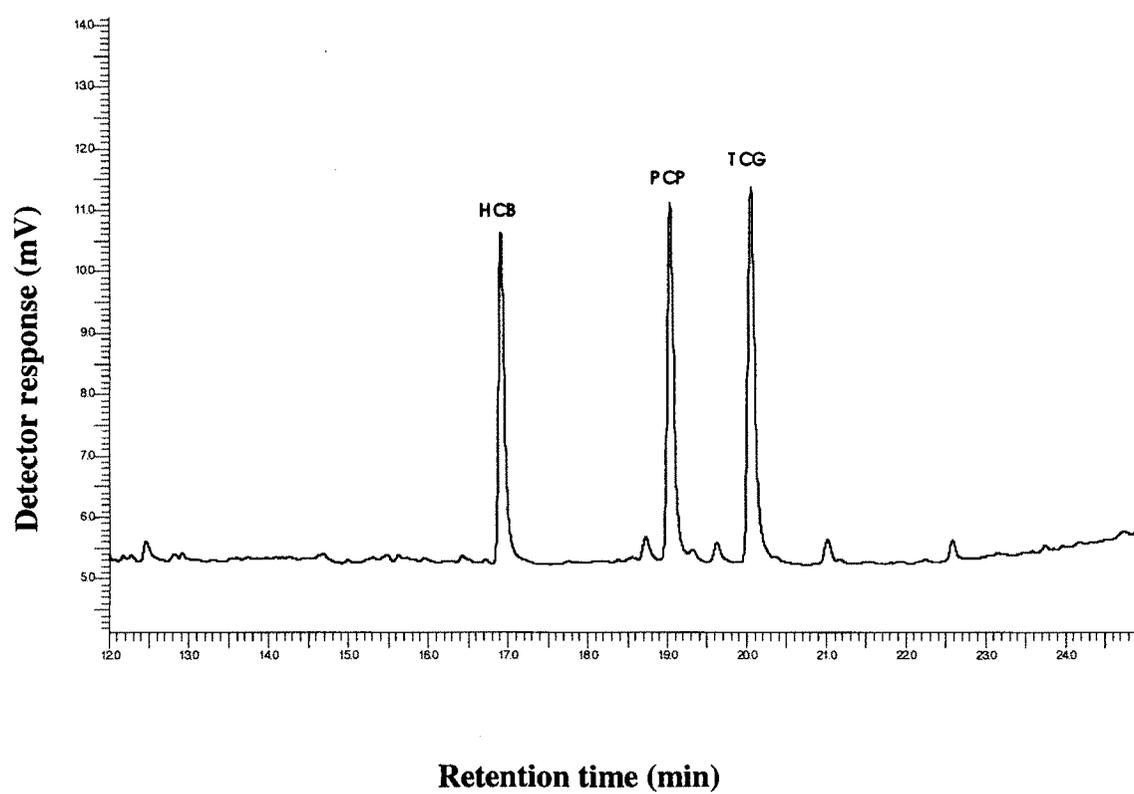
**Figure 4.16** GC chromatogram of a textile sample extracted by in situ derivatisation method using 1 ml of n-octane. PCP originally present in the sample is detected. TCG shown is an internal standard added while HCB is added as an injection marker
