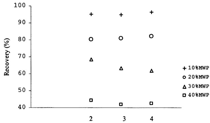
**Figure 4.7 Recovery data of MCPs from soil on varying MW heating**
