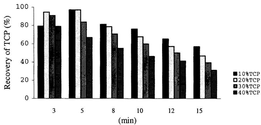
**Figure 4.3** Dependency of recovery of 2,4,6-TCP in Textile on MW heating duration
