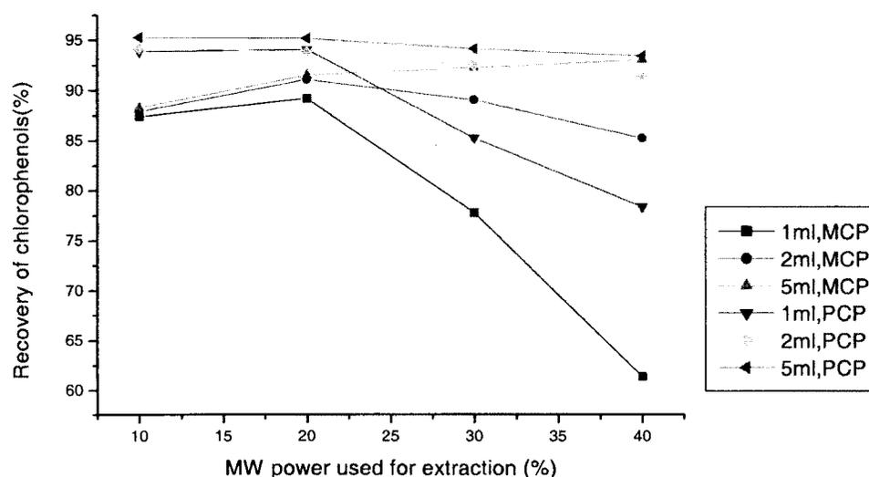
**Figure 4.13 Influence of variation of solvent used for trapping in correlation to the variation of MWP from 10-40%. The other conditions: 25 ml aqueous phase and duration of extraction is 3 min**
