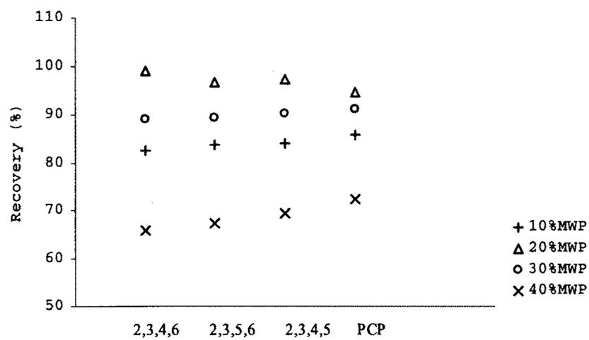
**Figure 4.10 Recovery data of TeCPS and PCP from soil on varying MW heating**
