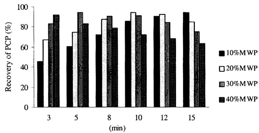
**Figure 4.2** Dependency of PCP recovery from soil sample on MW heating duration
