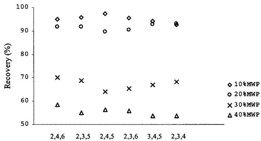
**Figure 4.9 Recovery data of TCPs from soil on varying MW heating**
