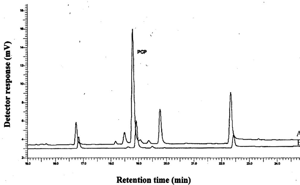
**Figure 4.15** Overlay of chromatograms of PCP extracted (as derivative) from a leather sample (native) A. extracted using 1 ml n-octane; B. extracted using 5 ml n-octane
