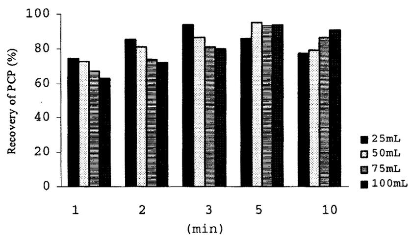
**Figure 4.6** Dependency of recovery of PCP on sample volume in water sample in correlation to MW heating duration (MWP 10%)
