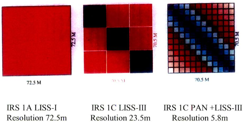
**Figure 1.2 Graphical representation of the concept of multisensor image fusion**
