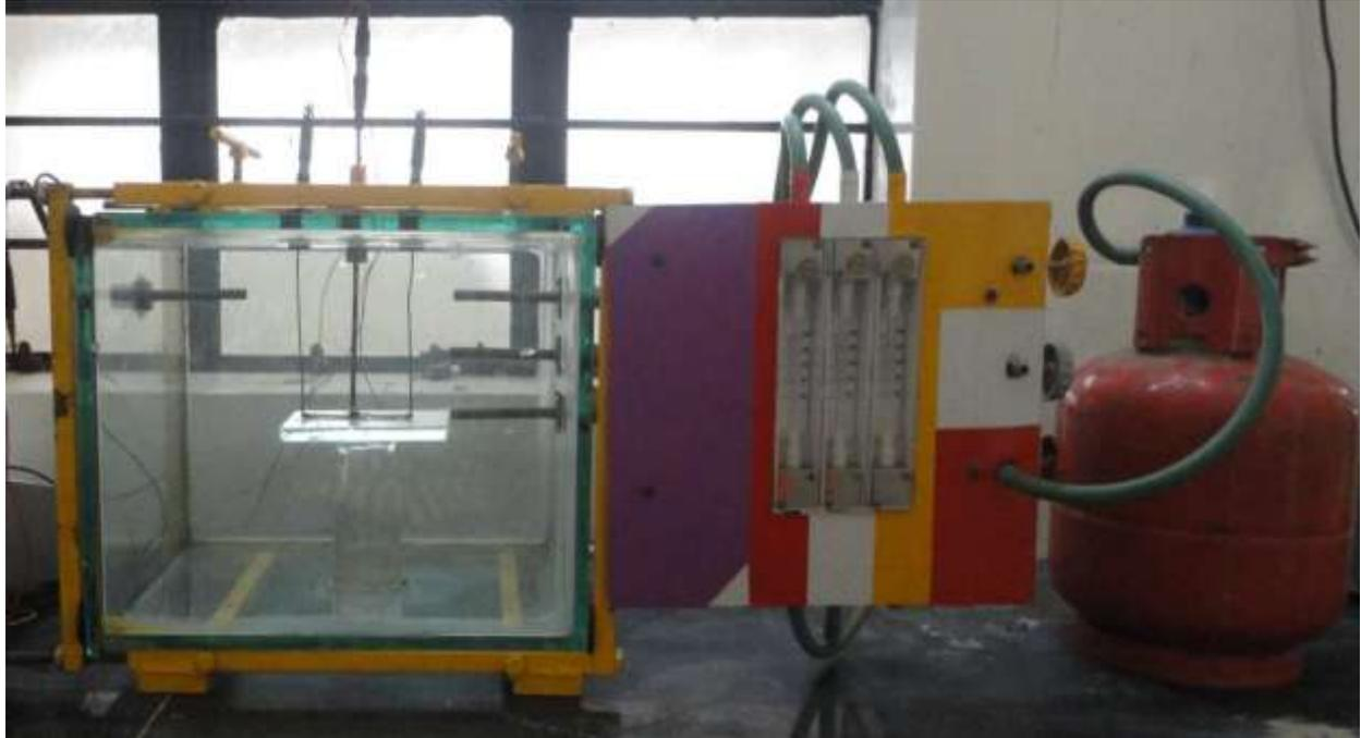
**Figure 5.2(b): Photograph of gas sensor set-up**
